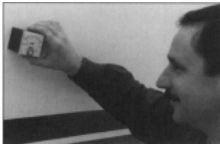
Duarte Picanco of Toronto-based Noahs checks moisture levels of the hull laminate prior to painting.
