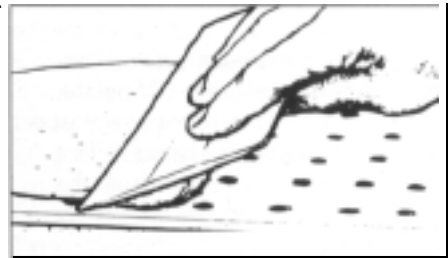
Step 6: Sand the surface then fill low spots with thickened epoxy.
