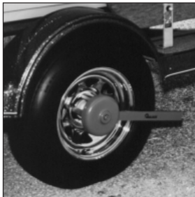
Trailock attaches to the lug nuts and prevents the wheel from turning.
