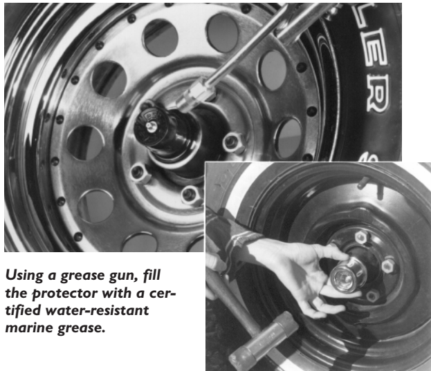
Bearing protectors fit tightly over the hub and are tapped into place with a rubber mallet.
