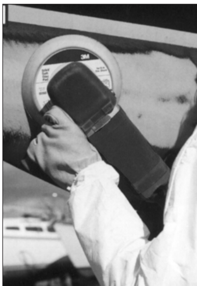
Use a grinder with a foam disc pad to remove bottom paint.
