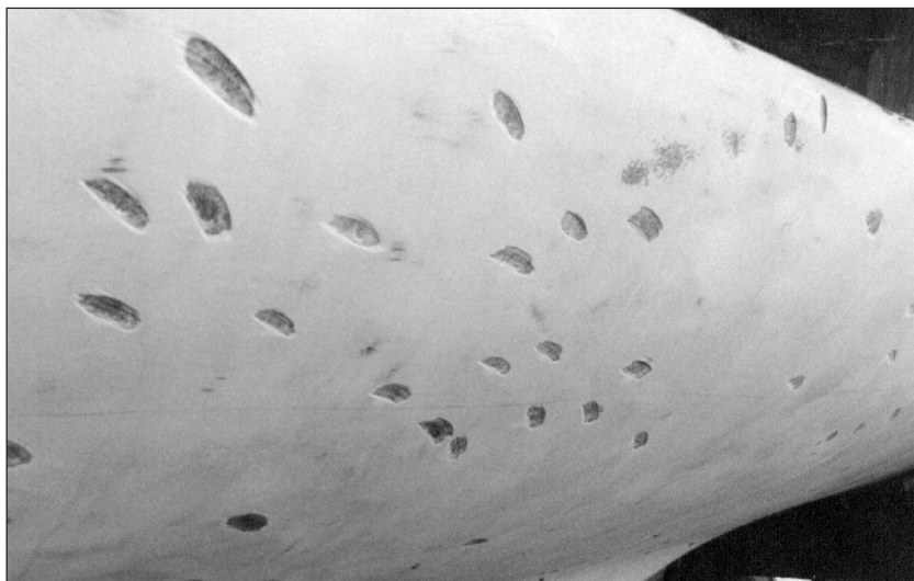
Damage can range from a few small blisters to an entire hull dotted with the "pox."
