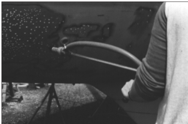
Sandblasting removes gelcoat and opens blister cavities but must be done by a competent operator.
