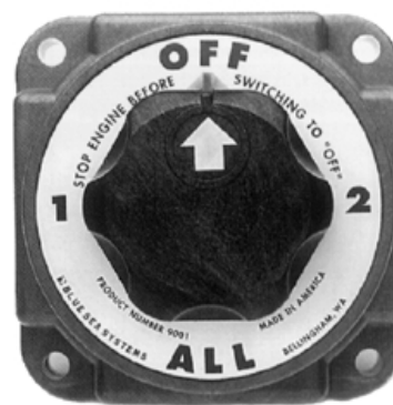
Figure 1: A four-position master switch lets you isolate the batteries, select which battery requires charging or completely cut off all power.
