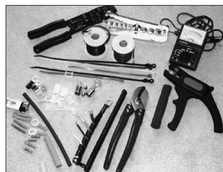
Figure 6: A typical DC electrical tool kit for DIY installations: crimp tool, lug crimper, multimeter, wire stripper, coaxial cable stripper, AWG wire, cable ties and clamps, fuses, assorted crimp and heat-shrink terminals, butane lighter or heat gun, heat-shrink tubing, spiral wrap, wire/cable cutter and wire markers (missing).
