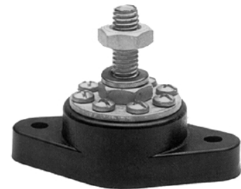
Figure 5: A negative consolidation terminal such as the PowerPost+, provides an attachment point for multiple negative cables, allowing a single cable to connect to the engine ground.
