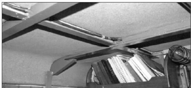
The pilothouse deckhead of Playfair , a 21.6m (72') brigantine based in Toronto, Ont., was covered in cork three years ago and still looks as good as new.
