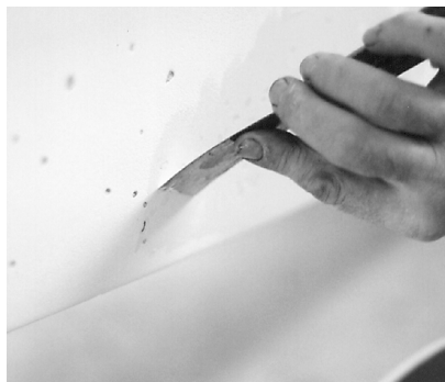
Fill pinholes with fairing compound and a putty knife held at a low angle.
