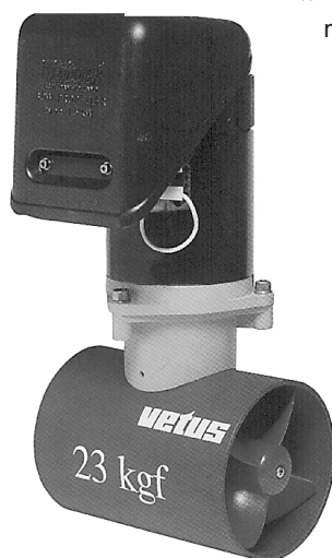
The Vetus 23kgf fits in a 12.7cm (5") tunnel — ideal for boats in the under-9m (30') range.
