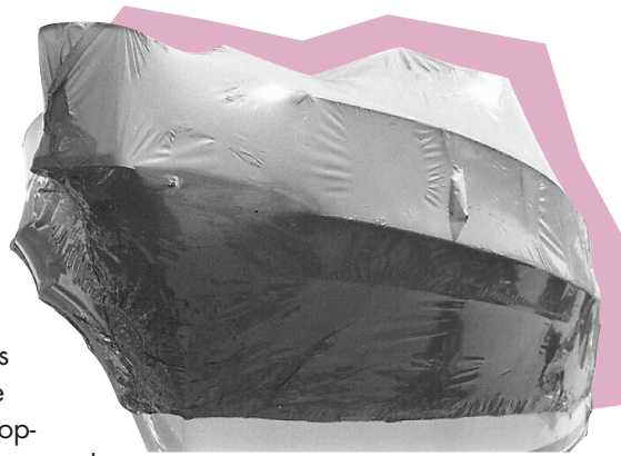
Shrinkwrap fits like a glove but traps moisture. Vents help to reduce condensation and mildew buildup.
