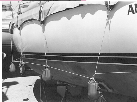
Plastic jugs filled with water or canvas bags stuffed with sand and tied around the hem of the cover maintain an even tension and prevent the cover from flapping in the wind.
