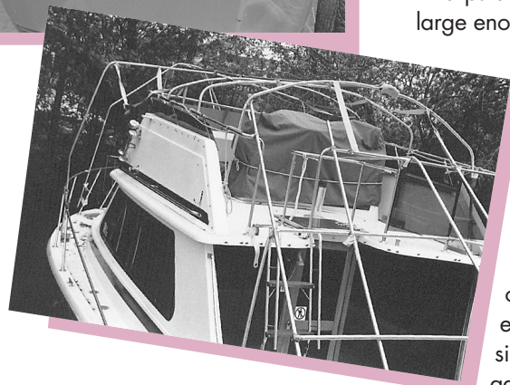
Frames made of PVC (top), or galvanized pipe (bottom) are inexpensive and easily assembled to fit a variety of cabin and deck shapes.
