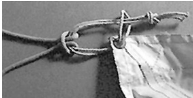
Make the toggle cord just long enough so it fits snug against the clew. It's shown larger than it needs to be for clarity.
