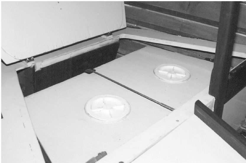
A removable wood-epoxy water tank fits snugly in the vee-berth and has two inspection ports for cleaning. A stainless-steel cable with adjustable turn-buckle attaches to the bulkhead and leads around the tank to a floor-mounted pad eye to hold the tank securely in place. A rubber gasket under the wire on the forward edge protects the tank from chafe.
