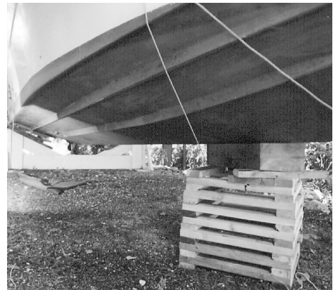
Bow view: Box frame is simple to build and fully portable.
