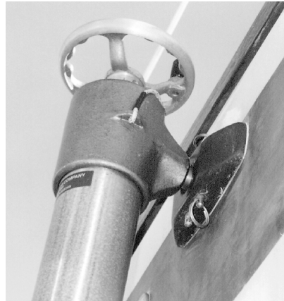
(Left) The "leg" sits snugly against the hull at a 7° angle on the Corbin 39. (Top) Closeup of the upper leg assembly shows the key and split ring locking mechanism and adjustable wheel for fine tuning.
