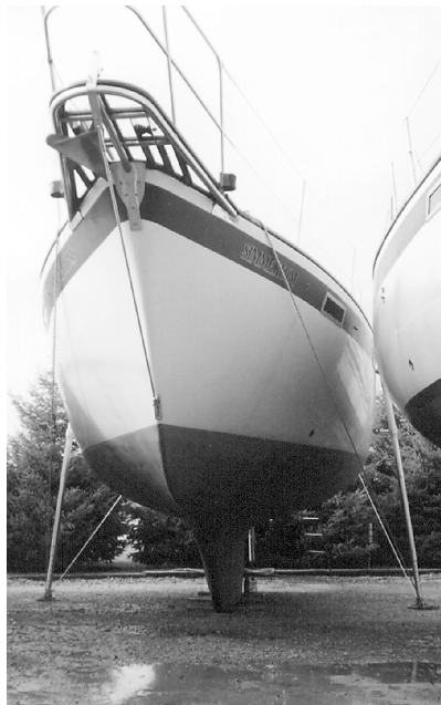
Portable "legs" keep the boat upright in mud, sand or on land, allowing clear access to the hull for cleaning or painting.
