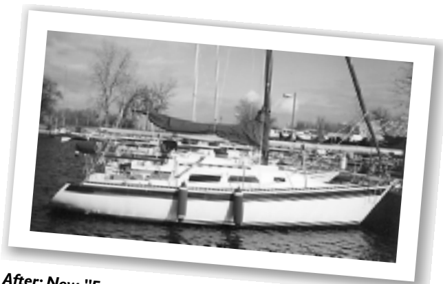
After: New "French stern" extension blends in nicely with hull lines.
