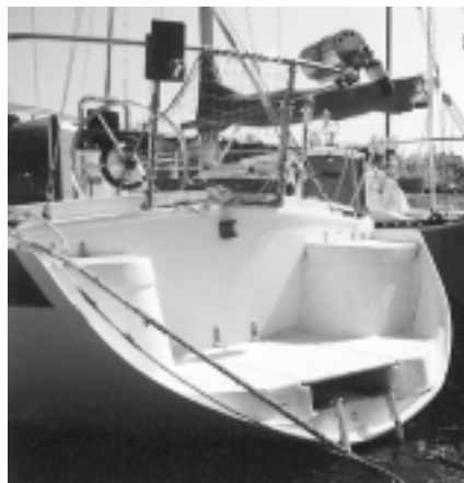
Plywood floor laminated in place with cored inner skin, floor cavity filled with foam, ready for finishing with gelcoat.
