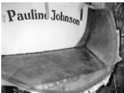
Plywood floor laminated in place with cored inner skin, floor cavity filled with foam, ready for finishing with gelcoat.
