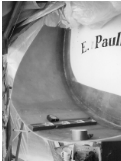
Mold removed and outer skin laminate trimmed to desired shape. Note tangs on top edge and transom flanges for bolting and supporting the extension floor.
