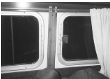
(top) New windows are set in from the outside leaving no channels to lodge dirt and trap moisture; (bottom) Inside view of window clamps.
