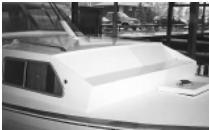
Finished full-width foredeck seat, fiberglass deck and cabin top, and new windows.
