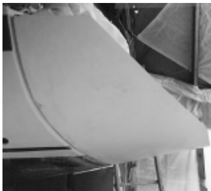
Extension bolted temporarily in place. Take a close look: if you don't like the shape, scrap it and start over.
