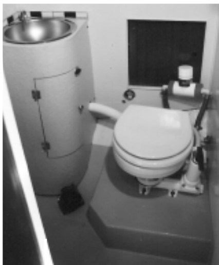
Original head compartment required moving bulkhead and reshaping floor to accommodate larger Ecolet. Instructions for building the curved locker shown on the left appeared in "Good Boatkeeping," DIY 1998-#4 issue.
