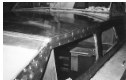
Cabin top and sides coated with epoxy resin.
