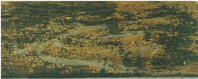
Highly caustic two-part cleaners chemically react with the teak, turning it black, then orange and expose the wood layer underneath.
