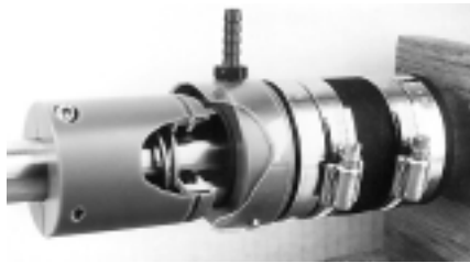
Vent line combination water-injection hose barb on the Lasdrop Gen II prevents air locks in slower-moving hulls or provides cooling water for planing hulls.
