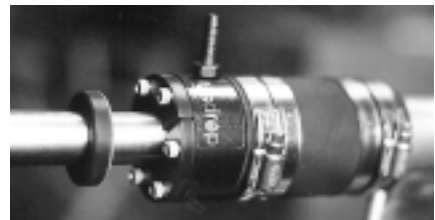
Lasdrop Dry-Seal's split-face plate design allows quick in-water replacement of the inner lip seal.
