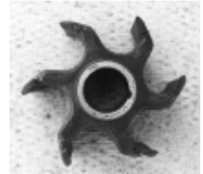
When impeller vanes are cracked or worn or have taken a permanent set as shown, replace the impeller with a new one.
