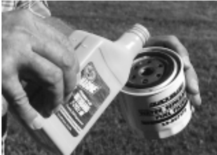
Fuel-injected engines are "fogged" by putting a 50/50 mix of fuel stabilizer and two-cycle oil into the fuel-water separator.
