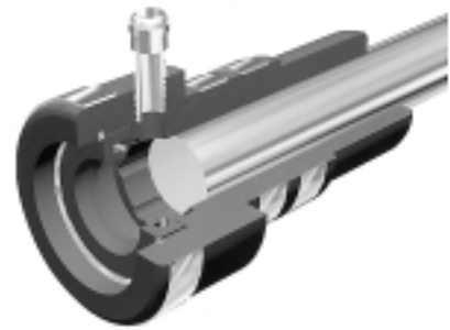
Cutaway of Strong Seal shows the inboard end of the UHMW plastic with the recess that holds the lip seal. Water pick-up connects to engine's raw-water cooling system.
