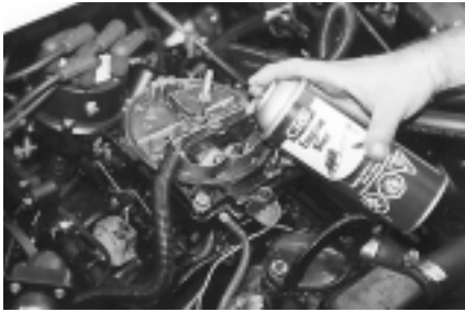
Fogging carbureted engines coats the cylinders with a sticky residue to prevent corrosion.
