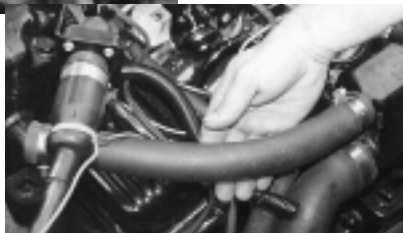
Carefully inspect coolant hoses for signs of softening, cracking or bulging.
