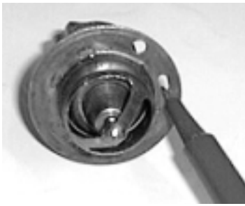
Single-stage diesel engine thermostat showing coolant bypass hole.
