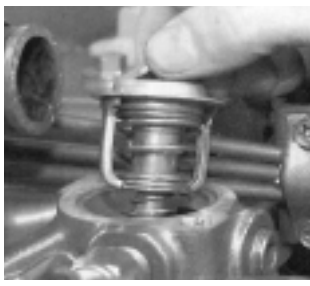
To remove, disconnect coolant hose, remove thermostat housing and lift thermostat.
