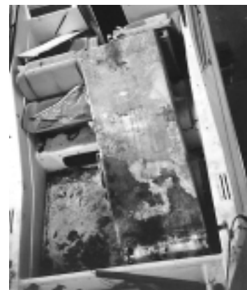
The end of the line: fuel tank replacement costs can be high enough to send a boat to the junkyard.
