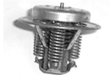
Two-stage gas engine thermostat open at 62°C (145°F).
