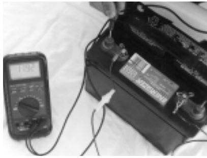
DMM checks loads or voltage drop on an existing circuit before adding accessories.
