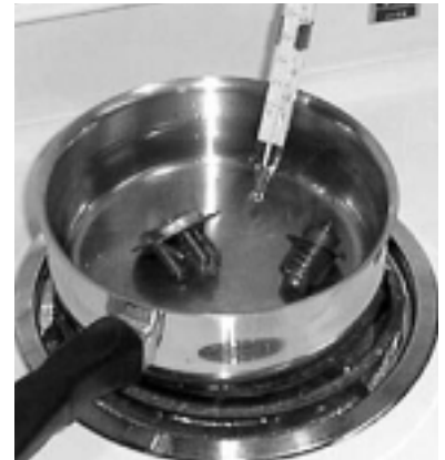
Testing the thermostat: place in water-filled container and heat, then place in cold water. It should open then close quickly without sticking.
