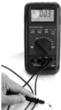
Top: Use the low-resistance scale to test a fuse. Left: To test equipment for resistance, disconnect the circuit (otherwise, you will measure the entire circuit), set selector switch to the proper resistance scale and connect test leads, red to the positive side. Defective equipment will have no resistance reading.
