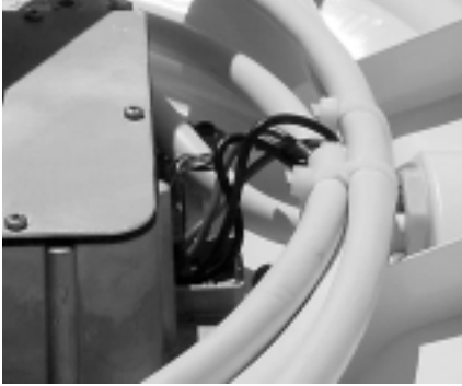
Never cut or splice the multi-conductor antenna cable; instead coil extra cable in the base of the dome.
