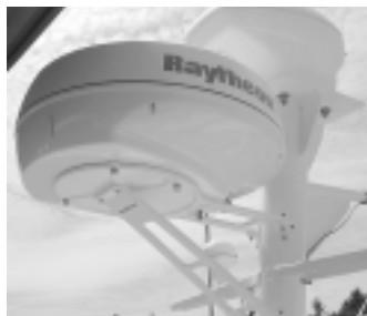
Scanner must be securely mounted but and high enough to keep the transmitted energy safely above an area where people may be and above other antennas: (top) Fixed bracket-mounted antenna on short mast on author's Tollycraft; (center) Edson NavCom Tower Systems provide a single mounting pod for radar, GPS or VHF antennas, flood lights and other accessories; (bottom) Gimballed, self-leveling sailboat bracket mounts pole connected to the backstay.
