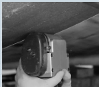
Peeling a 32-footer took three hours, removed about 90% of the gelcoat and required minimal sanding to ready the hull for recoating.
