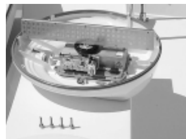
Inside view of a dome scanner shows the antenna, drive motor, transmitter, receiver and antenna position sensor.
