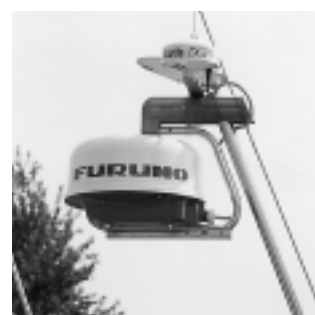
Scanner must be securely mounted but and high enough to keep the transmitted energy safely above an area where people may be and above other antennas: (top) Fixed bracket-mounted antenna on short mast on author's Tollycraft; (center) Edson NavCom Tower Systems provide a single mounting pod for radar, GPS or VHF antennas, flood lights and other accessories; (bottom) Gimballed, self-leveling sailboat bracket mounts pole connected to the backstay.
