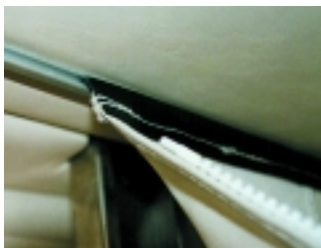
(right) An inside view through entryway; (below) bolt rope sewn to canvas slides in a channel mounted on the hardtop.
