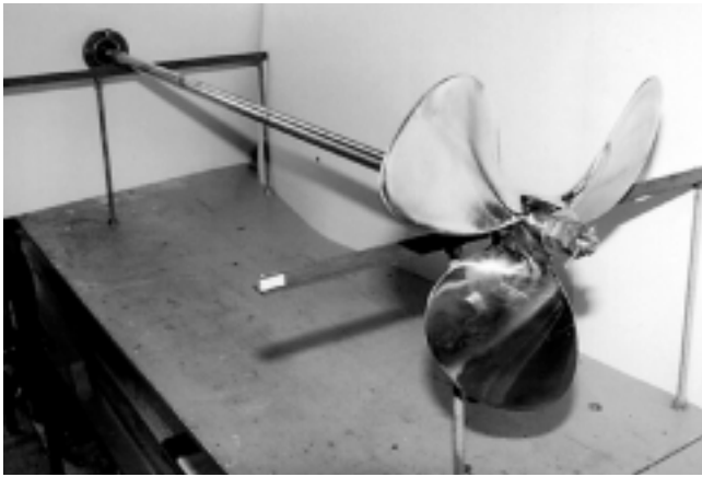
DIY jig for balancing props.
