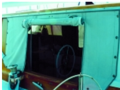
(right) An inside view through entryway; (below) bolt rope sewn to canvas slides in a channel mounted on the hardtop.
