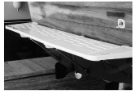
Modern looking platform made of StarBoard makes a nice addition for this classic cruiser.
