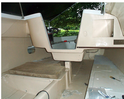
Interior nearing completion with cushions installed. I still need to paint the vee berth overhead and install a padded panel. Wood bullnose molding, stained and varnished, hides the hull-deck joint and wires. It cost about $30 to trim the interior.
