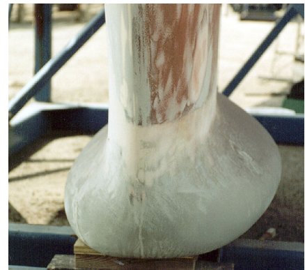
After installing the Torpedo Bulb, the keel-bulb joint is faired with a mixture of epoxy resin and microballoons.
