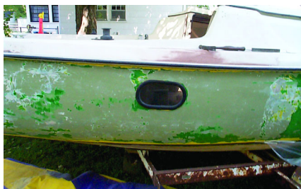
Scraping two coats of paint off the hull was a time consuming and tedious job.
