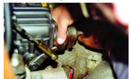
Checking for movement in the keyway.
