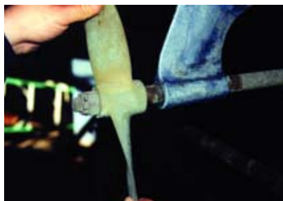
Checking for play in the cutlass bearing.
