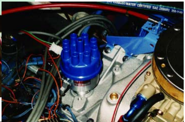
Multiple Spark Discharge units installed on each engine deliver a spark 10 times more intense than a regular coil and distributor.
