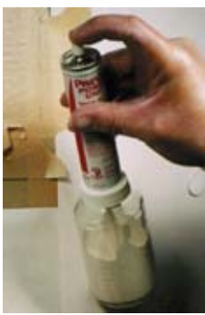
Preval, a disposable spray gun available at auto-body supply shops and some BoatUS stores, comes with its own supply of propellant, thus eliminating the need for a compressor.
