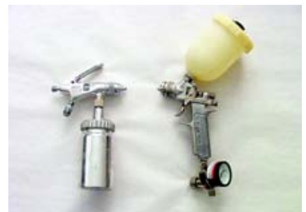
DeVilbiss guns, a siphon feed touch up gun (left) and a small gravity feed gun with a regulator for setting compressor output, costing $200 to $300 each, are better suited for paints as they clog easily and easily ruined by poor cleaning.
