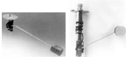
Common float-arm type fuel sender.
