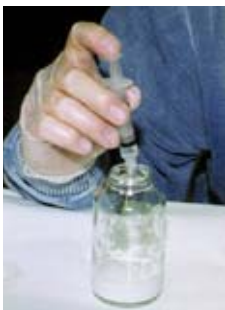
A syringe allows accurate measuring of the amount of MEKP required to catalyze the gelcoat resin.
