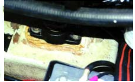
(left) A typical engine mount with slotted base and adjusting nut that raises or lowers the engine to reposition the transmission coupling. (right) Deteriorated engine bed.
