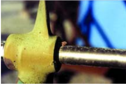
Worn shaft key must be replaced.
