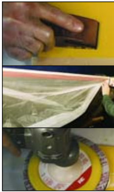
Resist the temptation to sand spot repairs with your hand or fingers, or hurry the job using a power sander. Always sand with a backing block of rubber, wood or hard felt.
