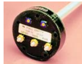
Probe type sender has no moving parts. Constructed of one small tube inside a larger tube, the inner tube acts as a capacitor, measuring air volume as fuel level changes in the tank and activates the sending unit.
