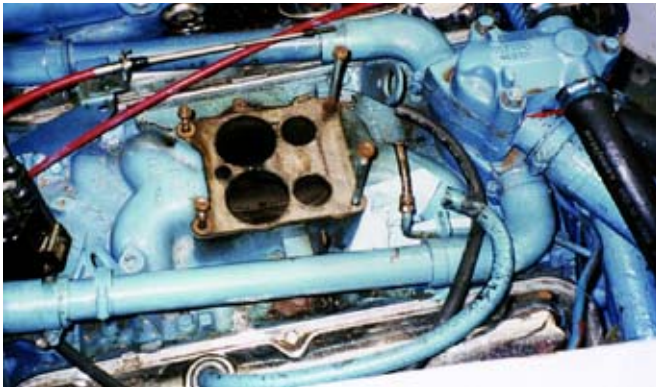
Original cast-iron intake manifold.
