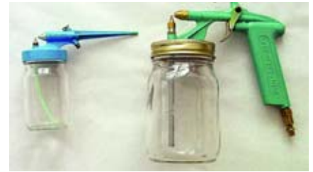
Inexpensive siphon spray guns, Badger model 250-4 (left) and Canadian made Critter model 118, both cost US$40 or less, are the best choice for gelcoat repair jobs. Catalyzed gelcoat is sucked up the tube by the air passing over the venturi, creating low pressure. Varying the height of the venturi increases or decreases the flow rate.
