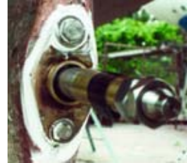
(top) Strut assembly. (middle) New cutlass bearing installed in stern tube. (bottom) Seizing wire locking screws prevents shaft locking screws from loosening.
