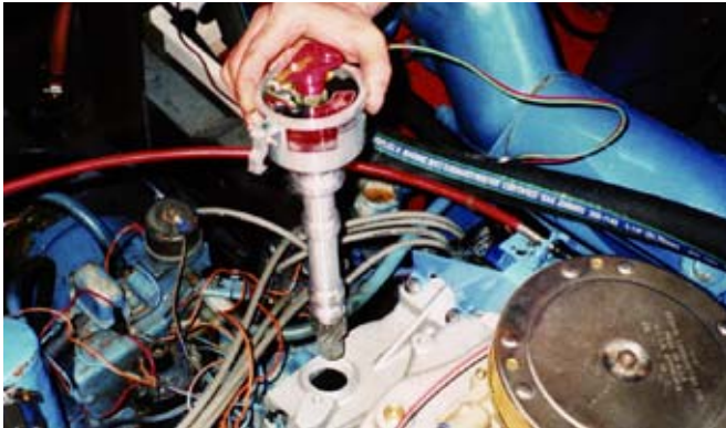
Installation of Mallory electronic distributor.
