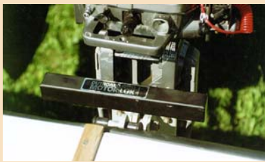
Fulton Outboard MotorLok has a locking mechanism on the bottom.
