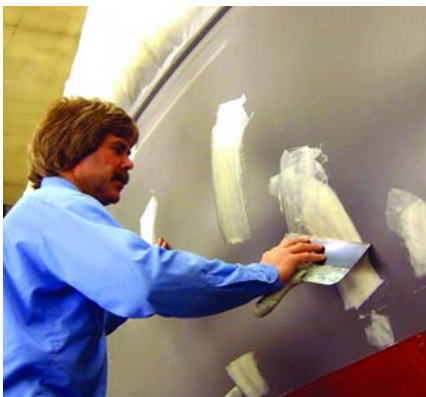
Hadcock applies surfacer with a drywall putty knife to squeeze it into minor surface imperfections.
