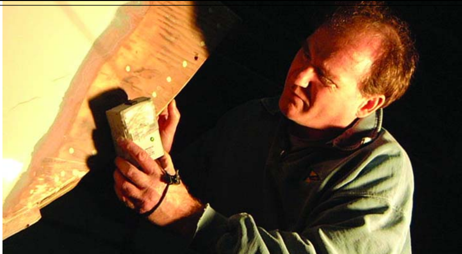
During a routine pre-launch moisture inspection, the author discovers a water soaked bow on his '60s vintage glass-over-ply Thunderbird.
