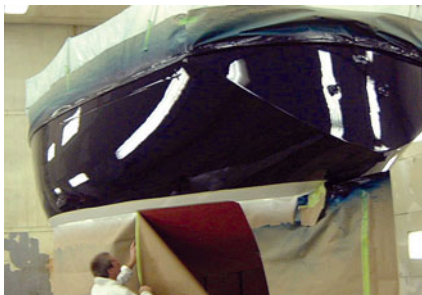
Mask removal is done as soon as possible after the paint has cured.
