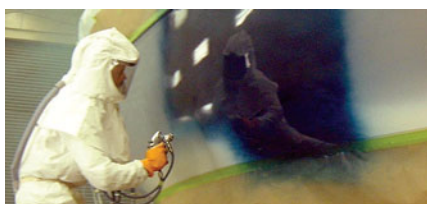
Applying hull topcoat.
