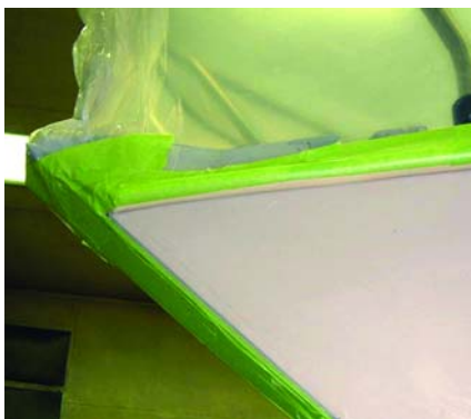
Plastic shroud encloses the deck and cabin of the boat in an air and dust tight cocoon.
