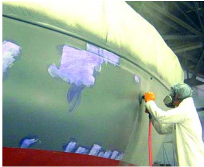
Final prep sanding of epoxy primer with 320-grit paper.
