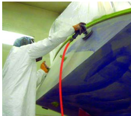
Prep sanding with a dual action (random orbit) air sander fitted with 15cm (6") sanding disc. Note blue wash on the hull as a sanding indicator.
