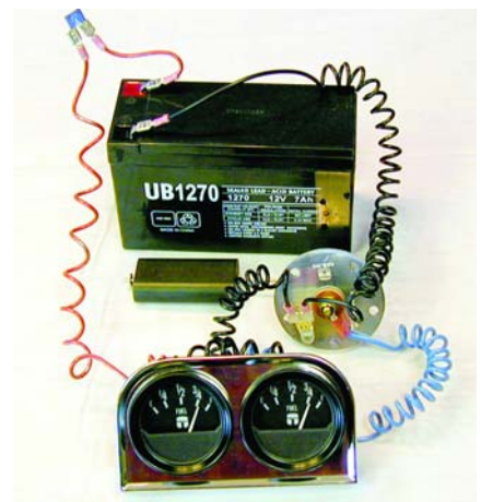
Two gauges in parallel using a single-gauge rated sender. Note that the gauges don't read full even though the sender float is fully in the full position.
