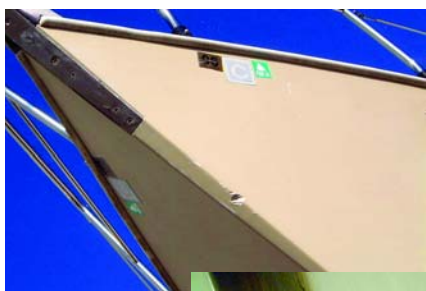
(top) Bow close-up before painting showing ding. Decals and some hull fittings will also be removed.
