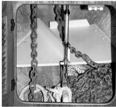
Mold on surfaces in anchor locker forms in a buildup of condensation compounded by poor ventilation.
