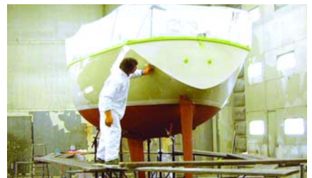
In the spray booth, polyurethane paints demand the controlled environment of a spray booth for best results.
