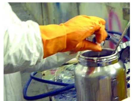
Viscosity dilution check of the topcoat with reducer for proper spraying is gauged by the amount of time the calibrated cup takes to drain. Mixed topcoat is poured one batch at a time into the pressure pot then small amounts of additives are added.
