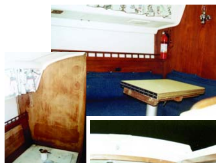
Interior woodwork was cleaned, sanded and refinished with four coats of gloss WoodPro.
