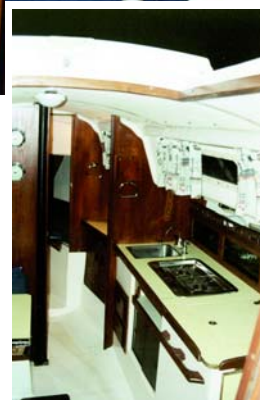
Interior woodwork was cleaned, sanded and refinished with four coats of gloss WoodPro.
