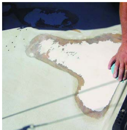
After filling and fairing babystay location is block sanded in preparation for gelcoat or paint.
