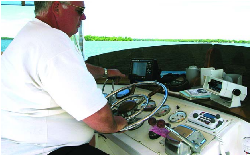
At-a-glance instrumentation, each gauge contains port and starboard meters with red pointers to easily reference gallons per hour or speed and engine rpm (right). Throttle settings are adjusted for the most economical speed versus fuel consumption ratio as indicated by the LCD digital meters.
