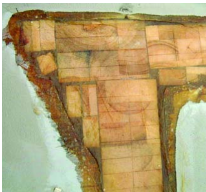
Close up of replacement core potted in place at babystay location prepped for upper laminates.
