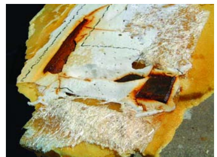
Close up of the mild steel web exposed after the loss of the skins shows it partially encased in solid filler but the greater volume of the rudder interior is foam.
