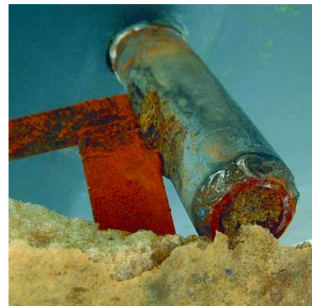
Close up of the broken rudderstock. The failure occurred where the lower stock, a smaller diameter stainless pipe, was inserted into the upper stock and welded in place. Some corrosion can be seen but striking a submerged object may have caused this failure.
