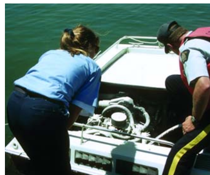
Thick residue from a portable chemical fire extinguisher coats the entire engine compartment, means an expensive cleanup for this unfortunate boatowner
