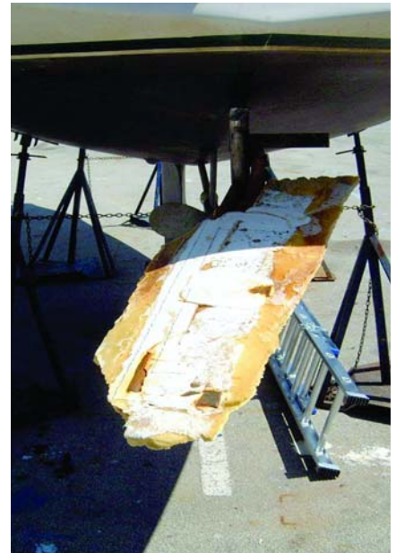
This rudder suffered a sudden breakage of the rudderstock, folded 90° and had the rudder skins peel off completely.
