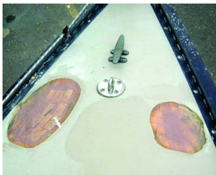
Bow pulpit repair shows new core "potted" in place with chopped fiber and resin.
