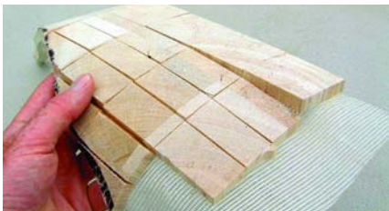
A piece of new balsa core ready for installation.
