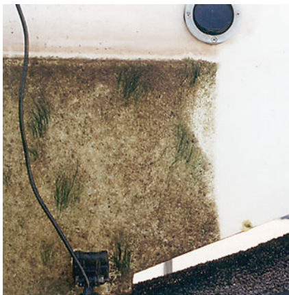
(left) Transom of DIY's test boat coated with a bottom wax shows build up of slime. (right) Always water test the hull after cleaning to ensure all wax is removed. Repeat the cleaning on any areas where water beads.
