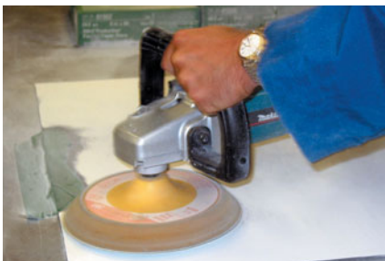
(counter clockwise starting at the top) Test panel with coats of soft antifouling (Bottomkote XXX); Surface is lightly skimmed over with 3M Fre-Cut 24E on a 3M Skikit pad and dual-action sander running at 3,000 rpm; The trick is not to dwell — it took less than 10 seconds to break the paint adhesion on the 61cm (2") square test panel and expose the original white surface; Remaining paint residue is removed with 60 grit; Final finish with 80-grit sandpaper is similar to a primed surface, though some paint systems may need to be sanded finer with 120 grit.
