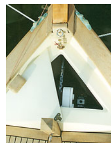
A horizontal windlass easily fits in the anchor locker and is simpler to install and maintain.
