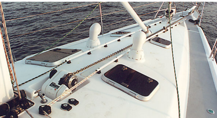
Windlass is best mounted mid-deck rather than adding uncalled-for weight on the bow.
