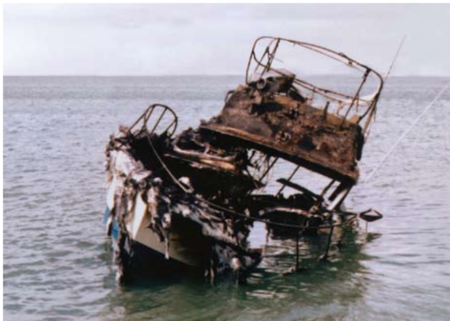
The aftermath of pouring gasoline into a fish rod holder: After mopping up the gasoline in the bilge, the skipper of this sportfisherman in Texas thought it was safe to start the engine. What he failed to account for were the fumes that remained.
