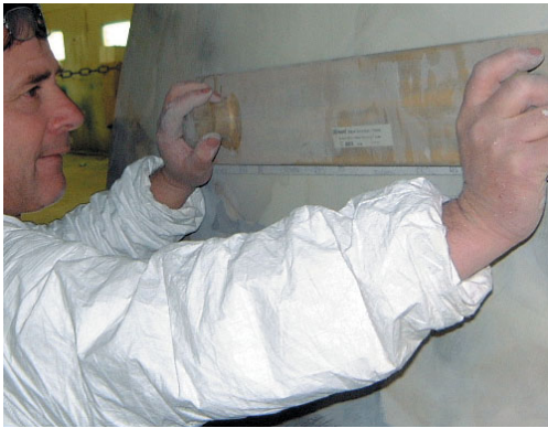
(left) 3M Fairing Board in action. (right) Coarse sander in action. Tool must be kept nearly flat to prevent swirl marks in finish.
