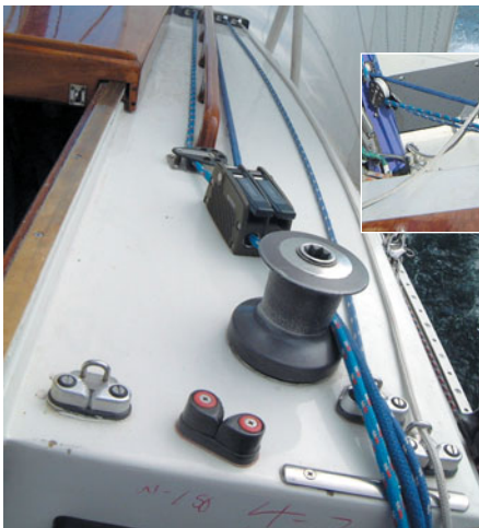
FIGURE 4 (left) Keep-it-simple outhaul and main halyard lead to a rope clutch and winch. (inset) Deck organizer in action.
