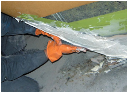
Shaping a curved leading edge with a flexible plastic spatula.
