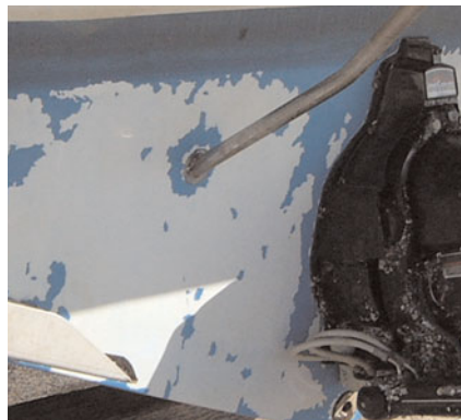
Badly chipping paint indicates poor original prep, as hull surface is still glossy! Needs to be stripped.
