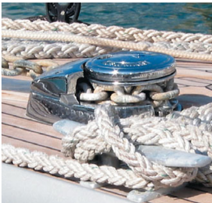
Low-profile vertical windlass on small cruiser easily manages chain (or rope) anchor rode to provide secure anchoring with less scope.
