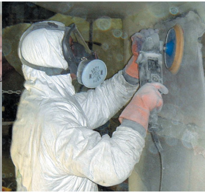
(left) 3M Fairing Board in action. (right) Coarse sander in action. Tool must be kept nearly flat to prevent swirl marks in finish.
