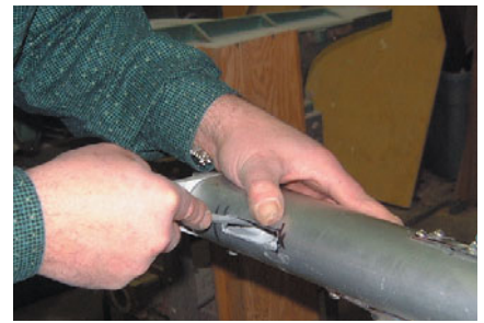
FIGURE 6 When sheaves are not integral, flush-mount the block by cutting and filing an opening in the base.
