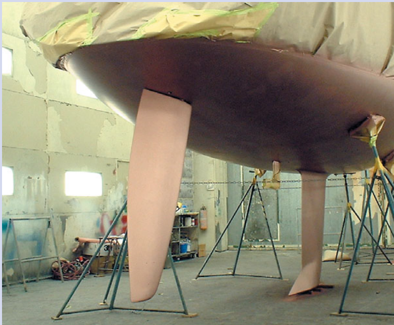
New VC 17m Racing Bottom. The copper color darkens after immersion.
