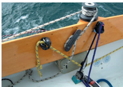
FIGURE 8 Rigging a backstay: (clockwise, top left) Backstay attaches to 6:1 double ended tackle in the aft locker; 2:1 wire cascade enters deck at block; Yellow line exits the aft locker and follows the cockpit perimeter (both sides); Secures to a cleat on both port and starboard coamings.
