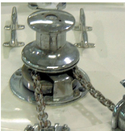
A vertical windlass mounts the electric motor and gearbox on the underside of the deck.
