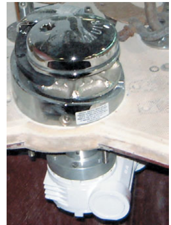
Vertical windlass requires a deeper rode locker to make room for the windlass drive and anchor rode.
