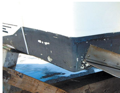
Typical epoxy ester shows some paint build-up and chipping. Scrape loose paint and lightly scuff sand to prep for recoat.
