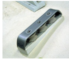
FIGURE 11 Triple organizer has a shim to compensate for deck camber cut from King StarBoard.
