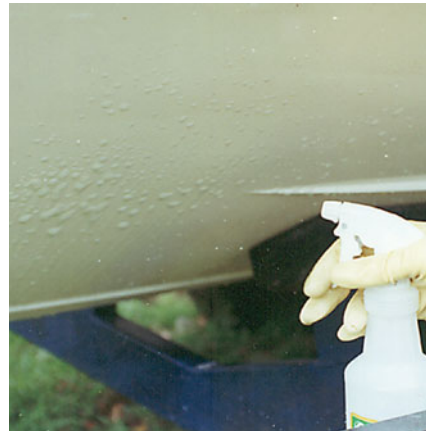
(left) Transom of DIY's test boat coated with a bottom wax shows build up of slime. (right) Always water test the hull after cleaning to ensure all wax is removed. Repeat the cleaning on any areas where water beads.
