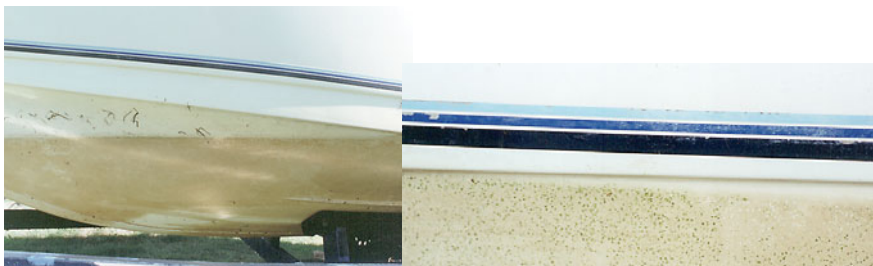
Multiple coats of QuickCraft bottom wax didn't prevent slime growth along the waterline and hull bottom after four weeks in freshwater.
