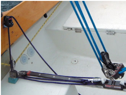
FIGURE 3 Ball bearing traveler with 3:1 cross-haul cleated on the coaming.
