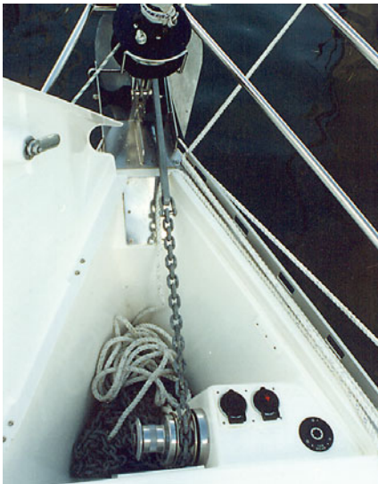
Anchoring package complete with up/down/off switches all neatly stowed in foredeck locker.
