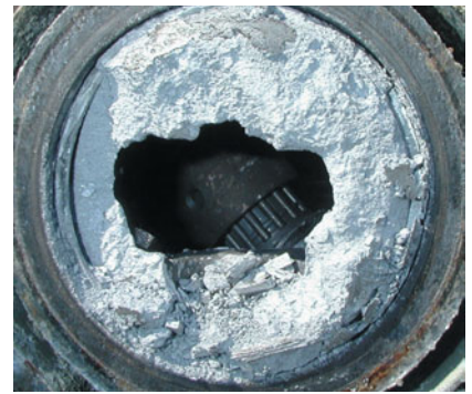
Note how the detonation shock wave has literally pulverized the top of this piston.
