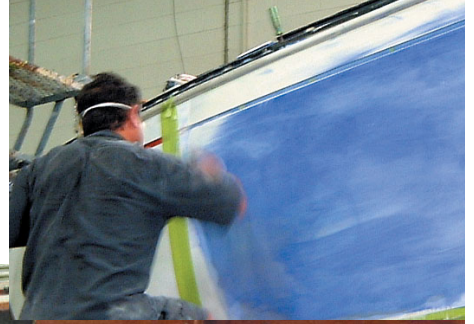
(top, below) Blue dye applied as a visual aid to filling and fairing. (bottom) Blue dye patchwork remaining on this hull after preliminary board sanding indicates many low spots requiring more filler.
