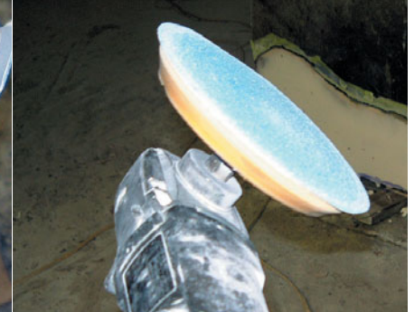
(top left, clockwise) Detail sanding to fair a flat surface requires a sanding block; 3M Fairing Board uses special self-adhering Hookit paper; Low-speed sander/polisher fitted with a 20cm (8") foam pad and 60- to 80-grit self-adhering sanding disc for coarse sanding; Dual-action sander with 15cm (6") foam pad and 80- to 120-grit Velcro disc for fine sanding.
