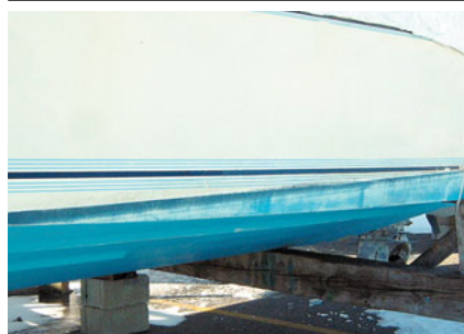
Waterline wears but the otherwise good condition of this paint means it's an ablative type, most likely multi-season copolymer.
