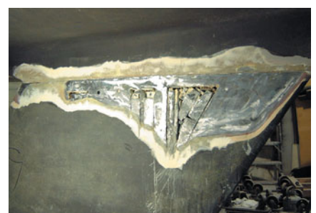
Keel repair prepped for initial putty application.
