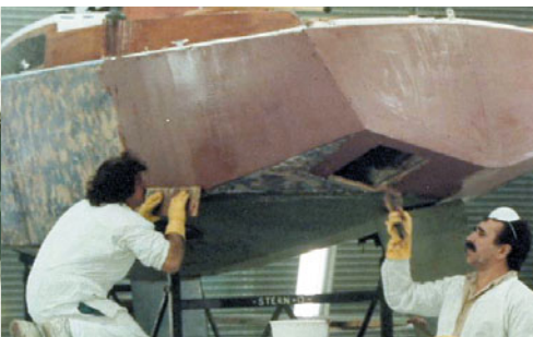
Leveling or "screeding" filler with a piece of scrap Plexiglas. Also touch ups with a small 10cm (4") putty knife.
