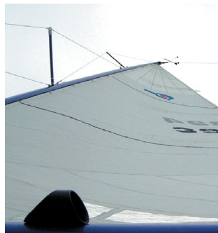
FIGURE 1 A depowered main. Note minimal draft due to full outhaul, cunningham and halyard tension, lots of backstay to bend mast and pull sail flat also eases the leech plus significant backwind due to eased traveler.
