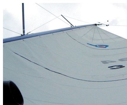
FIGURE 2 A powered-up main has deep draft, straight mast, tighter leach and very little backwind.
