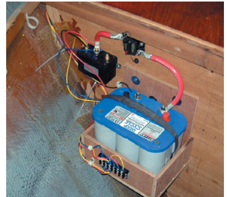
Dedicated battery mounted in the bow reduces wire size. Battery must be installed in a sealed case and away from any ignition sources.
