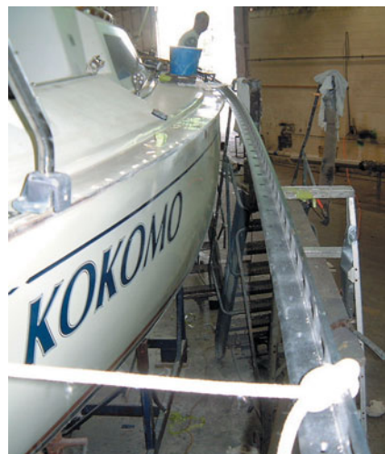
New toerail arrives as a straight section and is bent into place.
