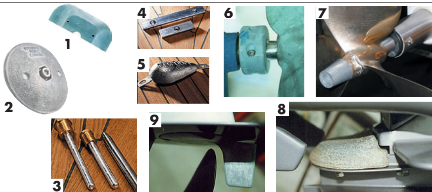
1 Magnesium anode for freshwater use only. 2 Streamlined disc anode bolts directly onto the rudder forward edge or trim tab; 3 "Pencil" anodes for engines and heat exchangers; 4 Power trim bar anodes; 5 Anode with tabs for attaching to a bonding wire; 6 Two-piece collar anode mounts directly over the shaft; 7 Bolt-in-place prop nut zinc; 8 Anode mounted on outboard gearcase, 9 Sacrificial zinc trim tab on outdrive.
