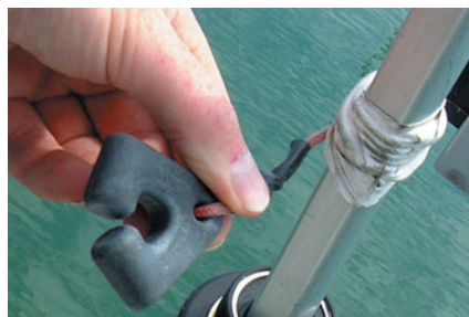
Prefeeder simplifies loading a headsail into the groove.
