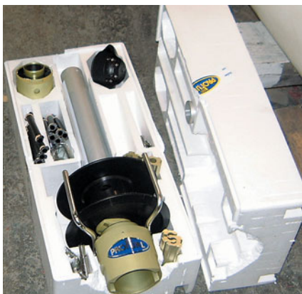
Profurl kit complete with everything needed to mount over the existing forestay and turnbuckle without mods to the rig.
