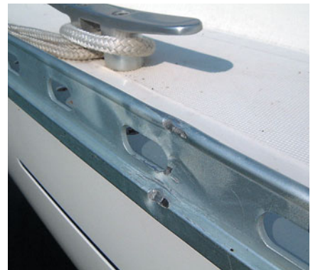
A candidate for replacement: any repairs to this damaged aluminum rail will show through the clear anodized finish.
