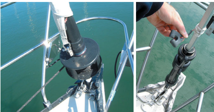
Race-ready Harken furler with drum removed, upper swivel dropped to bottom of stay exposing double groove headstay system. Note pre-feeder for smooth headsail changes.
