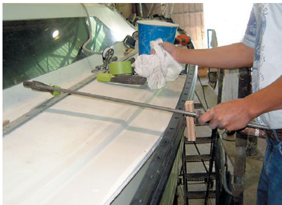
Using a large C-clamp to bend the rail.
