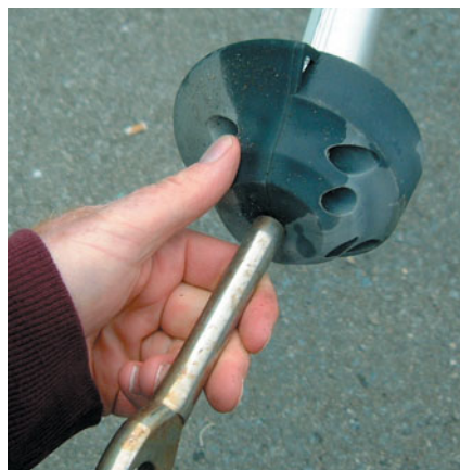
Profurl’s patented Wrapstop eliminates halyard wrap.
