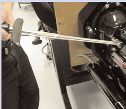
Rugged, durable and inexpensive, a beam wrench is the most common one used in engine repair.
