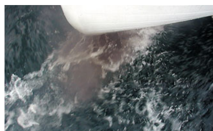
A sailboat engine "lugging down" because it's overpropped, a very common problem.
