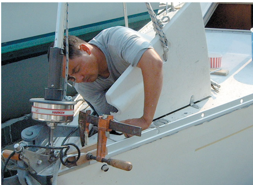
Installing the last fasteners. Note butyl sealant squeezing out at the lower edge.
