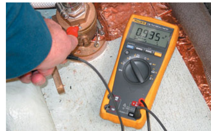
The reading taken at this bronze seacock (935 mV) indicates it's actually overprotected, although not dangerously so. Note the copper bonding strip.
