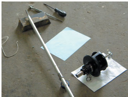
Cut forestay to the required length, if required.
