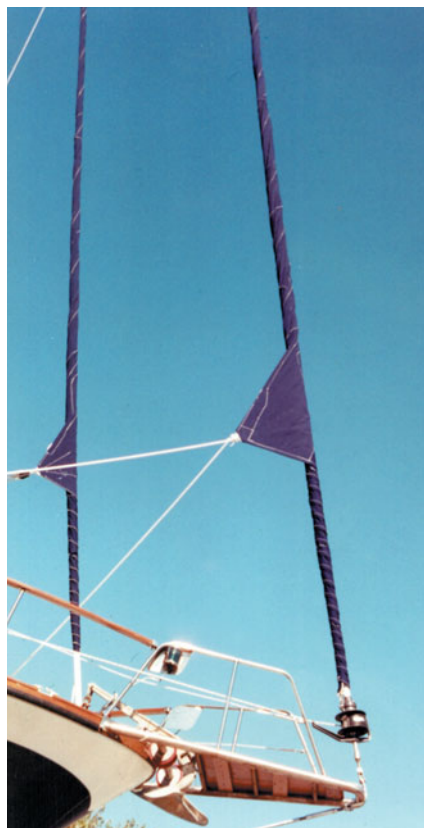
A sample installation. Photo is of the Canadian-made Ultra-Furl, an affordable furler for cruising boats with dual-aft facing grooves, stainless-steel bearings and a two-piece aluminum extrusion that feed over the existing stay. Distributed by North Sails (Toronto).
