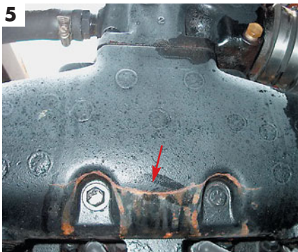
5 Manifolds also crack in the same areas.
