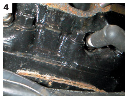
4 Because of the design of the internal cooling chambers, freeze damage in cylinder blocks usually shows in the same areas.
