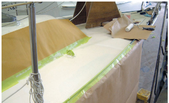
New "stucco" style deck anti-skid applied by roller on the C&C 25.
