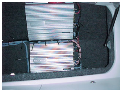
In this case, the amps are screwed down to a carpet-covered Ozite board mounted in a storage compartment. Notice the wires are tied together with wire ties to assure a clean installation.
