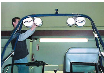
A tower is the perfect mount for speakers. These speakers from MB Quart were custom installed in enclosures then mounted on stainless steel brackets that bolt to the tower. All speakers face toward the back of the boat.
