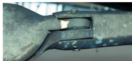
If the hub and pin are worn the hub will show a gap between the blade core and hub.
