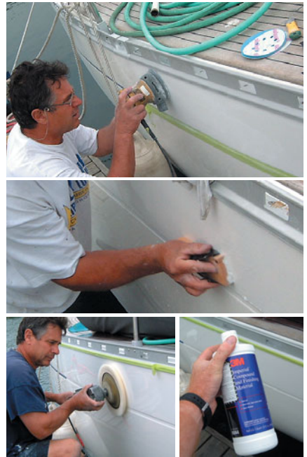
(top) Dufour 38: After spraying and cure, new gelcoat is dry sanded initially up to a 400-grit finish with a dual-action sander. (middle) The repair is then block sanded by hand with progressively finer wet sandpaper up to an 800 or 1,000 grit finish. (bottom left) Finally buffed to a gloss with polishing compounds. (bottom right) 3M Marine makes a full range of polishes for each stage of the process.
