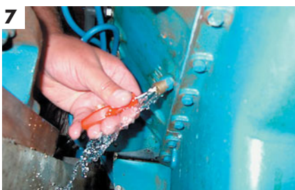
7 Using a small screwdriver as a probe will open a blockage of sand or silt and allow complete drainage.
