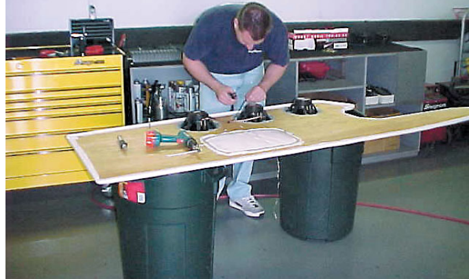
(above) Sounds Good Stereo installer wires three MB Quart 8-inch two-way coaxial speakers on to a side panel of a ski boat. The panel was removed from the boat, the speakers were mounted on it and then the panel was reinstalled (left). That's plenty 'o sound mon!
