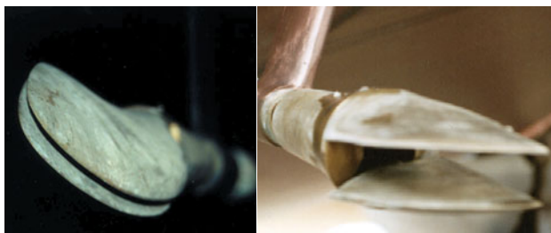
Blade clearance between the edges of the blades should be at least 6mm (1/4") on a Martec prop. (bottom) The two blades should lay parallel, the gap the same at the tip as at the base.
