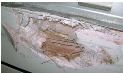
Dufour 38: Core exposed at hull puncture creates danger of water entry into core.
