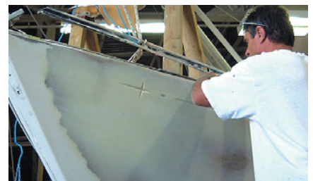
(top) Filling and fairing: First fill on Dufour 38 ready for sanding. More fills will be needed. (bottom) First fill on C&C 27 repair.
