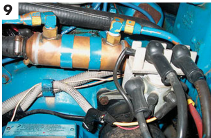
Your engine may have several engine oil coolers and or transmission oil coolers. Disconnect and drain the hoses is the most positive way to be sure the unit is protected.
