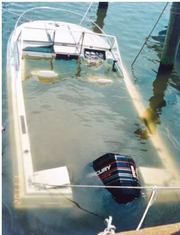
Water from the sky—not from below—is the most common reason outboard boats sink at the dock. A partially clogged drain is all it takes to make a boat's stern heavy enough to allow water to backflow through scupper drains. The best defense (aside from hauling out) is a close fitting cover that directs water overboard.
