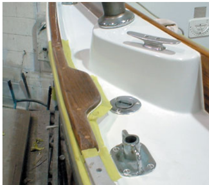
Damaged areas of teak caprail are replaced by new teak glued and scarfed into place and then given the necessary multiple coats of varnish.
