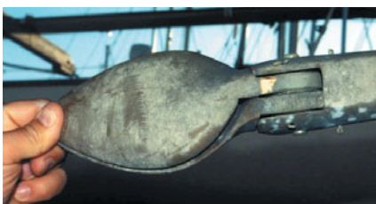
Close the blades and inspect for a gap between the inside of the blade tips. They should not touch.
