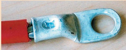
Little or no wire should be visible outside the lug.
