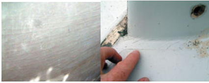
left) Viking 34: Sometimes stress cracks are hard to spot. This photo represents about 1.8 square meters (2 square feet) of hull, .6m (2') below the impact point. (right) Other stress cracks are easy to see but may just be the tip of the iceberg.
