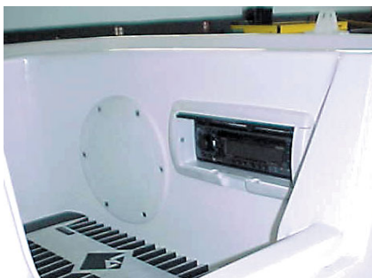
A large nook like this one stows the head unit, a speaker and amplifier. The compartment is away from water, dry and sealed. Fans were installed to cool the amplifier.
