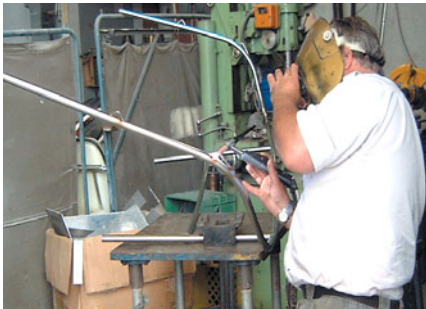
(bottom) New tubing is cut and shaped for fit prior to welding. (left) Welding stainless steel is followed by careful polishing.
