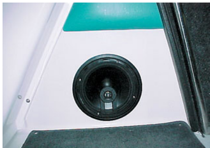
A panel makes a good location for a coaxial speaker.
