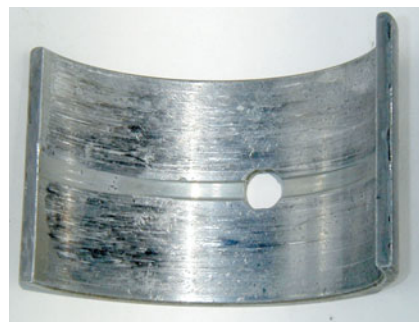
High lead and tin levels in the oil showed the extent of the damage to the main bearings after this engine ran low on oil when the hose to the oil cooler failed after chafing on the oil filter bracket.
