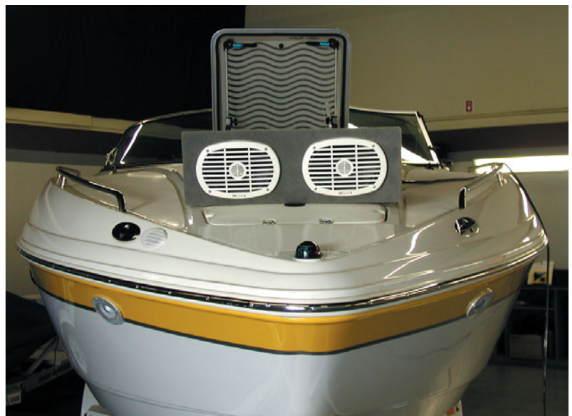
(left) Compartment constructed of medium-density fiberboard covered with fiberglass on the outside and carpet on the inside to serve as a mount and protection for a CD changer. (bottom) A custom panel holds two 6x9 speakers.
