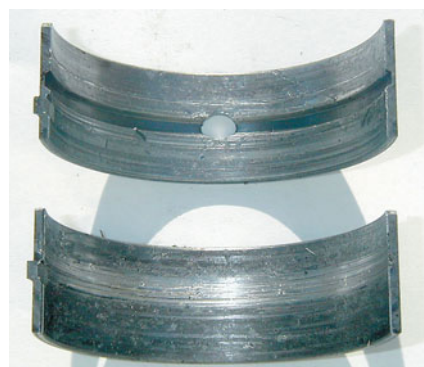
High iron, lead, tin and oxidation levels predicted the debris damage to this main bearing and its cause. Several camshaft lobes distempered from friction and wore flat because the oil broke down after a worn-down raw-water pump impeller cam caused the engine to run at an elevated temperature.
