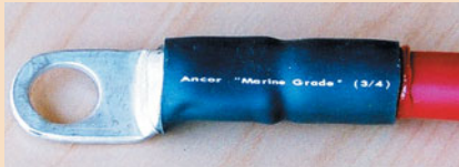
A heat gun produces the best results when shrinking tubing. Note how the adhesive is squeezed out forming a watertight seal.
