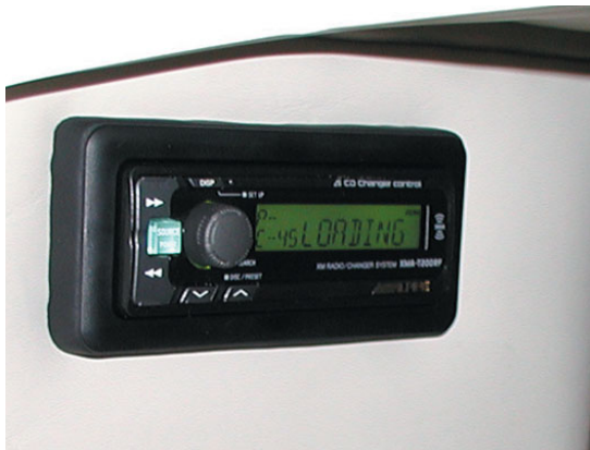
A CD changer control in a custom-made enclosure and mounted to a cabin bulkhead.
