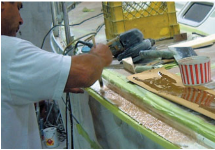
Dufour 38: Chasing bubbles out of a (relatively) small glass repair on a deck flange.
