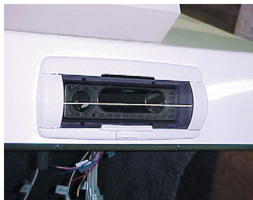
Head unit securely mounted. An optional plastic cover fits over the unit to protect it from water.
