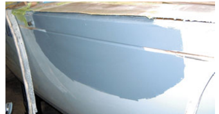
C&C 25 hull repair after priming. Ready for final sand and polyurethane painting.
