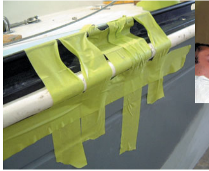
(left) A broken vinyl rubrail is rejoined and bonded together in the hull-to-deck joint on the C&C 25. (right) Gouges in vinyl can be filled, faired and painted using special vinyl repair products.
