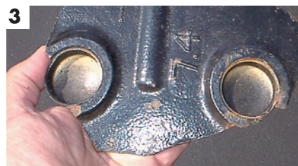
3 What was left of a 454 engine block after a quick cold snap. Note that both welch plugs are still in place.
