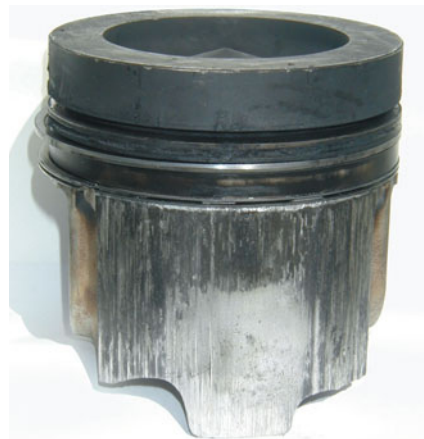
Very high aluminum levels in the oil helped determine how badly this engine was over-heat damaged when the raw-water pump drive belt broke.
