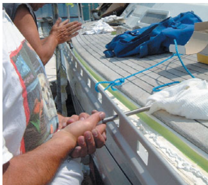
A new toerail is bent and fastened into place with lots of sealant.
