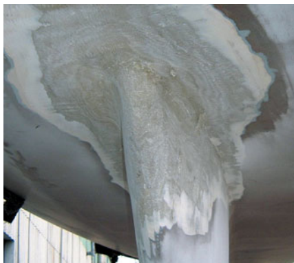
(above) After filling and fairing, epoxy primer or barrier coating is applied. (right) New interior work is painted with air-dry gelcoat or epoxy paint.
