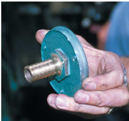
An aluminium plate was cut to size and fitted into the original base with epoxy adhesive and pop rivets. The plate was then drilled to accept a brass skin fitting hose barb of the appropriate size to match the hose barbs on the CCV. This was then fitted to the new base with a backing nut and sealing washers. The unit screws directly back into the engine breather outlet.
