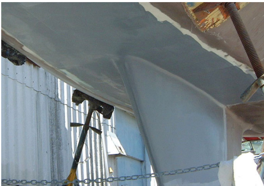
(above) After filling and fairing, epoxy primer or barrier coating is applied. (right) New interior work is painted with air-dry gelcoat or epoxy paint.
