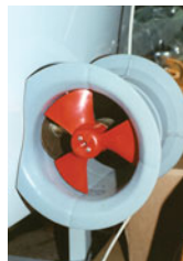
(left) Tunnel-mounted bow thruster in planning hull; (bottom left) Older-style stern thruster; (below right) New design of stern thruster includes a short tunnel.
