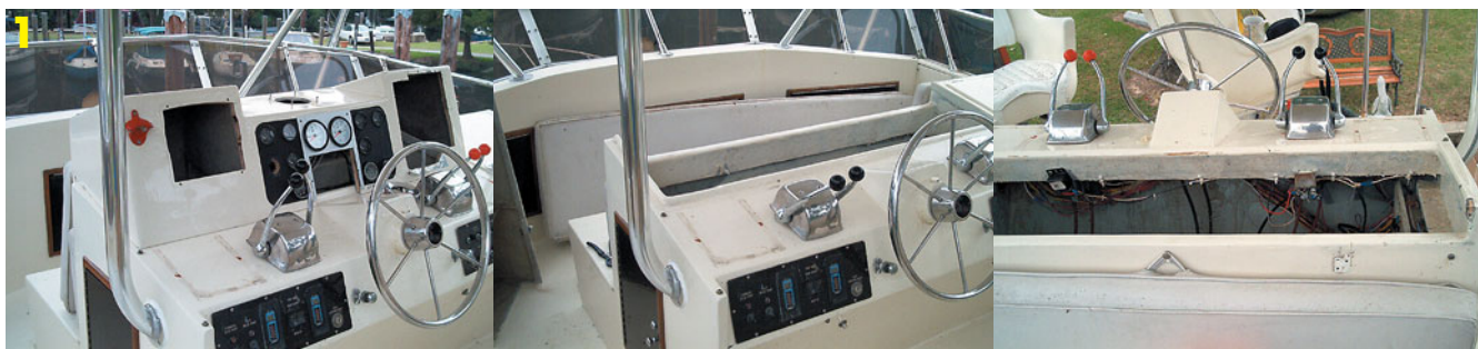
Existing console and instrument pod at the flybridge helm station has hinges on the back for easy access and servicing.
