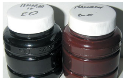
The transmission fluid in the oil analysis sampling bottle on the right tested positive for water contamination.
