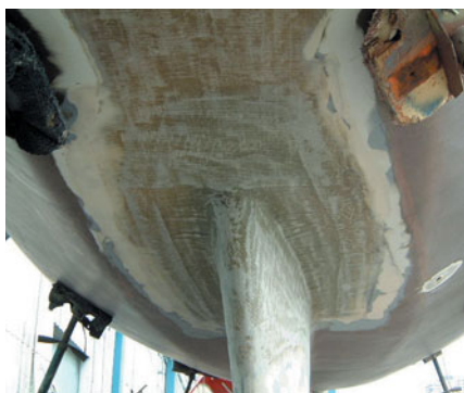
(top) Cut and dry fit the new glass before mixing any resin. (middle) First layers on. (bottom) Layers are lightly ground in prep for subsequent layers.
