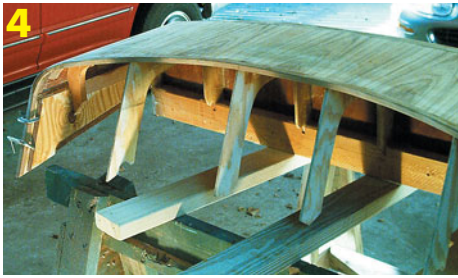
Attaching edge trim. To reinforce the frame before gluing on the veneer, it was sheathed in fiberglass cloth with epoxy resin.
