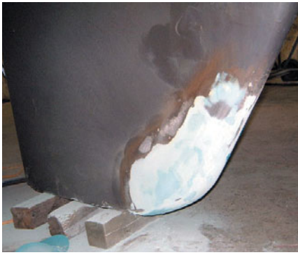
Keel dents shaped, filled and faired.
