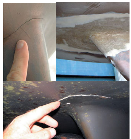
(top left) This small crack on the leading edge of the keel stub may indicate significant hidden damage. (top right) Preliminary grinding shows evidence of delamination where the keel stub meets the hull. (bottom) Tension fracture where the leading edge joins the hull on the same keel. This one leaked!
