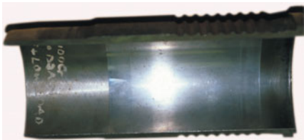
Note how the crosshatch pattern on the unworn section contrasts with the highly polished worn section.
