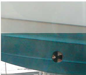
(left) Tunnel-mounted bow thruster in planning hull; (bottom left) Older-style stern thruster; (below right) New design of stern thruster includes a short tunnel.
