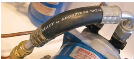
Flare fittings can vibrate loose and leak.
