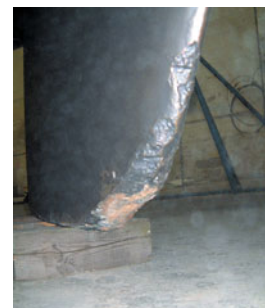
Grounding damage to the keel tip is minor but may represent more extensive, hidden damage.
