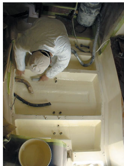
(above) After filling and fairing, epoxy primer or barrier coating is applied. (right) New interior work is painted with air-dry gelcoat or epoxy paint.
