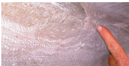
The last bit of delaminated glass (whitish edge) at the keel stub to hull radius must be removed.
