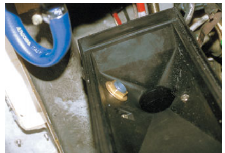
The thru-hull hose barb backed up with a nut inside the air filter box.
