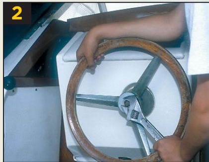
After disconnecting the old cable at both ends, the nut in the center of the wheel is slacked and removed, and the wheel is pulled off the shaft.
