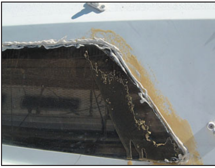
(left) A flush-mounted, bonded window after several amateur leak repairs. (middle) Tired flush mounted windows before add-on frames. (right) Flush mounted windows after add-on frames.
