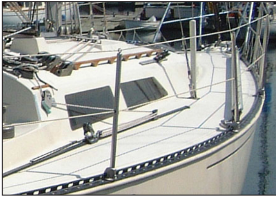
The fastener-free frameless window.
