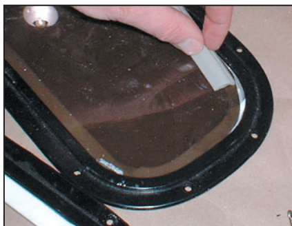
(left) Rubber gasket is pushed in until detent locks in frame. (right) Detent in sealing gasket.
