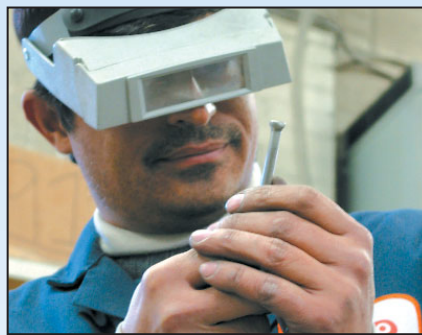
(left) Rod rigging on an '80s Pearson 43 is inspected by a worker at Klacko Spars. (right) Rod end is pushed into the turnbuckle and checked for cracks. Mast termination points are often inaccessible without destroying the rod end.
