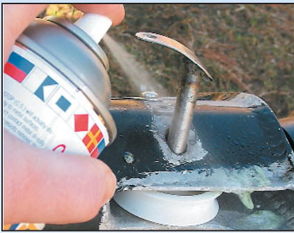
For free-spinning sheaves, remove axle bolt and apply a spray lubricant.
