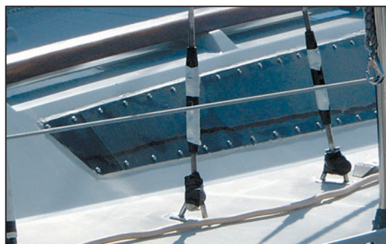
The classic mechanically fastened “Frankenstein” window.
