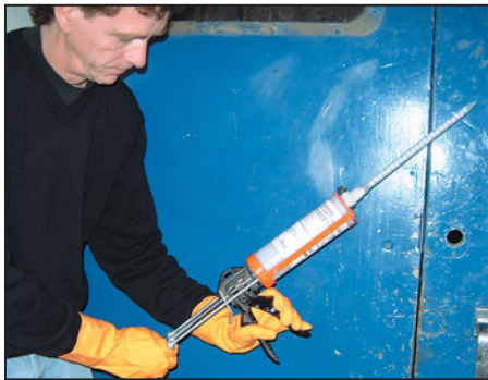
Steven Roll applies Plexus A320 methacrylate using a special adhesive gun.
