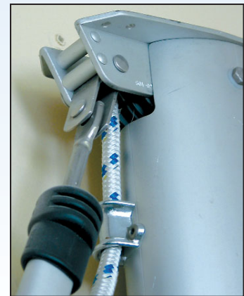
It's common to have a toggle at the bottom of the forestay but more critical is to have a toggle at the top. Put one at the top of the backstay as well.
