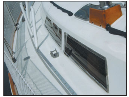
(left) A flush-mounted, bonded window after several amateur leak repairs. (middle) Tired flush mounted windows before add-on frames. (right) Flush mounted windows after add-on frames.
