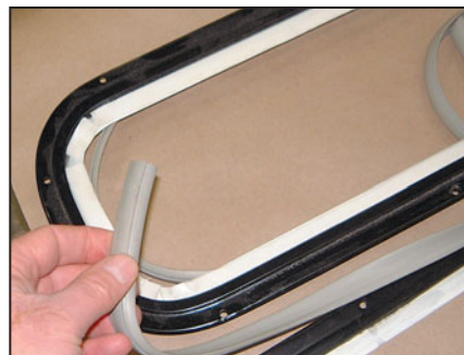
Beclawat aluminum framed fixed port and replacement rubber gasket.
