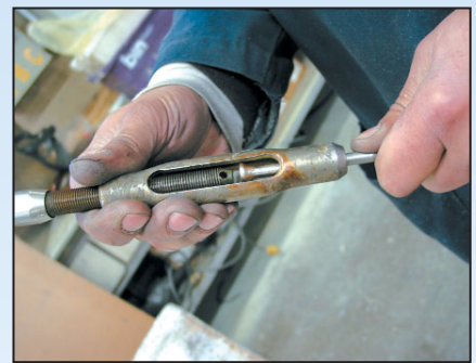
(left) Rod rigging on an '80s Pearson 43 is inspected by a worker at Klacko Spars. (right) Rod end is pushed into the turnbuckle and checked for cracks. Mast termination points are often inaccessible without destroying the rod end.
