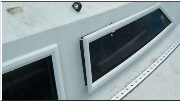
White painted aluminum add-on frame goes over top of flush mounted window.
