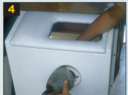
...which made it much easier to unbolt the old steering head for removal.
