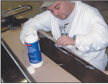
Clean off old sealant and polish the lens before reassembly.
