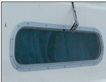
Beclawat aluminum framed fixed port and replacement rubber gasket.
