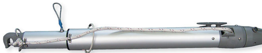
Heavy-duty telescoping whisker pole for a larger boat has jaw outboard end and socket inboard end. This pole features Forespar's patented Line Control. Simply uncleat the external line to adjust pole length.
