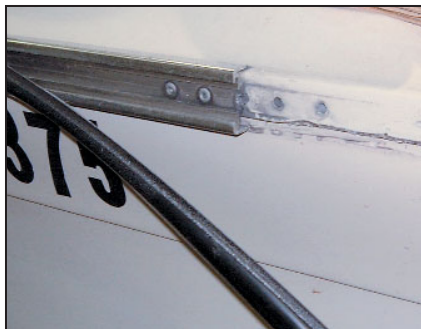
Look for the hull-to-deck joint under the rubrail. Here black vinyl rubrail insert is peeled back to expose the rubrail fasteners (pop rivets).
