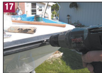
(15) No sealant was applied by the manufacturer under this rubrail.(16) Rubrail was pulled down, mating surfaces solvent cleaned, caulked and refastened (17). On a summer day, you must work quickly when using the 3M Fast Cure version to prevent the sealant from setting up before completing the job. (18) Spilled sealant is easily removed with BoatLife Release adhesive and sealant remover.
