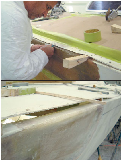
Hull flange reconstruction on a J-35. The deck flange in this case is relatively undamaged and requires little in way of repairs.
