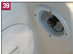
(38) Flojet Quad 11 washdown pump kit (model 4325-143L) includes a pressure nozzle, inline strainer and various hose ports. (39) Pump outlet hose connects directly to an
