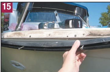
(15) No sealant was applied by the manufacturer under this rubrail.(16) Rubrail was pulled down, mating surfaces solvent cleaned, caulked and refastened (17). On a summer day, you must work quickly when using the 3M Fast Cure version to prevent the sealant from setting up before completing the job. (18) Spilled sealant is easily removed with BoatLife Release adhesive and sealant remover.
