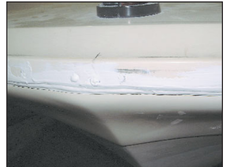
(top) The glass repair on this runabout is complete and the hull-to-deck joint is ready for bedding and fastening. Wedges separate the hull and deck to allow glass repairs to the hull and deck portions individually. (bottom) Hull-to-deck joint is sealed with lots of 3M 5200 and fastened this time with thru-bolts instead of pop rivets.
