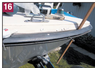
(15) No sealant was applied by the manufacturer under this rubrail.(16) Rubrail was pulled down, mating surfaces solvent cleaned, caulked and refastened (17). On a summer day, you must work quickly when using the 3M Fast Cure version to prevent the sealant from setting up before completing the job. (18) Spilled sealant is easily removed with BoatLife Release adhesive and sealant remover.
