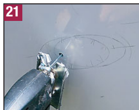
(19) Supplied template helps to properly position docking lights just back from the bow so they point straight ahead with the centerline of the light housing parallel to the water. (20) A 1/32" (.7mm) pilot hole is drilled to be sure there is adequate clearance inside the hull for the light housing. (21) To cut, drill a 3/8" (9mm) hole within the drawn line, insert the jigsaw blade and cut. (22) Heat shrink over crimped terminals provides a waterproof connection. (23) Mounting the docking light. (24) The compact, Paneltronics waterproof circuit panel for docking lights, washdown and one spare is now located where the keyed ignition had previously been.
