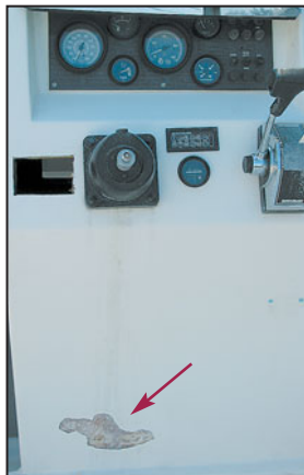
(14) A small pinprick at the bottom of the helm console revealed delaminated fiberglass, resulting in a huge hole to fill.
