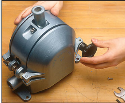
Secure the cover firmly shut with the retaining nuts.
