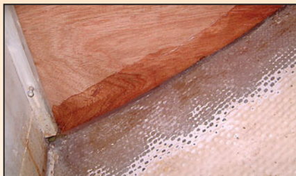
New bulkhead piece in place and ready for filleting. Gap at bottom has been packed with thickened resin.
