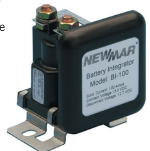
Newmar Battery Integrator allows the single charging output of an inverter-charger to maintain both the start and house battery banks. Batteries are isolated during inverter operation so current draws from the house bank only.
