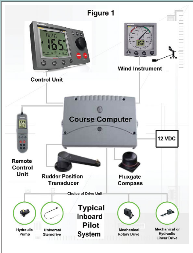
Typical inboard pilot system.
