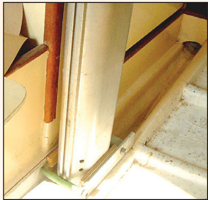
Freshly painted new stringer under sailboat mast step.
