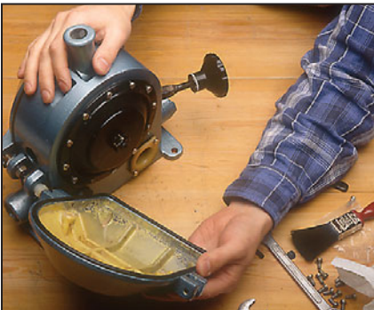
Check the seal is still in position before closing the cover.
