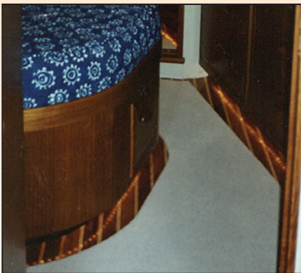
Custom cut and bound carpet is installed over teak and holly sole (floor) 4" (10cm) away from vertical surfaces. Low-voltage rope lighting accentuates high-gloss finish on sole.
