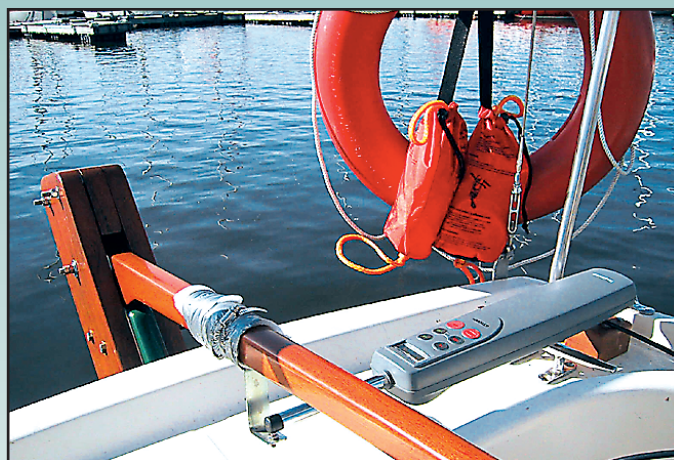
Typical installation for a tiller-mounted autopilot shown on a Contessa 26.
