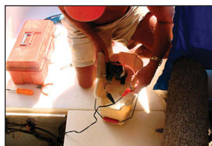
Figure 2 Every three to four months, the macerator pump is removed and cleaned.
