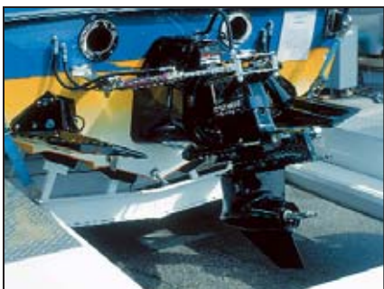
Long narrow tabs used on high-speed powerboats.
