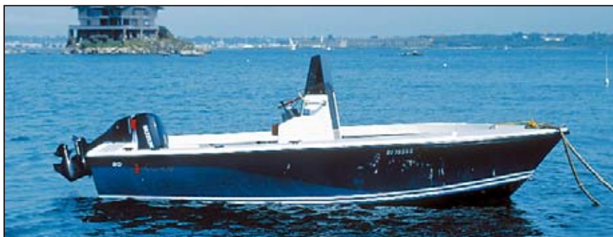
Author's boat floats stern-down, as noted by the white boot stripe, after mounting a heavy four-stroke outboard.
