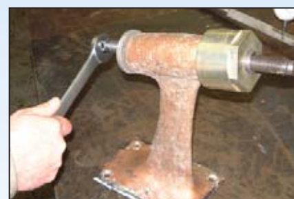
Once a strut has been removed and is on the work bench, a variety of techniques can be used to remove and reinstall the bearing, such as this improvised screw jack for pressing bearings.
