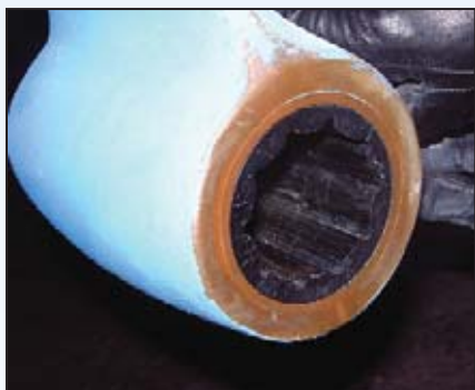
The rubber in this bearing has hardened and cracked throughout. Soon chunks will break off. Best to replace now.
