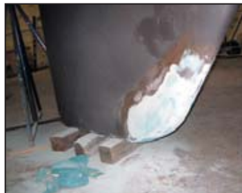
(top) Example of grounding damage to the keel tip; (bottom) Same dents shaped, filled and faired.
