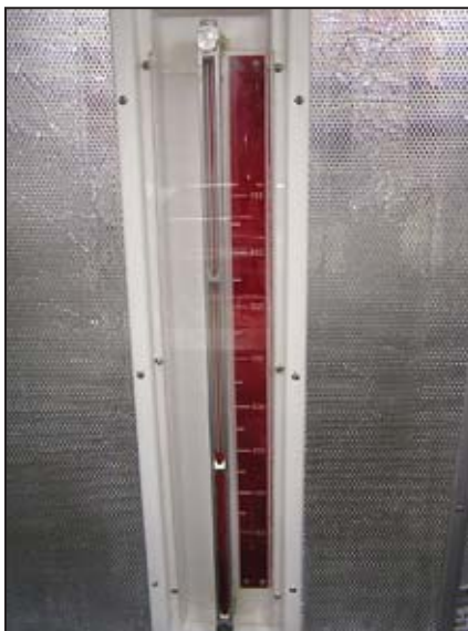
Calibrated sight tube made of standard plumbing fittings and Lexan tubing.
