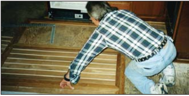
Teak frames, 1" x 5/8" (25mm x 16mm) mounted around the salon perimeter and hatches.
