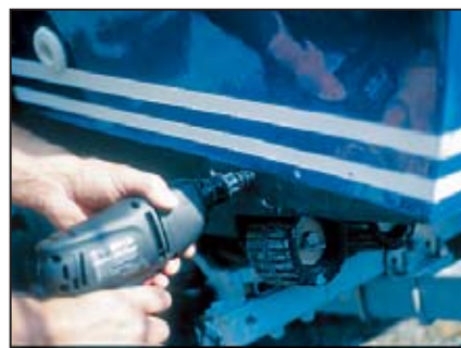
Drilling hole for the hydraulic tubing.
