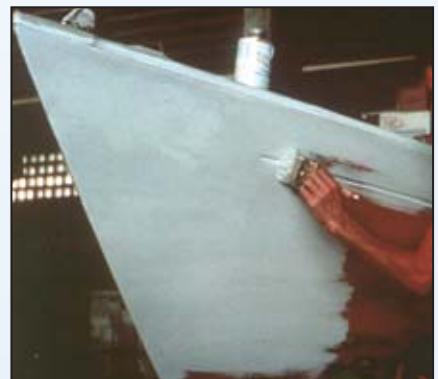
Properly prepped gelcoat receives a coat of primer applied with a natural bristle brush.
