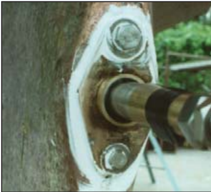
Stern tube configuration with fluted cutlass bearing.
