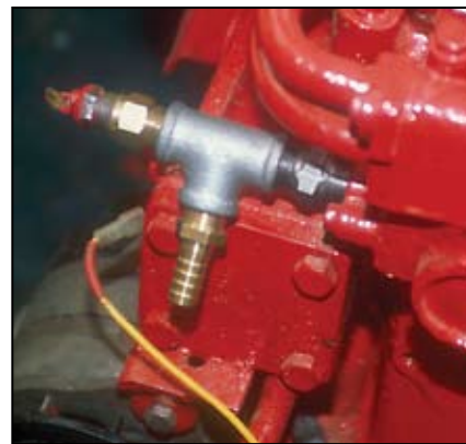
This was the Mark One layout with the sender in the end of fitting, which was later modified.
