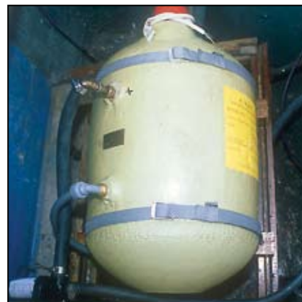
Note the inclined attitude of the water heater to allow the fittings to clear the seat and the final layout of the water outlet from the engine.
