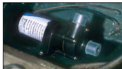
Circulating pump bolts to the bulkhead inside the engine compartment.
