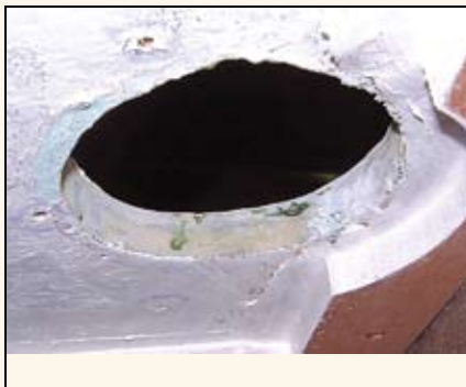
A deck cutout after potting with solid glass.
