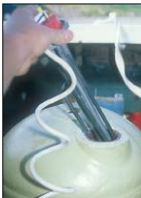
Marine grade double insulated immersion element fits inside tank.
