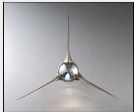
Nearly flat and symmetrical blade profile of this Max-Prop is typical of all feathering props.
