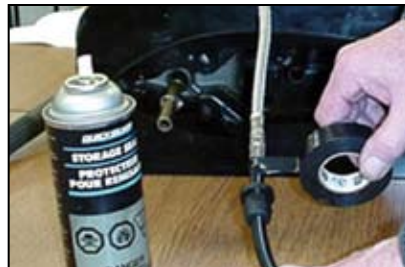
Wrapping electrical tape around the hose simplifies grommet installation.
