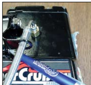
Braided hose retainer mounts to bell housing studs.
