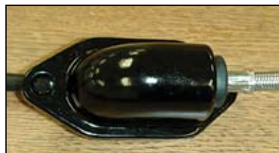
Mount the inlet cover on the transom and then install the grommet.
