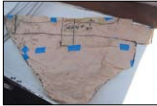
Paper template provides pattern for cutting fiberglass layers: cloth, mat, woven roving, mat and one more layer of cloth.
