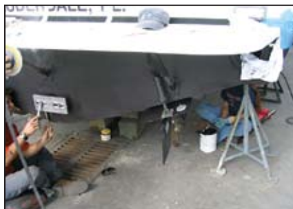
Plenty of helpers expedite the refit: over-size bonding plate is mounted on transom while hull receives new antifouling paint.
