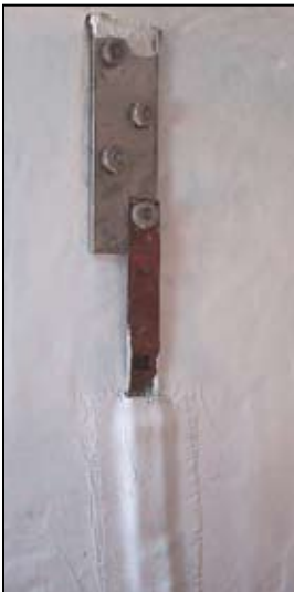
It was necessary to grind out chainplate portion due to too much fiberglass (again!).
