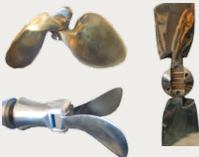
(top left) Martec, the original racer prop. (bottom left) Slipstream has a "bump" stop, which eliminates some of the shock loading on the shaft and clanging sound when blades open. (right) Most of the newer folding props have gears to make sure both blades open.
