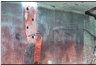
It was necessary to grind out chainplate portion due to too much fiberglass (again!).
