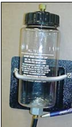
Lube reservoir bottle mounted on bracket.
