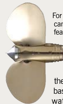
Nearly flat and symmetrical blade profile of this Max-Prop is typical of all feathering props.
