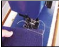
Sewing a dart on back side of cover.
