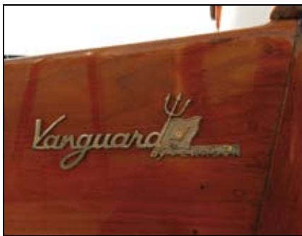
New replica cockpit coaming emblem of cast bronze.
