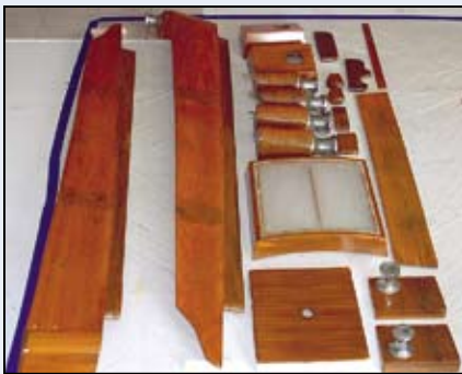
Brightwork was stripped then coated with Cetol Marine Light followed by Cetol Marine Gloss.
