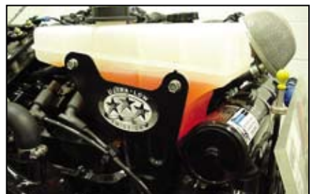
Placement of end cap on closed-cooling heat exchanger.
