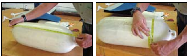
(left) Measuring the barrel length, 24" (61cm) for this fender, and (right) the barrel diameter, which is 27" (68cm).
