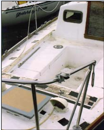
Deck work begins with removal of all hardware.
