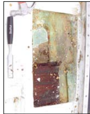
Wet deck repair: (clockwise, top left) Pilot holes drilled in deck to determine extent of wet core. The small area got larger with every drilled hole; Outer skin and core removed from area of core repair; Removing the wet core; New foam board in place with one layer of System Three resin.
