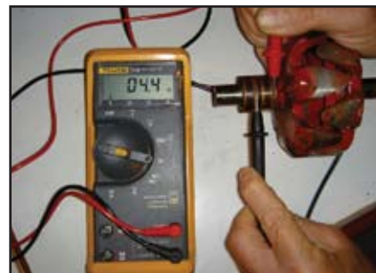
Measuring resistance of rotor with a digital multimeter.
