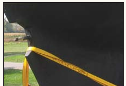
(top) In addition to the fore and aft tie-down straps, a tight ratchet strap to the trailing edge of the keel helps to keep the boat from creeping aft on the trailer. (bottom) On a full-keel boat you'll need to engineer the strap to pass through the propeller aperture.
