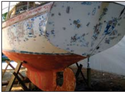
Various states of sanding progress before I applied InterStrip. The gray areas are where all the paint has been removed. Once the paint remover dried, the paint flew off the hull with my sander, saving me hours of work.
