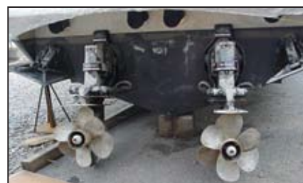
This boat with Bravo 3 drives and timed props maximizes propulsion efficiency.
