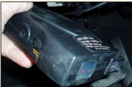
An electric brake controller. Note the brake power adjustment thumbwheel and manual override slide.
