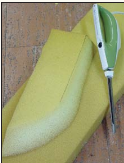
(top) A reciprocating carving knife provides excellent shape control for cutting foam, especially wedge cuts, and (bottom) leaves a smooth, clean edge.
