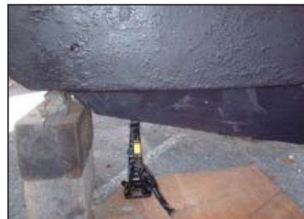
(top) Positioning the board and then climbing into the boat to (middle) winch in the pendant and then back to ground to (bottom) jack up the front end.
