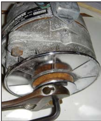
Use an Allen key to remove fan and sheave.
