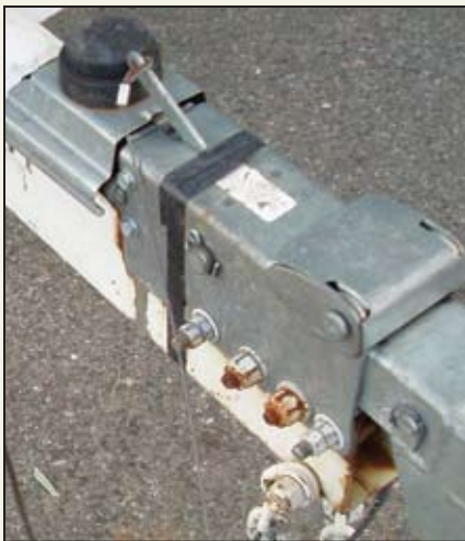
The master cylinder for hydraulic surge brakes is an integral part of the hitch and tongue assembly.
