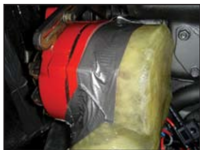
Shroud made of fiberglass cloth and resin and duct tape helps to cool the alternator.
