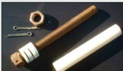
The parts for the custom centerboard pin: Delrin tube and washers, brass rod and nuts and stainless-steel cotter pins.
