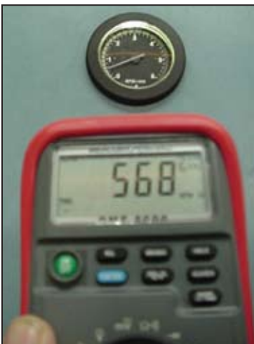
Verifying onboard tach with a shop tach. This particular instrument is a Mercury Marine combined DMT 2000 digital multimeter and tachometer.
