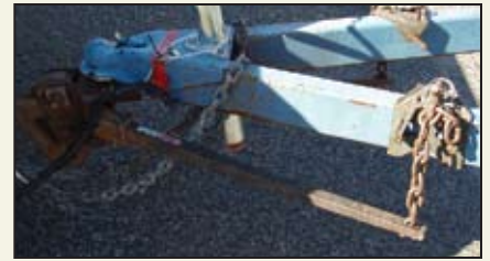
A typical weight-distributing hitch with spring bars. As the bars are tensioned by means of the adjustable chains and lever brackets, the rear of the truck is jacked up. This shifts tongue loads towards the front of the tow vehicle.
