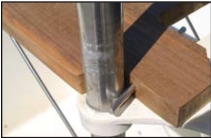
(top) Use extra long bit to drill for holding pins. (bottom) Holding pin positioned in table.
