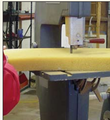
A band saw gives a quick, clean edge. Tilt the table for accurate wedge cuts.
