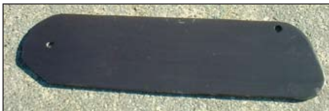
The finished replacement steel centerboard with five coats of Interlux Primocon followed by two coats of bottom paint.
