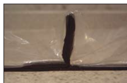
(top to bottom) Any excess bag material requires a pleat; To form a pleat in a vacuum bag apply a short amount of sealing tape to the perimeter tape, inside the pleat, then fold over the top of the short length of sealing tape; seal the bag against the short length of sealing tape, pinching it off at the top; seal the bag against the short length of sealing tape at the bottom corner; finished pleat.
