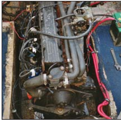
After a steam clean and tune-up and, except for some minor corrosion, the engine ran well.
