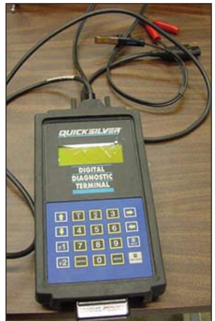
Mechanics use a scan tool to read engine faults in EFI engines.
