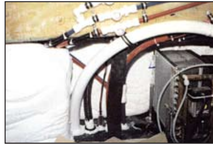
Lightweight 3M Thinsulate is ideal for insulating cabin ceilings.
