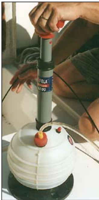
DIY's editor prefers the line of self-contained, hands-free Pela Oil Changer. About 10 or so strokes is all it takes to transfer hot oil into the built-in canister.
