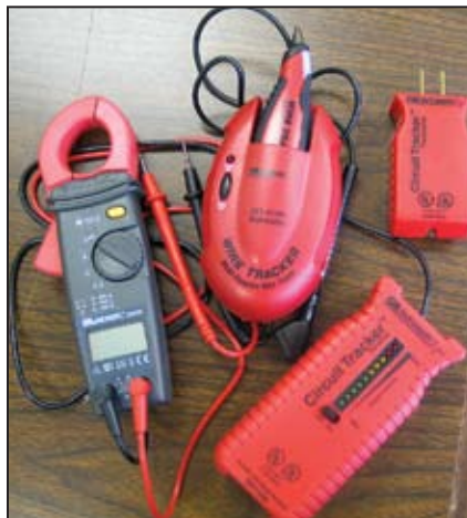
Simple to use tools for measuring current: (left to right) clamp-on meter, and two tone generators, the Wire Tracker and Circuit Tracker.
