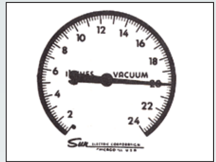
With engine at idle, you can identify possible engine malfunction at a specific vacuum reading. To view a readable pdf of a vacuum-gauge troubleshooting chart, click here .
