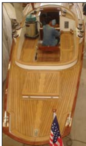
Completed deck prepared with teak sealer is strikingly beautiful.
