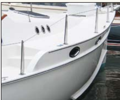
Albeit this trawler has a flared bow, mounting strakes near the waterline further reduce spray.
