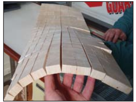
Balsa core sheet. Note system of kerf cuts to allow contoured lay-up.
