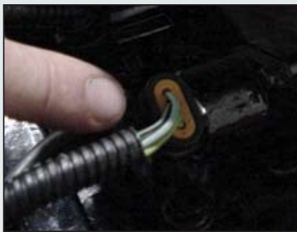
Idle air valve location on a multi-port injected engine.
