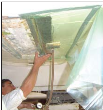
Vacuum bagging achieves better core bonding and resin penetration into the kerf system than hand lay-up but works best with low vapor pressure resins such as epoxy and vinyl ester. The high styrene content of conventional polyester resin can cause problems with bag or infusion vacuum systems.
