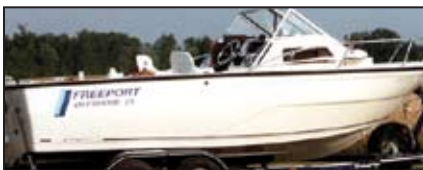
Chine on this boat runs in a straight line from amidships to the transom, a typical shape of a planing boat.
