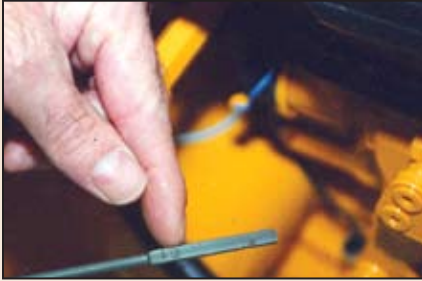
(top) Pour a quantity of oil into the engine crankcase, checking the dipstick as you add more oil. (bottom) Add more as needed until you detect the oil level at the "full" mark, as shown by the top notch on most dipsticks. Don't overfill!
