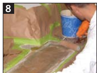
Typical repair sequence: 1 Core problems located by meter and sounding hammer. 2 Wet and delaminated areas cut open so the deteriorating core can be dug out and removed. 3 Old core is now gone and the inner skin cleaned and prep sanded to accept the new core. 4 New replacement core is cut and dry-fitted into place. 5 Next, the new core is bedded onto resin rich glass mat (or specialized core bonding putty). The perimeter gaps and kerf cuts are filled with a mix of chopped fiber and resin or bonding putty. 6 New core bedded and bonded in place and sanded to level, ready for lamination of the new outer skin. Note solid glass potting around the chain-plate. This penetration will never allow leakage into the core again. 7 Hand lay-up of the new outer skin. 8 Repair area is filled and faired, ready for gelcoat or paint application.
