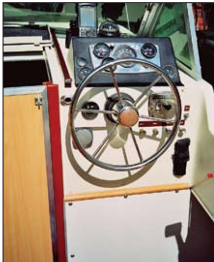
(top) Before: original woodwork and cabin door visible in bottom right foreground. (bottom) After: new cabin door capped with aluminum U-channel. Instrument panel received a coat of satin black paint to reduce glare.
