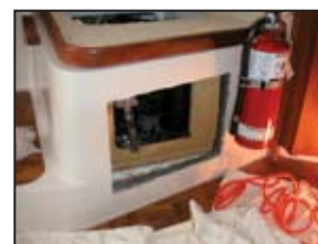
(across) Countertop cutout for larger air intake grill. (middle) Large cutout in front seat bulkhead for the return air grill. (bottom) Cut out in the countertop for one of two supply ducts with the other one installed in the forward cabin.
