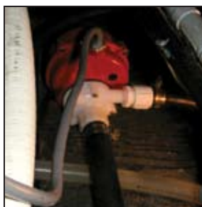
Water strainer mounted outside on the hull conceals the thru-hull.
