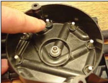
Corroded ignition components, in this case a distributor cap, causes the engine to labor resulting in poor idle quality and engine stalling.
