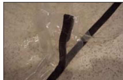
Typical laminate stack: (right to left) mold surface, inner fiberglass skin, foam core, outer skin, peel ply fabric, breather/bleeder layer and clear vacuum bag.
