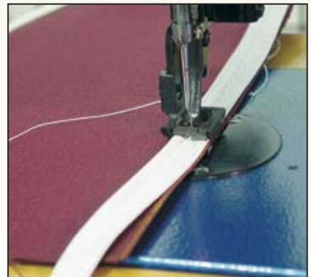
Figure 12 Sewing the welt to the right side of the first plate. By sewing in a clockwise rotation keeps the bulky material to the outside.
