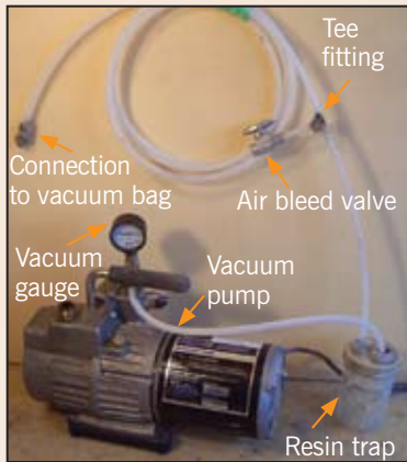
Vacuum pump equipment.
