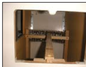
(across) The boatbuilder had roughed in passageways for the ducting. (right) Other areas were less accessible, making it difficult to run ducting in a straight line.
