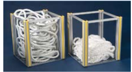
Comparison of 150' (45.7m) of three-strand nylon line (left) to the same length of Yale eight-strand nylon Brait (right).
