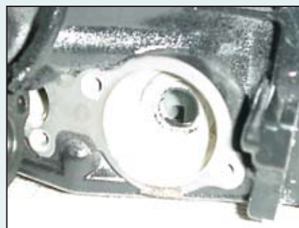
(top) Remove the poppet valve cover and inspect (middle) the cover and (bottom) valve and seat for debris.
