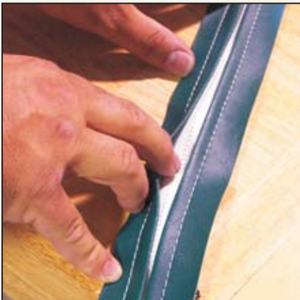
Figure 8 (top) Cutting the temporary seam in the placket. (bottom) The finished zipper placket. Note that the zipper teeth are centered along the seam and covered by material.
