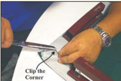
Figure 24 (top) Staplers serve to hold the boxing in place while the corner is pinched to find its center. (bottom) Cutting the corner notch.
