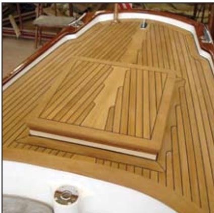
(left) Same diameter teak planks are notched in a matching king plank on the deck hatch. (right) Note plank details around skylight.
