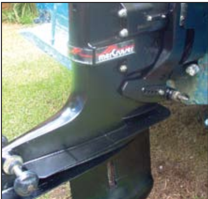
(top) Removing the tarry black mixture on the stern drive proved challenging but, (bottom) after applying primer and paint, it looks like new.
