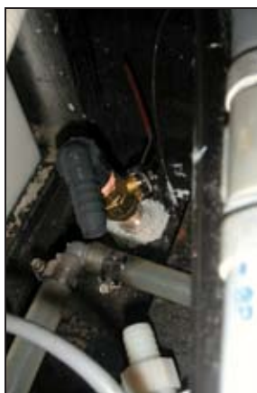
Water strainer mounted outside on the hull conceals the thru-hull.
