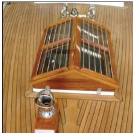
(left) Same diameter teak planks are notched in a matching king plank on the deck hatch. (right) Note plank details around skylight.
