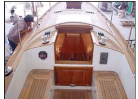
Note covering board and plank layout around cockpit locker hatches, cockpit sole and cabin top.
