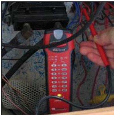
Beeper sounds and continuity light illuminates to show that resistance is low.
