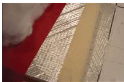
Typical laminate stack: (right to left) mold surface, inner fiberglass skin, foam core, outer skin, peel ply fabric, breather/bleeder layer and clear vacuum bag.
