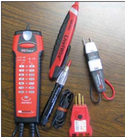
Multimeter substitutes for measuring voltage: (left to right) non-contact Volt Check, non-contact Live-Wire, AC receptacle tester and AC dual lead probe continuity tester.
