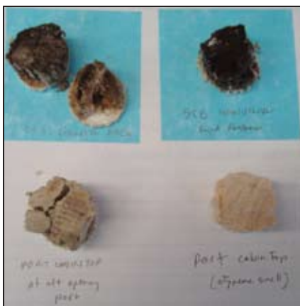
Core samples of balsa at various stages of deterioration. (Clockwise from the lower right): A dry sample in apparently good condition that, nonetheless, produced a high moisture reading due to excessive styrene retained in the core; a wet sample showing only slight darkening still in good mechanical shape; two wet samples showing intermediate deterioration and beginning to crumble; a black, crumbly and dripping wet sample in the last throes of rot.
