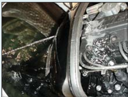
A healthy cooling system telltale water stream.
