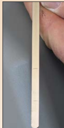
Dipstick removed from engine oil crankcase indicates empty and full levels.
