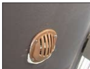
Water strainer mounted outside on the hull conceals the thru-hull.
