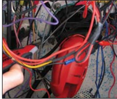
Wire-Tracker transmitter clips to the wire to be traced and a ground, and generates a tone along the wire that is detected by the hand-held receiver's probe.
