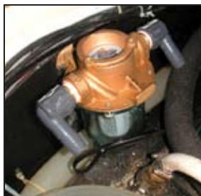
Location of (top) pump in the bilge and (bottom) water strainer on a nearby bulkhead.
