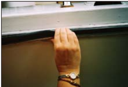
(top) Aged rubrail insert is replaced with (bottom) a black plastic insert that slips in easily after heating with a hair dryer.
