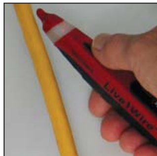
When Live-Wire senses AC voltage in a shorepower cable, the red light glows and speaker chirps.
