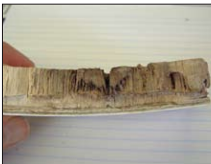
Core samples of balsa at various stages of deterioration. (Clockwise from the lower right): A dry sample in apparently good condition that, nonetheless, produced a high moisture reading due to excessive styrene retained in the core; a wet sample showing only slight darkening still in good mechanical shape; two wet samples showing intermediate deterioration and beginning to crumble; a black, crumbly and dripping wet sample in the last throes of rot.
