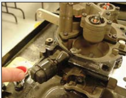
Idle air valve location on throttle-body injected engine.
