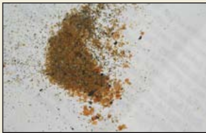
The engine had been missing at high speed and finally wouldn't start at all. The engine-mounted fuel filter was removed and set on a bench to dry out for a few days. This photo shows about 20% of the residue that fell from the filter when tapped on clean white paper. Note the different "stuff" in the filter, mostly bits of fiberglass stained by gasoline along with other contaminants. Clearly the clogged filter caused the engine to be starved for fuel.
