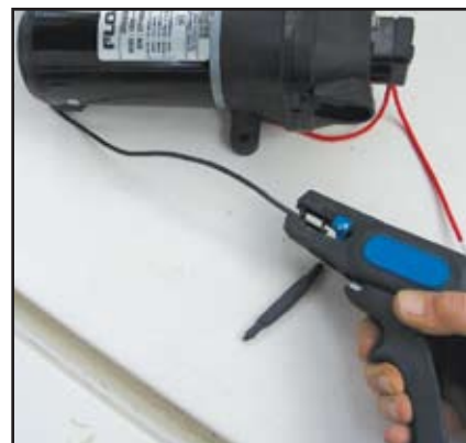
Wire ends are stripped in preparation for remounting pump.
