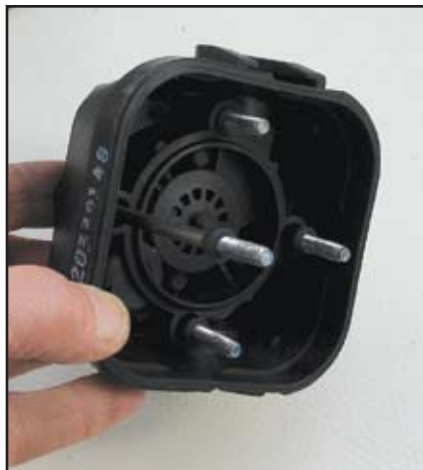
Threading bolts through the housing and rubber ferrules made reassembly easier.
