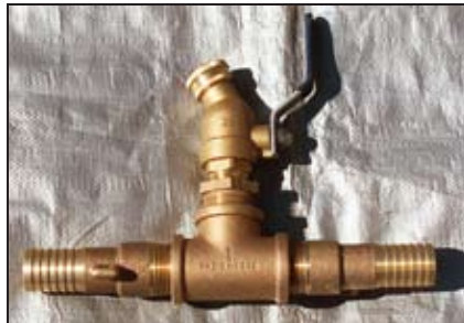
Components and assembled parts for genset and HVAC flushing device.
