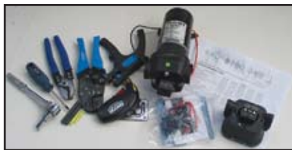
Repairing freeze damage to this washdown pump required about 60 minutes and a few hand tools, a replacement switch and upper housing assembly kit available from the manufacturer.
