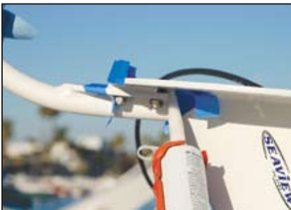
Author caulks around radar cable and GPS pole mount to prevent water intrusion inside the mount or arch. "We get some pretty wet rides on this boat when the seas kick up."
