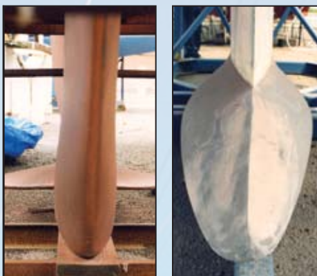
Adding "wings" or a torpedo bulb to the keel bottom is the simplest and lightest method for adding ballast and consequently increasing stability.
