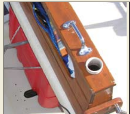
Replacement 7.5 gallon (28L) plastic (not fiberglass) tank and new fuel fittings. Not shown is a canister water separator 22-micron fuel filter installed on the transom, which is now used in addition to the filter mounted on the engine.
