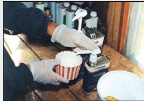
Dispensing pumps measure the correct ratio of resin to hardener to ensure a proper mix.
