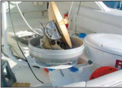
M3 and scanner are attached to the Seaview mount before hoisting onto the arch.
