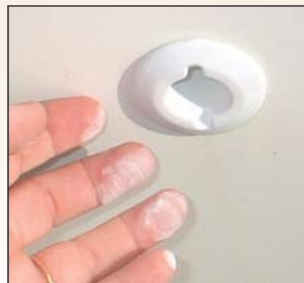
Chalky residue indicates UV attack and breakdown of inferior plastic thru-hull.
