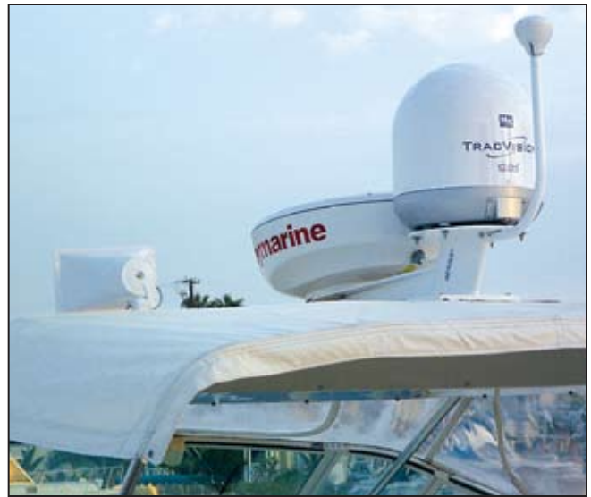
Job completed! The hailer is mounted on one side and the VHF on the other side.
