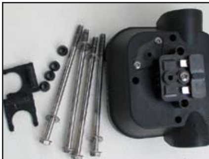
Included in the upper housing kit are replacement check valves, ferrules, hex bolts, sealing discs and port clips not required for this repair but good to keep in your spares kit.
