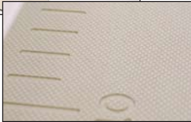
(above) Cockpit floor hatches made of StarBoard AB offer a high-friction slip-resistant surface. (right) Dot pattern on the finished side. Note accent grooves cut with a router.
