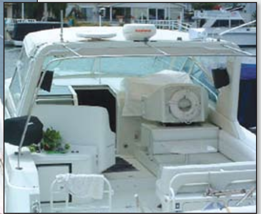
Original radar arch. Note positioning of equipment. As part of the refit, the author relocated all gear to improve aesthetics and performance.
