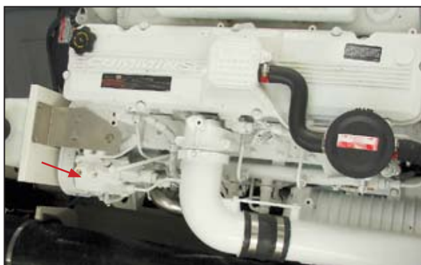
Cummins OSC series 500-hp six-cylinder shows injection pump (see arrow) with fuel lines to a fuel rail that feeds fuel to the individual injectors that act independently. On smaller engines, the injector lines run directly from the pump to the cylinders.
