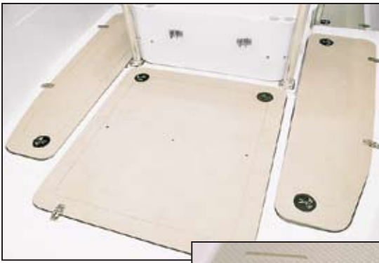
(above) Cockpit floor hatches made of StarBoard AB offer a high-friction slip-resistant surface. (right) Dot pattern on the finished side. Note accent grooves cut with a router.
