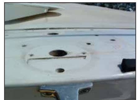
Marking the footprint of the new mount on arch top seemed like a good place to start this project.
