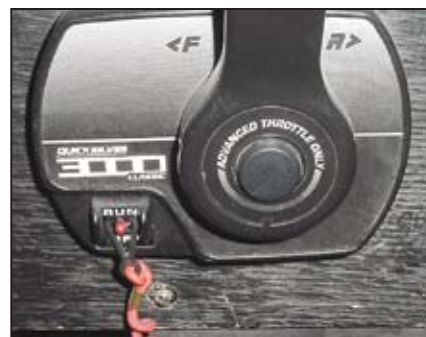
Safety lanyard and engine shutdown control switch mounted near the helm station.
