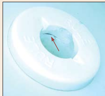
The perfect example of a failed plastic thru-hull fitting (note the crack). It will eventually break off at the inside nut causing the bilge pump discharge to flow back into the bilge.
