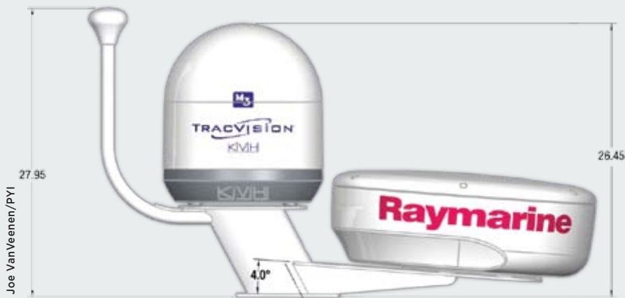
Seaview Dual Mount with custom modifications engineered by PYI to keep the profile as low as possible and shrink the total height from 35" to 27.95" (889mm to 709mm).
