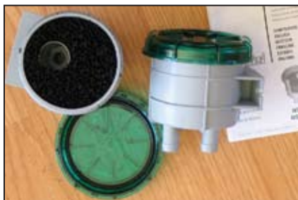
Vetus No-Smell filters contain an odor-absorbing material and mount in-line in the waste holding tank vent hose.
