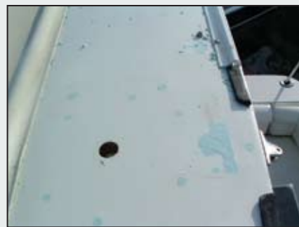
After filling two-thirds full of epoxy resin, the perimeter of each hole was beveled using a Dremel then filled with 3M Marine Premium Filler.
