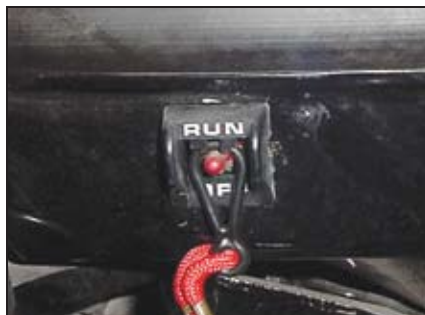
Most tiller-steered outboards built since the mid-80s are equipped with a “kill” switch either on the engine front panel (left) or on the cowl (right).
