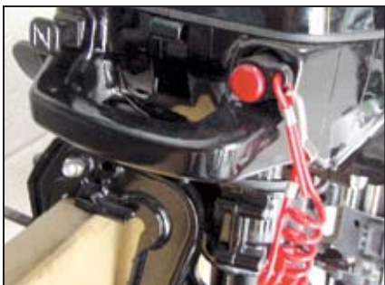
Most tiller-steered outboards built since the mid-80s are equipped with a “kill” switch either on the engine front panel (left) or on the cowl (right).
