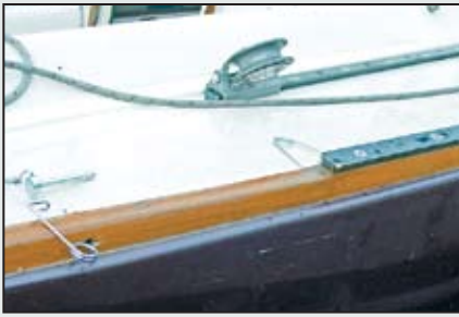
Drain holes with two types of locking pins demonstrated.
