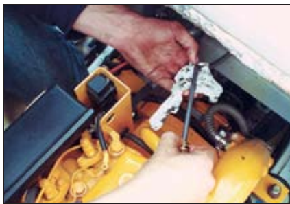
Black oil identifies the residue remaining from out-the-dipstick oil changes.
