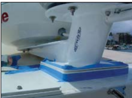
(top) Fitting predrilled StarBoard wedges. (middle) Drilling mounting holes in arch for the Dual Mount. (bottom) Taping edges before caulking saves on cleanup.
