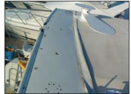
Removing old equipment left 43 holes to fill. Shown on the bimini is the new Seaview Dual Mount.
