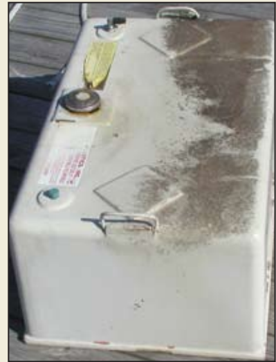
(top left) Close up of damaged fiberglass fuel tank (right) after using 10% ethanol for just four months. This tank was made by Pate Plastics and installed four years ago under the center console seat on a Boston Whaler 17' (5m) Montauk. Fuel was slowly seeping out onto the deck where it became obvious to the owner that something was amiss. (bottom left) The other side of the same tank had not yet been penetrated (paint was chipped away to check for damage). A big sticker on the tank stated: "Do not use for alcohol."
