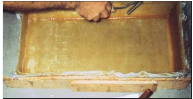
It's important to roll all the air out to achieve a smooth laminate. Two layers each of 1-1/2oz mat and 24oz biaxial roving, rolling quickly between layers, followed the skin coat. Once cured, two additional layers were applied. Checking the thickness with a calliper, additional layers were then added to achieve a 3/8" (9mm) laminate.
