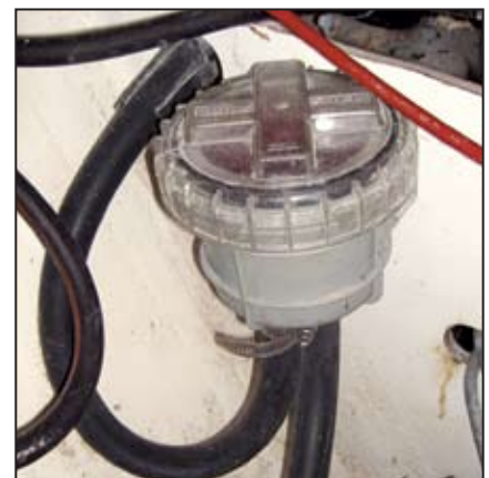
Vetus sea strainer on raw-water intake mounts to bulkhead.
