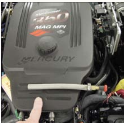
Manometer hose attached to air intake system inside engine compartment.
