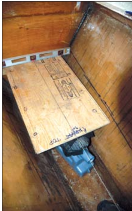
(left) Checking shaft position with laser level. (right) Engine mockup in position to locate engine beds. On this engine, the mid-point of the adjustable engine mounts lined up almost exactly with the gearbox output flange. If they were lower, we would have had to make a wooden support at each end of the plywood to position the reference wire.
