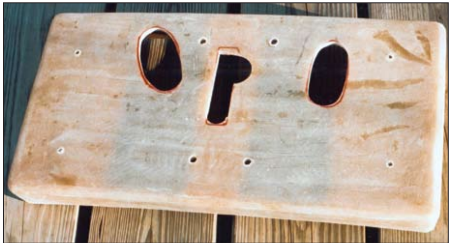
Modeling clay is scraped off and the residue cleaned with acetone and then edges are trimmed with a hacksaw and mini-grinder. For extra stiffness, without significantly increasing thickness, two strips, six layers each of carbon fiber (visible in black), are added at the bolt locations before the final layer of mat. Hawseholes and the motor installation hole in the center are marked using the old backing plate as a template and then cut out with a holesaw and jigsaw. As the box fits neatly between the deck beams, the fore and aft flanges are cut to the same depth as the beams. Finishing the box inside with a one-part polyurethane paint is optional.
