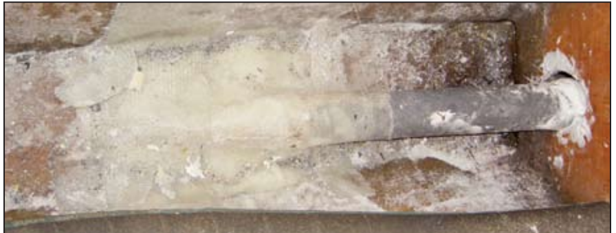
(left) Overlength stern tube ready for epoxy putty and fiberglassing. (right) Trimmed stern tube. (bottom) Stern tube fiberglassed in place on inside.
