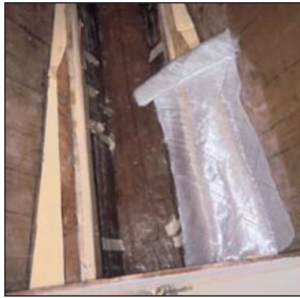
(left) Measuring fiberglass to cover the engine beds. (right) Applying peel ply to the fiberglass to leave a smooth appearance.
