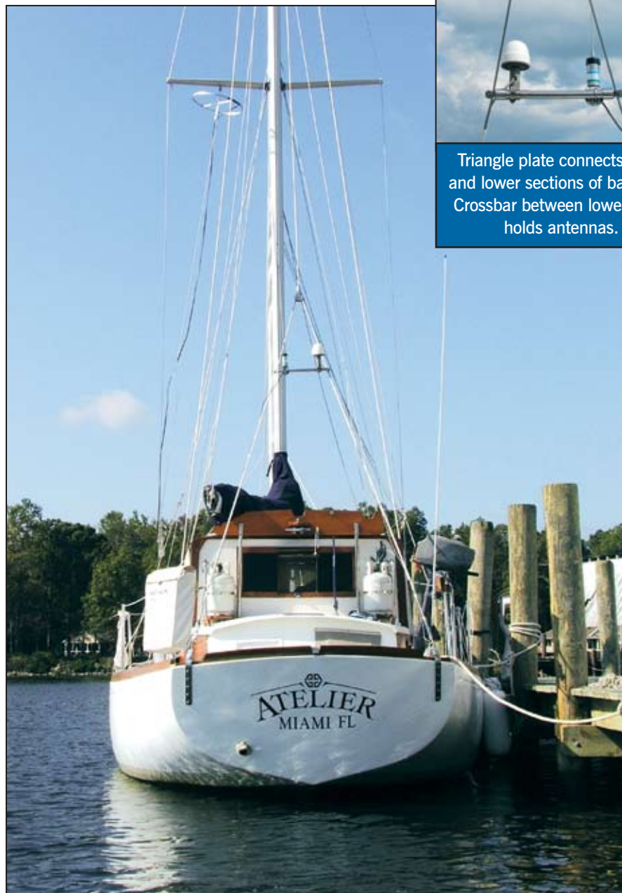
Overview of new split backstay assembly. New chainplates attach to the transom and are bent to match the angle of the new stay. Note stern light and cleat for dinghy line on boom gallows.
