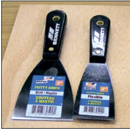
Putty knives come in various grades. Choose a flexible one for scraping plywood and round the corners with sandpaper or a grinder so you don't inadvertently gouge the wood.
