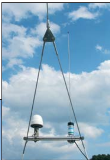
Triangle plate connects upper and lower sections of backstay. Crossbar between lower stays holds antennas.
