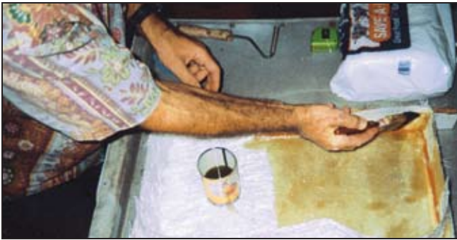
For a small part like this, a brush gets the resin into corners better than a felt roller. Wetting the mat adequately and evenly is essential to achieve a smooth and solid laminate. The polyester resin should be catalyzed at about 5cc to 10cc per quart at room temperature. Be sure to use unwaxed resin.
