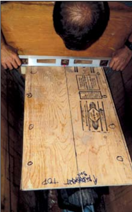
(left) Checking shaft position with laser level. (right) Engine mockup in position to locate engine beds. On this engine, the mid-point of the adjustable engine mounts lined up almost exactly with the gearbox output flange. If they were lower, we would have had to make a wooden support at each end of the plywood to position the reference wire.
