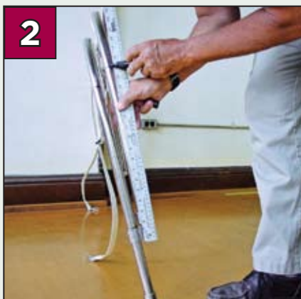
Marking for the second rail.
