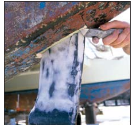
Trimming excess foam shims at the carbon fiber cutlass bearing strut prior to shaping fairing compound.
