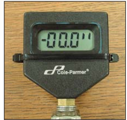
Pass: Manometer showing no engine compartment vacuum at wide open throttle with engine compartment sealed.
