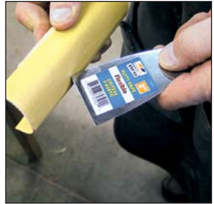
Putty knives come in various grades. Choose a flexible one for scraping plywood and round the corners with sandpaper or a grinder so you don't inadvertently gouge the wood.
