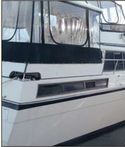
Air intakes enable air exchanges that deliver fresh air and dilute heat buildup within the engine compartment
