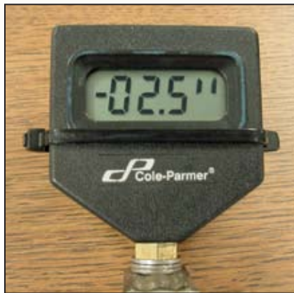
Fail: Manometer showing 2.5" (63mm) of vacuum at wide open throttle with engine compartment closed. This boat needs more air vents and the engine will be down on power and could vapor lock.
