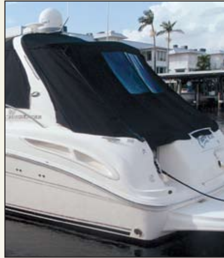
Air intakes enable air exchanges that deliver fresh air and dilute heat buildup within the engine compartment
