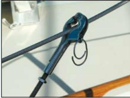
What's wrong with this picture? A high-quality pelican hook is compromised by a split ring that is easily snagged by a sail sheet or crew clothing, resulting in unintentional opening of the latch. The tension adjustment nut is not threaded tight to the fitting.
