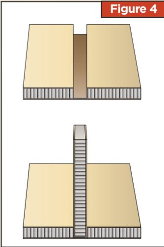
Method 1 for creating a "T" joint: Dado a recess through one skin and the core, leaving the other skin uncut. Glue the end of the joining panel into the recess using thickened epoxy.
