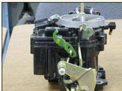
Green arm is the adjustable accelerator pump on a two-barrel carburetor.
