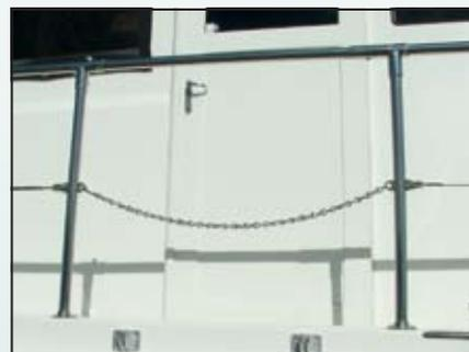
The upper rail gate is secured with a latch activated by a small knob that permits the rail to lift vertically and fold over, via a hinge, onto the fixed section. It’s a good arrangement but the light chain at the lower lifeline would not survive the load test.
