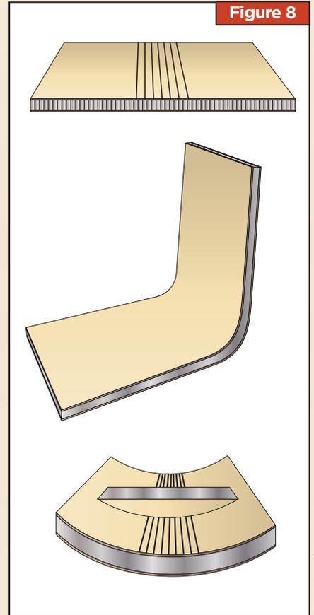
To create a rounded corner, kerfs (slots) are cut through the back face and core that allow the panel to be folded and bonded to make the curvature permanent. A reinforcing gusset bonded to the backside of the curved panel is optional but adds strength.
