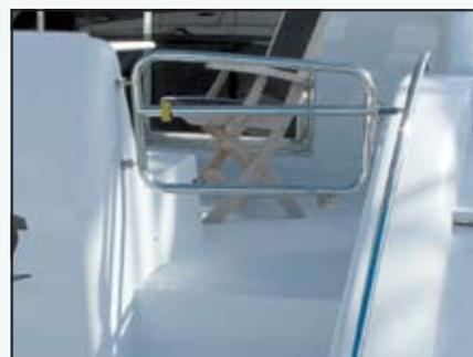
A simple, effective gate that opens inward is much safer than an outward opening gate or transom door that can dump into the sea the unwary leaning on a gate/door that is not securely latched.
