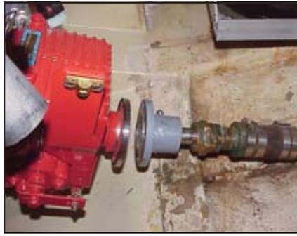
Coupling clearance is critical to ensuring the correct engine alignment. Shown is a R & D Marine flexible shaft coupling supplied with the engine.
