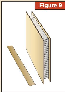
Removal of the core from the panel edge to provide clearance for a spline, joint or edge finishing trim is done with either a table saw using a straight blade or a dado set to the core width or with a router. The trim is then bonded to the edge.
