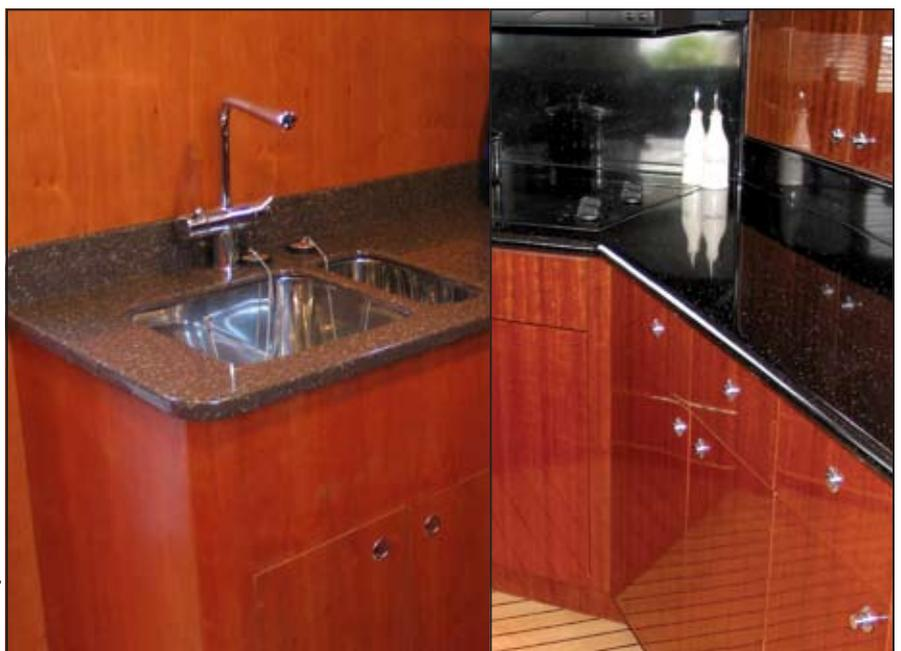
Countertops installed in many top-end yachts are actually lightweight cored panels.
