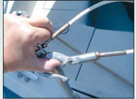
Swage at the lifeline (shown by the arrow) gate wire is cracked. The good design and condition of the pelican hook will not save this gate when the swage fails and the gate opens under load.
