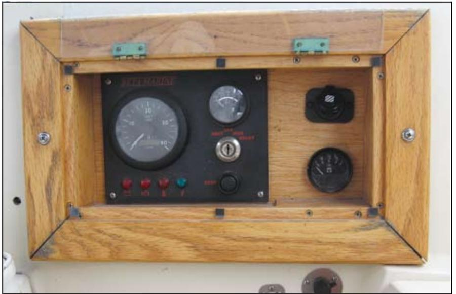
New engine control panel has tachometer with hour meter, key start, push button stop, warning lights and audible alarm for low oil pressure, high temperature and alternator not charging, and optional temperature gauge.
