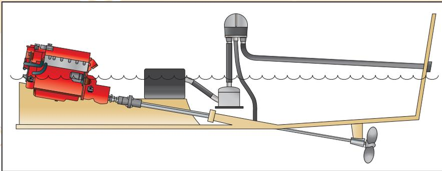
An HMI exhaust water separator replaces the gooseneck and removes the cooling water, draining it below the waterline thus minimizing backpressure. Ideal for gen-sets, by eliminating the splashing noise out of the exhaust, it reduces noise up to 90%.
