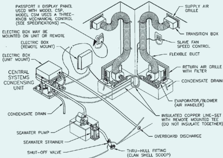
Components of a central air-conditioning system.
