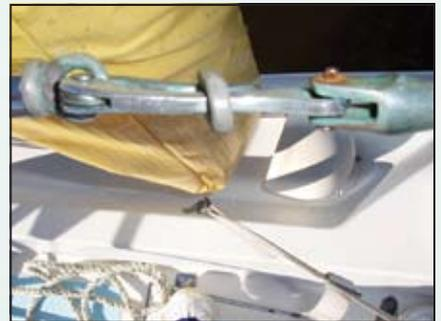
A well-designed gate terminal arrangement with a fairly goof-proof pelican hook if it stays connected to the toggle. Clevis pin in toggle is missing the cotter pin to secure its position as the key connection to the toggle.
