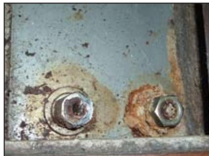
Shaft strut mounting bolts in a trawler yacht built in Taiwan. The bolts are wasting away inside the nuts. Later, the bolts were removed and found to have dissolved to half their original diameter. Zincs were totally wasted and the bolts were sacrificed to the cause.
