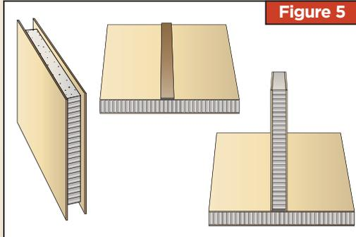
Method 2 for a "T" joint: Glue a wood spline to the surface of one piece and then remove the core from the adjoining piece to create a recessed edge, apply thickened epoxy to the recessed edge and then fit the recessed edge of the spline and clamp.
