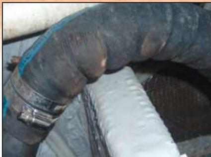
Easily identifiable problem hose that is suffering from extreme bend radius sickness. In many cases, this kind of hose damage is not visible since the inside radius is not readily visible. You'll need a lighted mirror for the inch-by-inch inspection of the underside of hoses and clamps.
