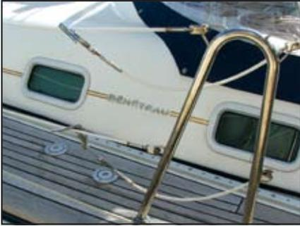
“Old reliable” lifeline gate design with upper and lower, vinyl-coated wire lifelines and gates fitted with pelican hooks. As long as this system is maintained, it should do its duty. Rust is the biggest enemy of coated lifelines and uncoated wire, which doesn't suffer hidden corrosion issues, is a better choice.
