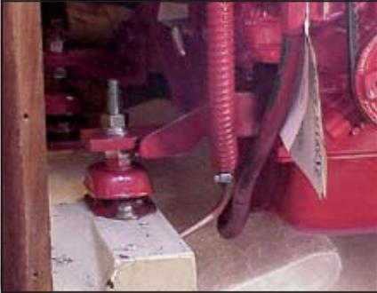
(Top) Chain hoist takes the engine weight until completing engine alignment. (bottom) Adjustable, customized mounts simplify engine alignment.
