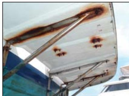
Localized corrosion of swim platform supports and fasteners is an example of the boat builder's choice of stainless steel that is not suited to this application, which exposes the metals to constant immersion in seawater.
