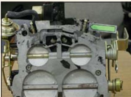
Idle mixture screws on a four-barrel carb.
