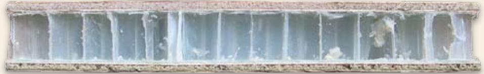
Where cost is no object, aircraft industry honeycomb cored panels, using many of the core materials mentioned above as well as polycarbonate thermoplastic, stainless steel and carbon fiber, are available from Hexcel, M.C. Gill and Cattco, to name just a few.
