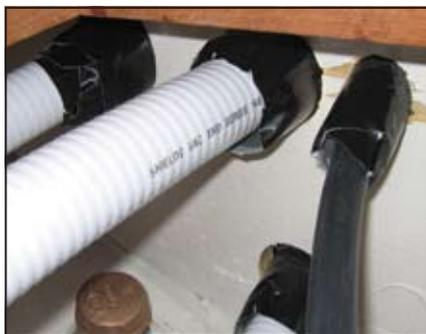
Chafe protection, namely Gorilla Tape, is installed around sanitation hoses where they pass through the locker divider.
