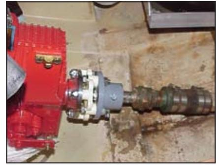
and bought new stainless-steel bolts for mounting. With the mounts secure, we rechecked the clearances and completed the coupling installation.
