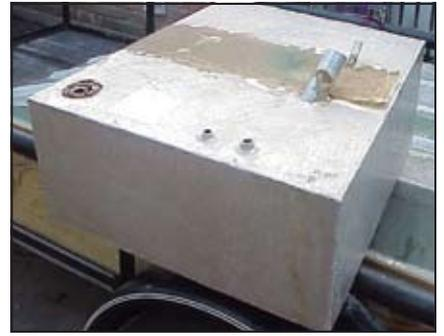
Cleaned fuel tank gets a return fuel connection and shut-off valve.
