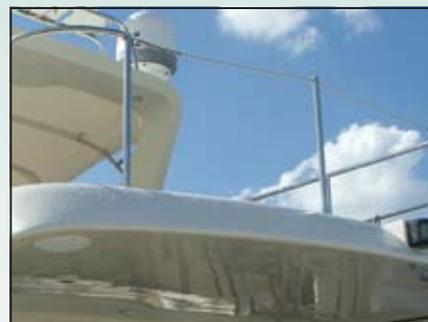
This gate is provided to allow the launching of a dinghy from the upper deck. The gate is opened and the intermediate stanchion removed temporarily during dinghy lifting and launching operations.
