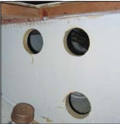
Locker dividers were installed to make the lockers more functional and add strength to this area of the hull and settee. Holes were then drilled for hoses and cables.
