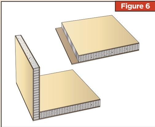
To make a corner joint, remove a section of skin and core to create a rabbet and glue the end of the joining panel in place over the exposed rabbet.
