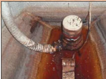
Multiple waterlines in this bilge tell a story of several bouts with high bilge water levels. Worse news is found in the fuel-laced bilgewater. A boat owner or buyer cannot ignore the obvious evidence of fuel and water leaks.
