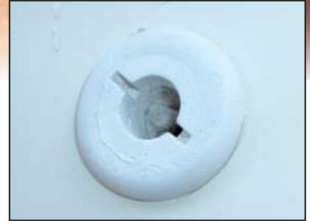
Degraded plastic thru-hulls are something easily seen, even by the casual observer. Non-fiberglass reinforced plastic fittings were common in older boats. Today's boatbuilders use reliable and durable reinforced plastics like Marelon with confidence in their performance above and below the waterline.
