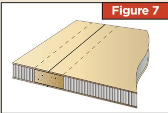
Joining two panels end-for-end is done with an overlapping wood spline, epoxied in place of the core along the joining edge and clamped.
