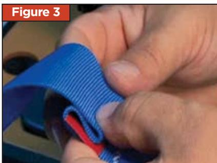
Figure 3 Inserting a flag to show overload.
