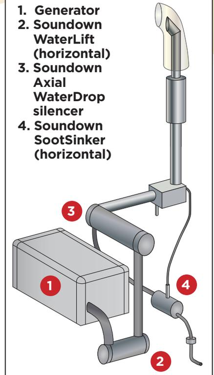
A typical dry exhaust system sends exhaust gases aloft. This eliminates exhaust fumes, reduces sooting on the hull and provides quiet, splash-free operation.
