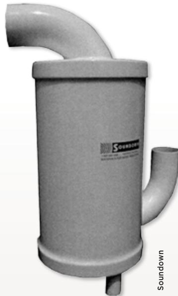
Made of composite fiberglass, Soundown's Classic WaterDrop silencer discharges the cooled, dried exhaust gas from the silencer side housing and the raw water to a thru-hull fitting below. Extremely quiet, separating the gas and water silences the engine's combustion noise and creates minimal backpressure.
