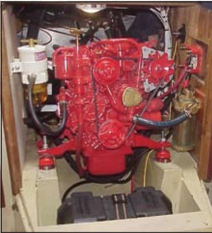
Job completed. Note the top-load fuel filter and water strainer.
