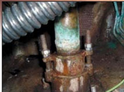
“Out of sight, out of mind.” One of a pair of rudder bearing/stuffing boxes on a 41' (12.5m) motoryacht. Notice adjusting bolt at left is bent from persistent attempts to control leakage. Water was flowing from these fittings and the owner could not find the source. Visual access was difficult enough. Physical access for service requires orangutanian flexibility.
