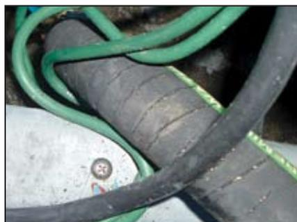
Cracks in outer ply of hose compound are external symptoms that the hose is degrading. The real story is unfolding within the inner plies. When will it fail? Replace now. Ask the question later.
