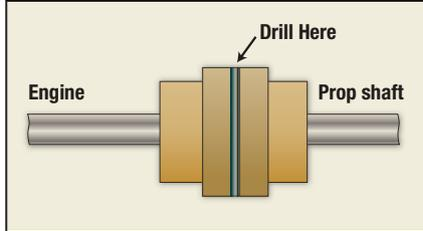
Drilling multiple holes (visible in the top photo) freed the corroded shaft coupling from the engine.
