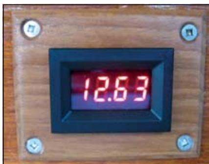
New digital meter installed. The photo of the analog gauge was taken just before installing the new meter so both meters read the same actual voltage. Certainly, it's easier to know the true voltage with the digital one.
