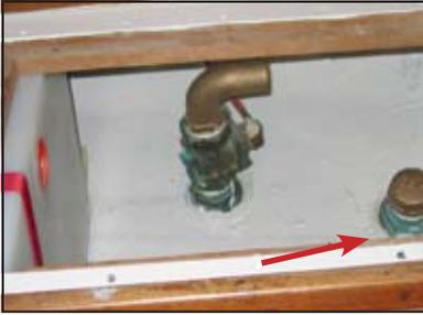
Overboard discharge thru-hull is capped off, as discharge is not an option when cruising in freshwater.
