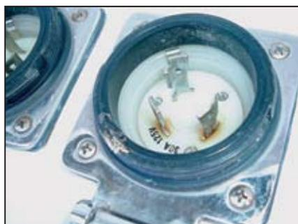
Corrosion makes for a high-resistance connection that can cause overheating and start a fire.
