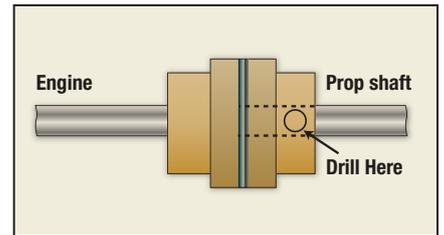
Drill slightly through set screw hole into shaft to allow set screw to bite into the shaft.
