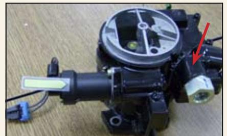
Modern turn key start carburetor doesn't require a choke plate due to its fuel enricher system (shown by yellow arrow). Red arrow points to the fuel filter on this two-barrel carb.
