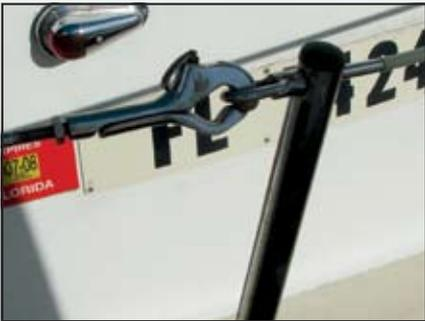
This pelican hook arrangement on a sailboat lifeline gate has stood the test of time as a good design, well installed.
