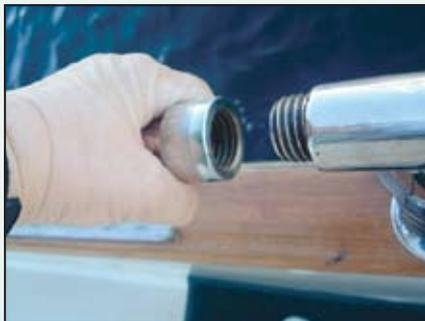
The section of railing in hand slides out of the fixed tubing of one end of the railing and has a nut that threads on to the other end, which is threaded to accept the nut. The resulting closure is effectively bolting the gate closed.
