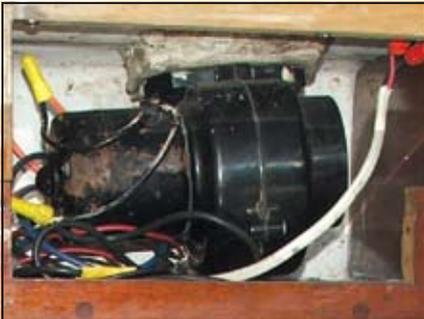
The idea for the galley blower in DIY Projects column in the DIY 2007-#3 issue is a good one but the picture on page 53 captioned: "Blower installed in shelf area above stove. Metal screen filter covers the blower compartment;" shows wire nuts used in this installation. The use of wire nuts is prohibited by the USCG and isn't approved by ABYC for marine use. Editorial review of the illustrations as well as text by a real expert would make your publication a first-class tool for boaters.
