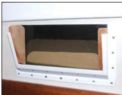
To close the port, the Lexan panel replaces the screen, held in place against the interior surface of the cabin by the wooden wedges.
