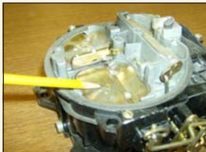
Secondary air valve on a Rochester four-barrel carb opens the adjustable rpm.
