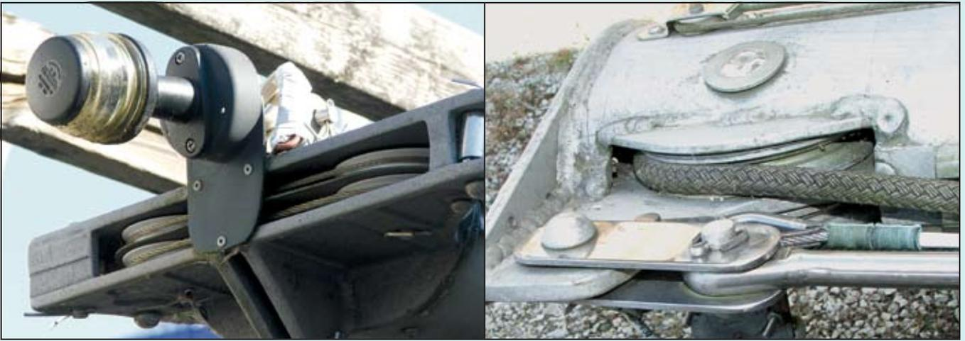
With so many different masthead configurations, replacing the masthead sheave may not be easy, particularly on an older boat. (left) All-wire sheaves. (right) Stepped-down sheave for wire and rope.
