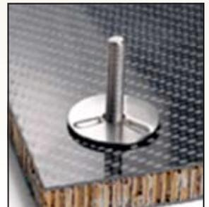
The new TwinDisk from EFC International provides a rapid fastening point anywhere in a composite panel. A hole drilled in the panel removes the core, adhesive is applied and TwinDisk pushed into the cavity. The bottom disk bonds to the bottom skin, the top disk to the top skin, to form a secure fastening mount.
