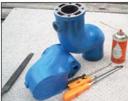
(left) A filed riser surface. (right) Various screwdrivers used to separate the elbow from the exhaust hose, the file used to flatten the machined surfaces and Aero Kroil penetrating oil.
