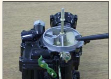
Choke plate closed on a modern two barrel carb.
