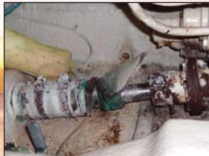
The shaft rotation has been slinging water and spray has rusted stuffing box hose clamps and coupling. Even the cleverly devised shield cannot deny an excessive leak at the shaft stuffing box. The leak will soon become uncontrollable and possibly sink the boat. BoatU.S. Insurance does cover a sinking related to conditions like this.
