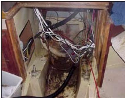
(top) Original 30-year-old Atomic 4 was inoperable. (middle) Removing the old engine with a chain hoist suspended from a metal bar across the main hatch. (bottom) A mess of wiring and hoses and years of dirt.
