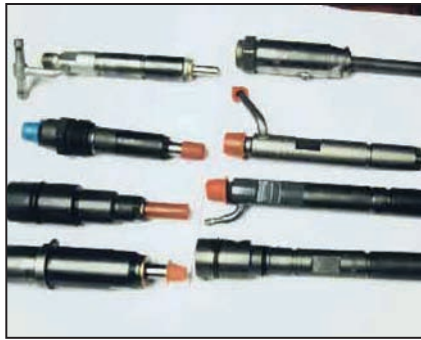
Various injectors all have one thing in common: they require servicing at specified intervals. Red plastic caps protect injector nozzles.
