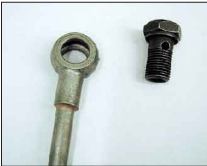
Fuel return line with hollow bolt.
