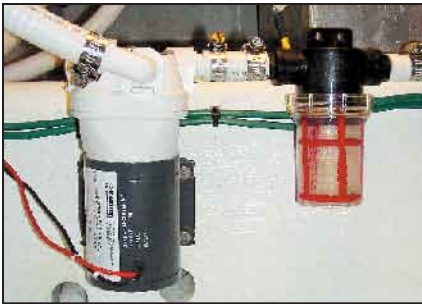
Inline strainer mounts to valve and connects to the seawater pump.
