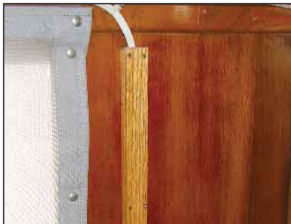
Use a wood channel to cover the solar panel wire where it passes through the wheelhouse.
