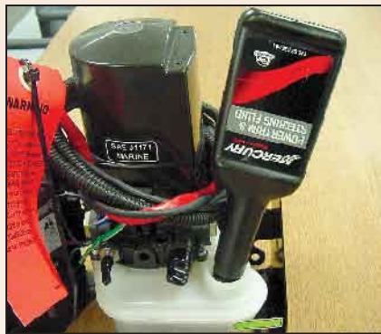
Some oils are specific to the application. Never mix oils or you could contaminate the original lubricant. Green arrow shows the full mark on the trim pump.
