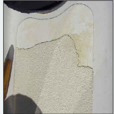
On this boat, the areas originally covered with non-skid are molded in as raised platforms. This made the taping and sanding easier.
