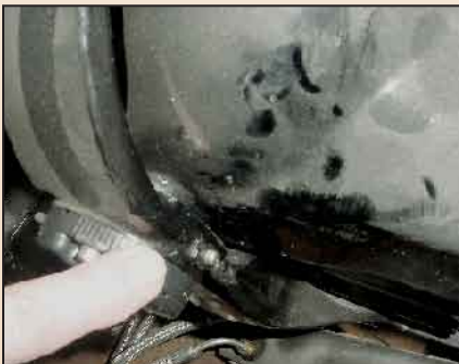
One of two hinge pin grease fittings located on an older (1990) Alpha drive gimbal ring. Note the protective cap.
