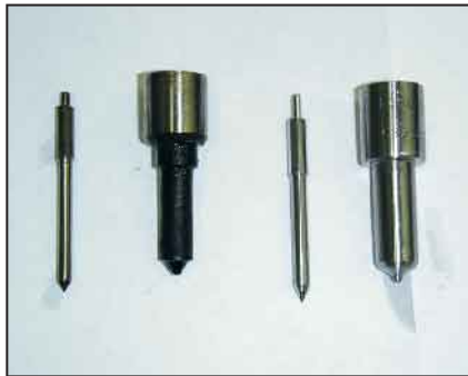
Clean (right) and fouled injector nozzles and tips.
