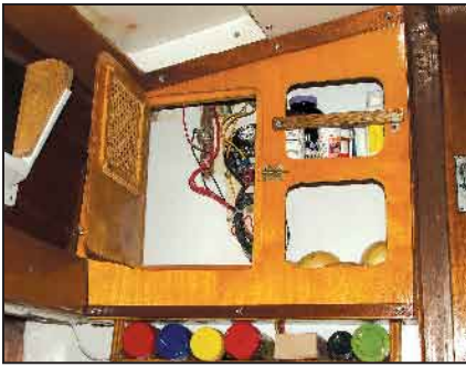
A custom-built cabinet provides storage for small items as it hides and protects the backside of the depth sounder and other instruments.
