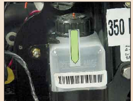
Green arrow shows the full mark on the gear-lube reservoir.
