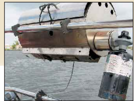
Grill leaning badly. Notice the bend in the support rod.
