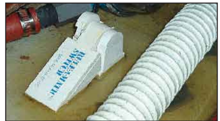
(Top) The popular ITT Rule Super Switch and Rule-A-Matic mechanical float switches. (Bottom) Older models like these contain mercury and should be properly disposed of when replaced.
