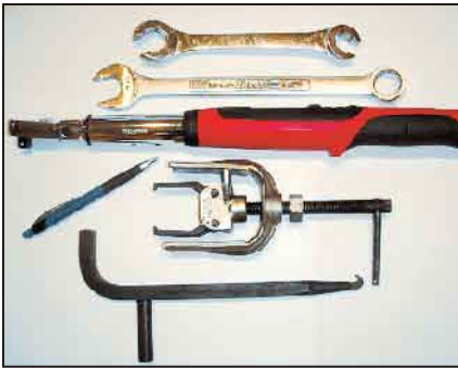
Injector service tools: (top to bottom) line wrench; conventional wrench (do not use); torque wrench; and injector puller.
