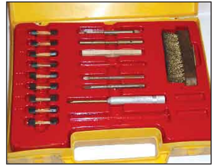
For those times when you cannot access a service shop carry an injector cleaning kit to clean small engine injectors.
