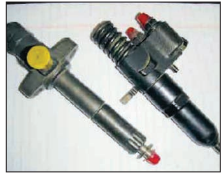
Two injector types, internal and external spring. Injector on right has its own throttle rack.
