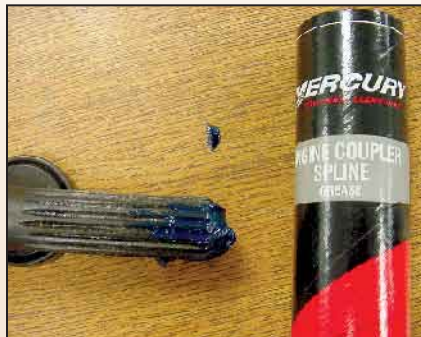
Engine couplers and the shaft splines require a special high-pressure grease.
