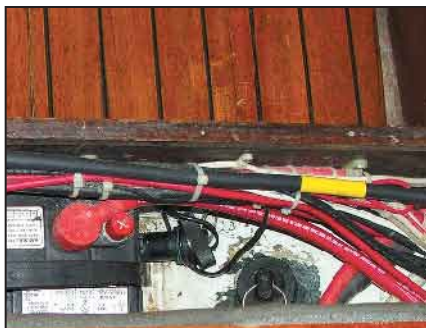
Use cable ties to bundle wires and to keep them safely in place.
