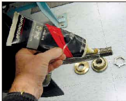
Lubricate propshaft splines once a year and always torque on the prop nut.
