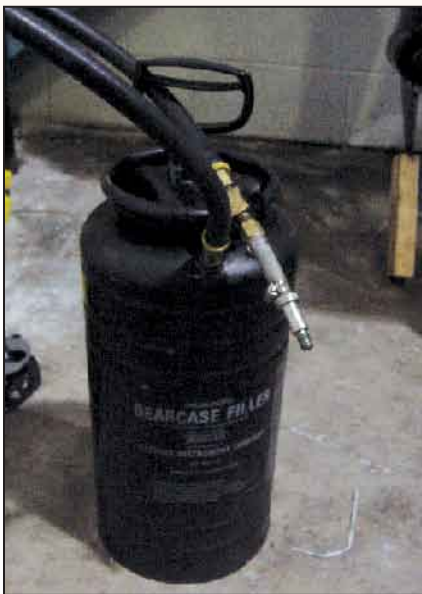
(top) This hand pump greatly simplifies refilling the drive oil. The pump connects to a 1 quart (946ml) gearlube bottle and the hose end screws into the fill hole on the drive. (bottom) The pros use a Stevens Equipment gearcase filler model S-33 to change gear oil.
