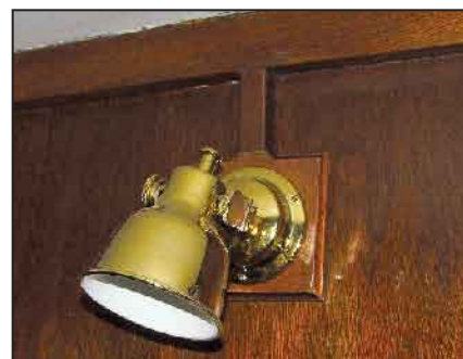
Wooden channels hide the wire leading to a cabin light.
