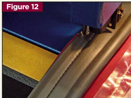
Foam is sewn in place with a single row of stitches. With a walking foot machine, the foam is sewn on top like this; normally, it is sewn with the less sticky fabric on top.
