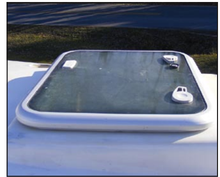
After painting the cabin top, the hatch was bolted in place.
