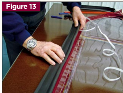
Baste the weather-stripping foam in place.
