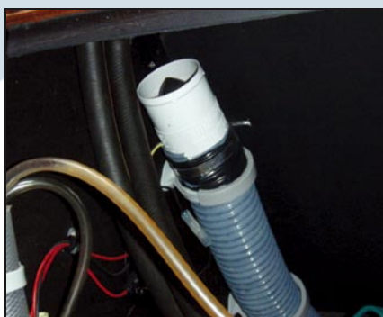
Bilge blower (left) mounted very high in the engine compartment is routed low into the bilge (middle) then to the transom where it was not attached to the exhaust vent (right). The engine smoked badly, ran warm and aged very quickly in less than 100 hours as a result of practically no ventilation made more deadly by a nearly airtight engine box. This was a factory installation on a new vessel from a very respected builder. Being new or used does not ensure a proper ventilation system.
