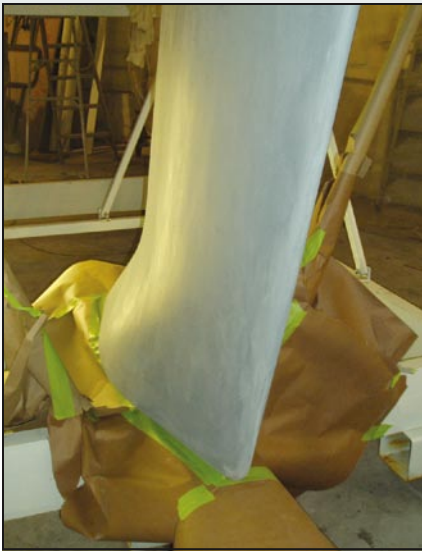
(left) A Beneteau 36.7 keel barrier coated at the factory, faired, epoxy primed, sanded and ready for the application of racing antifouling. (above) A C&C 27 keel ready for combat after many hours of prep.
