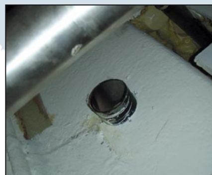
Bilge blower (left) mounted very high in the engine compartment is routed low into the bilge (middle) then to the transom where it was not attached to the exhaust vent (right). The engine smoked badly, ran warm and aged very quickly in less than 100 hours as a result of practically no ventilation made more deadly by a nearly airtight engine box. This was a factory installation on a new vessel from a very respected builder. Being new or used does not ensure a proper ventilation system.
