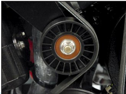
When adjusting or replacing a serpentine belt, spin the idler pulley by hand and replace if it makes any noise or has any play.
