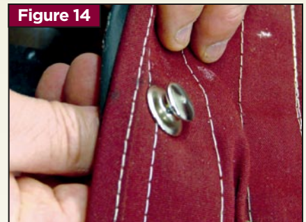
Pull-It-Up fasteners provide a secure deck attachment. Use four at critical points.
