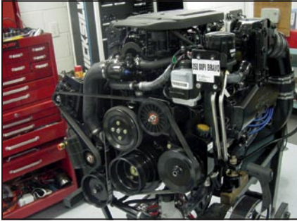
(top) 2008 model Mercury sterndrive uses a serpentine belt with a manual tensioner to drive engine accessories. (bottom) Manual serpentine belt tensioner requires only two wrenches to set belt tension.
