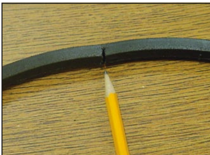
Inspect vee belts for wear and cracks every 100 hours or 120 days, whichever comes first. This belt requires replacing.
