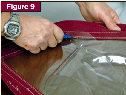
Use a seam ripper to cut away the old window.
