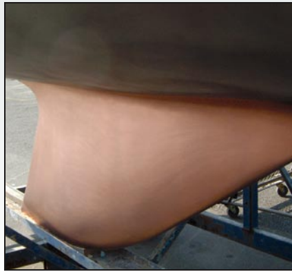
(left) A Beneteau 36.7 keel barrier coated at the factory, faired, epoxy primed, sanded and ready for the application of racing antifouling. (above) A C&C 27 keel ready for combat after many hours of prep.
