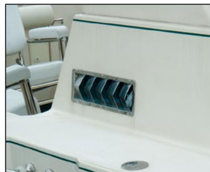
This sport fishing boat was given heavy spray and with the exhaust vent facing forward the ventilation hoses filled with salt after four years of use. Lack of engine space air flow caused the engines to smoke and lose performance.
