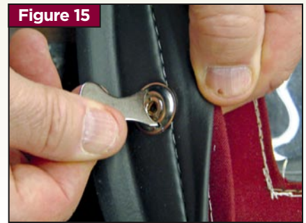
Pull-It-Up fasteners are screwed in place with a key.
