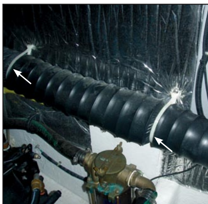
(left) Aged and torn hose. (right) Hose crushed by installation from the builder caused flow restriction in a fairly new vessel with ABYC-approval plate installed.
