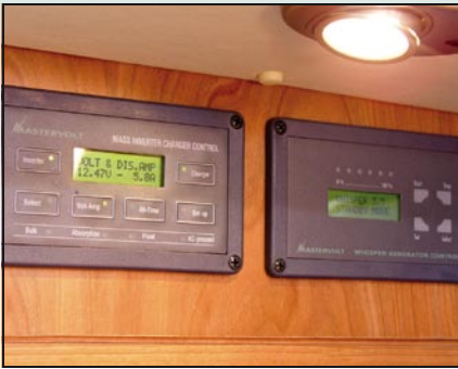
Mastervolt fully automated one-button operation generator controller module (right) mounts alongside the controller for the charger/inverter.
