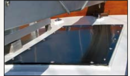
A Lexan panel is set into the hardtop covering the center cockpit.
