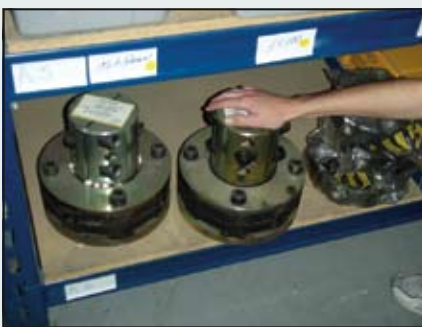
(left) Large Vetus Bullflex couplings. Note the split coupling on the shaft end to allow “clamping” the coupling on the shaft when installing. (right) Vetus Bullflex unit showing the heavy flexible “doughnut” between metal plates that attaches to the shaft and transmission.
