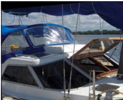
After: All new Plexiglas windows and a custom opening center section.
