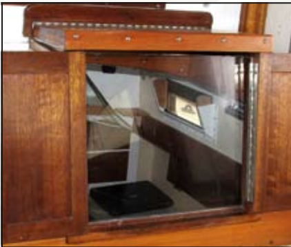
A window in the forward cabin door lets in light when the door must be closed.
