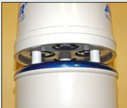
PB100's four ultrasonic transducers are visible through the four holes in the top of the sensor's wind channel.
