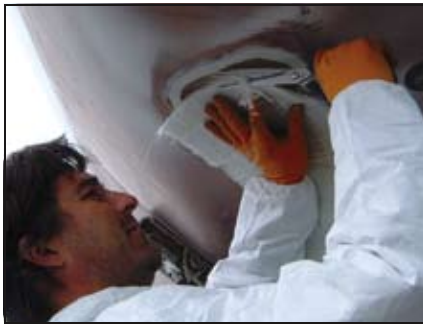
Cut out patches of fiberglass, 1810 stitch mat in this case, of approximately the same size and shape as the layers that were ground away.
