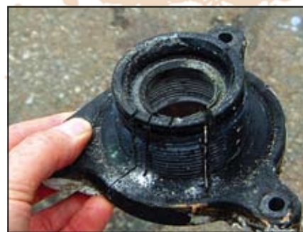
Remove the redundant thru-hull, in this case, a seacock thru-bolted in place.
