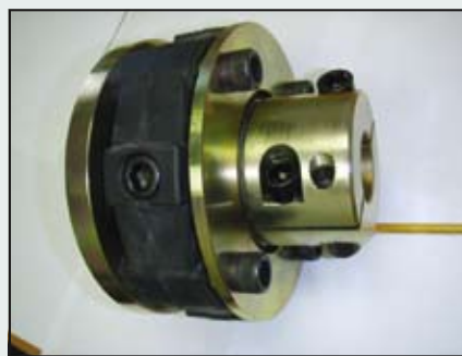
(left) Large Vetus Bullflex couplings. Note the split coupling on the shaft end to allow “clamping” the coupling on the shaft when installing. (right) Vetus Bullflex unit showing the heavy flexible “doughnut” between metal plates that attaches to the shaft and transmission.
