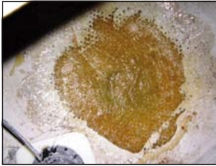
Any hole repair should be an (top) inside and (bottom) outside repair, although only a layer or two of glass suffices for the patch on the inside of the hull.
