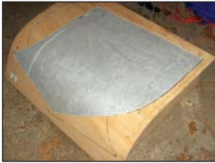
(top) Plywood and particle board mold construction. (bottom) Photo shows the outline of the port and starboard front wraparound windows.
