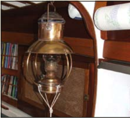
Hanging lanterns must be secured at the bottom to limit the swinging that could cause the glass to break or the lamp oil to leak.
