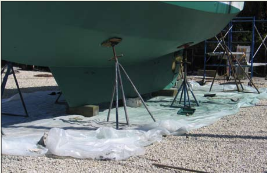
When refinishing bottoms, always lay a ground tarp to collect debris, runoff and paint spills.
