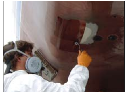
Bottom paint application is the final step. This may or may not include epoxy barrier coat primers prior to antifouling.
