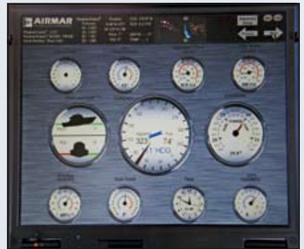
Third screen shows the weather information as well as pitch and roll. Through this display, I learned that my PB100 mount had a lean of 7 degrees toward the bow, now corrected.
