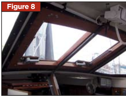
Figure 8 View of hatch from cabin interior. Support bar hides the radio wires.
