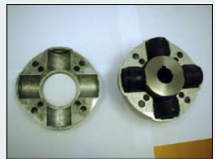
Vetus Type 6 coupling showing the bushings inside the unit. This coupling works with fixed or flexible stuffing boxes and a special conical clamping hub saves installation time.
