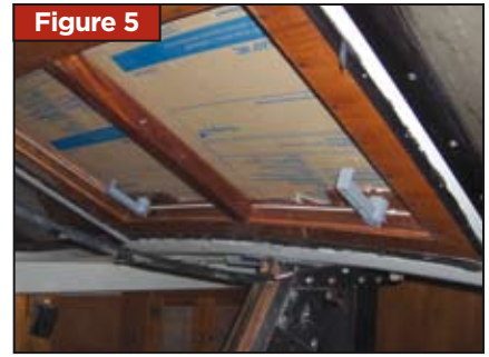
Hatch lip was extra wide to make a base for the Vetus hatch locking handles. Note wooden bungs that cover the screw heads.
