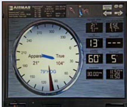
The second screen shows a mix of analog and digital information. Wind chill does not display unless air temperature is below 42F (5.5C)
