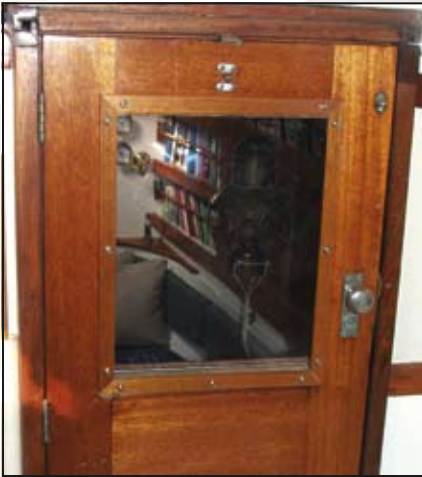
A window in the forward cabin door lets in light when the door must be closed.
