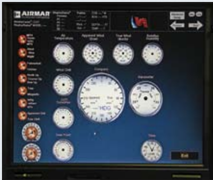
The main screen in blue background before setup. The orange icons on the left permit display customization including color, units of measure, time, direction, etc. There are three display screens and a choice of two background colors and night mode.
