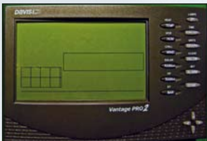
(top) The all-in-one Davis Vantage Pro 2 measures barometric pressure, humidity, rainfall, temperature, wind speed and direction using wireless stations. (bottom) The Vantage Pro Monitor (data not connected).
