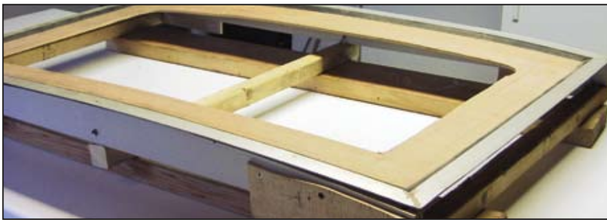
(top) Wood jig to hold window frame. Jig must be strong enough to hold the frame curvature, as plywood tends to flatten it when bent. (bottom) Plywood cut accurately on the outside dimension and secured into aluminum frame with rubber gasket. Interior cut was made with a router using a laminate trimming bit after hatch lip was laminated.
