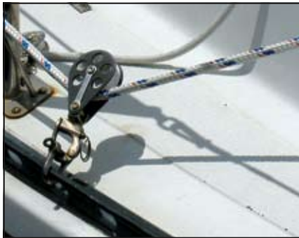
Single block attached to the toerail makes a acceptable and uncomplicated lead block for jib sheets.
