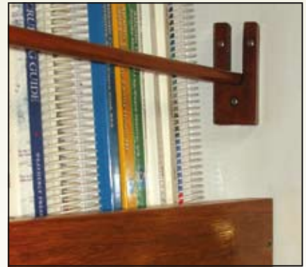
Open bookshelves need a fiddle rail and an added restraint about mid-height.
