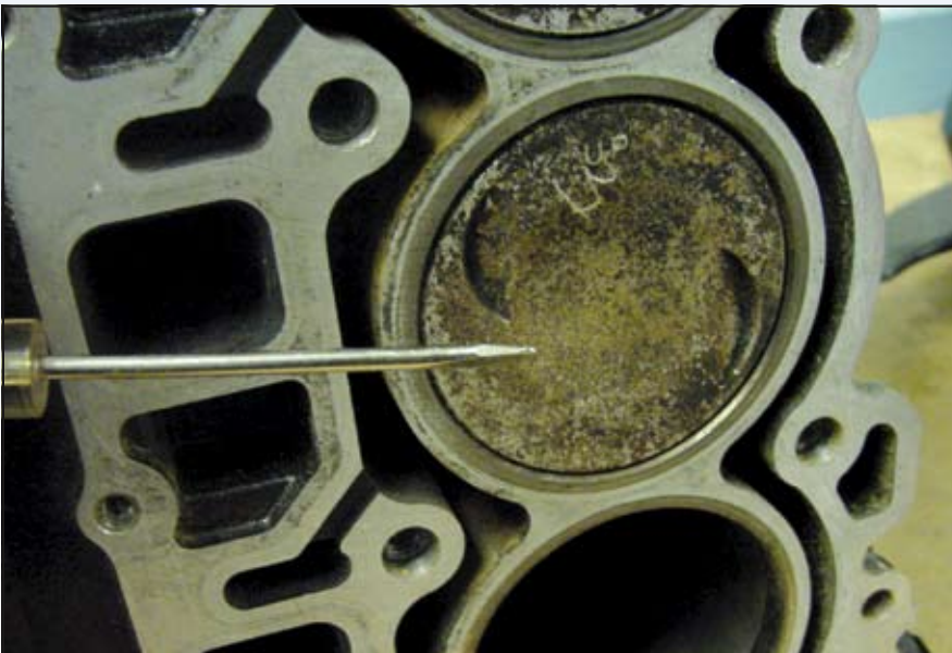
(top) Carbon deposits on a four-cycle engine piston. (bottom) Clean piston without carbon.
