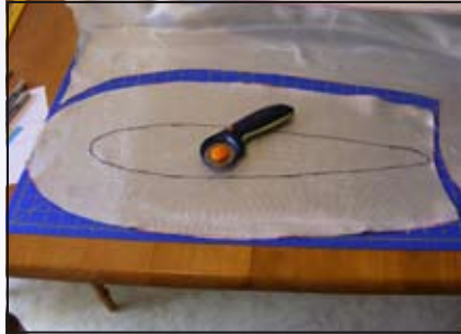
One of the three pieces of cloth needed for the bottom of the rudder. The outline helps center the cloth under the rudder.
