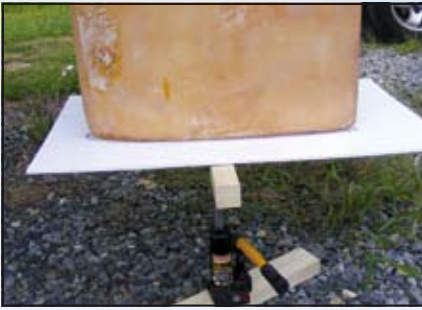
A small hydraulic jack supports the foam board in position for tracing. This also was the technique the author used to laminate the cloth on the rudder bottom.
