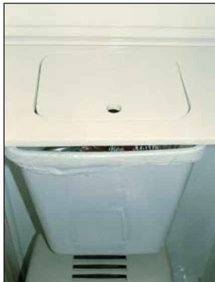
Recycle bin shown against bulkhead hangs on lashing hooks and rests on shelf/bracket.
