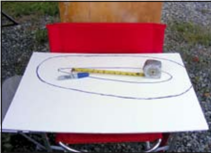
A line drawn 4" (101mm) out from the rudder outline formed the outside of the pattern.
