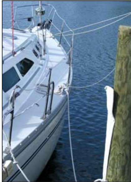
Midship cleats allow a better lead for spring lines. Note the twin cleats for bow lines.
