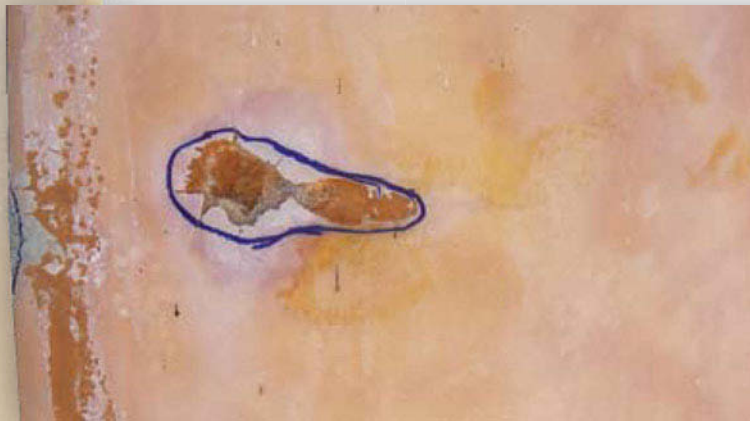
This was the gouge in the side of the rudder. Luckily the foam was dry.
