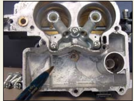
Modern fuel contains alcohol, which holds water that corrodes and affects carb performance.
