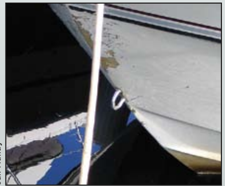
During a storm the stern line chafed through causing the bow of this powerboat to grind against the dock.
