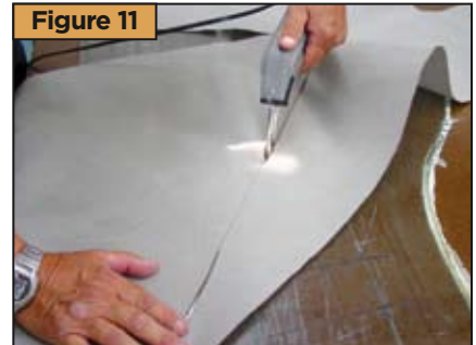
Cutting the Sunbrella shade with a hot knife to seal the edge.
