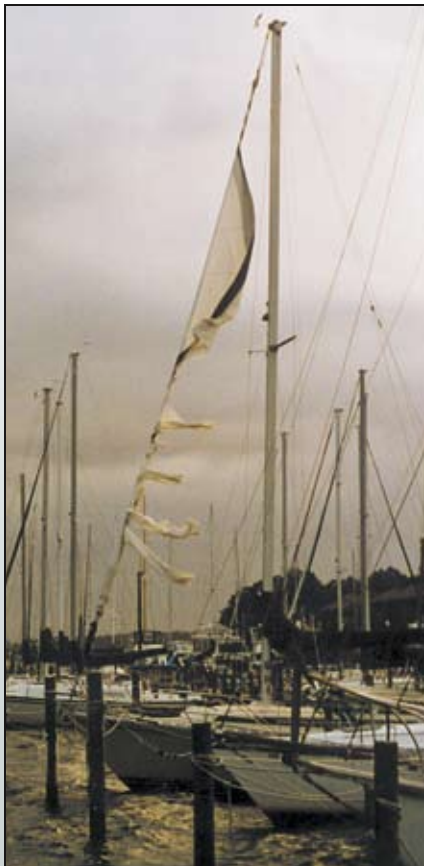
If your sailboat has roller furling, removing the sail is the only sure way to prevent winter storm damage to the sail.
