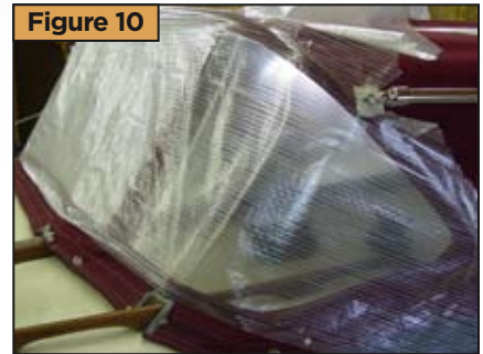
Making a pattern for the dodger window. Double-sided tape holds everything in place.
