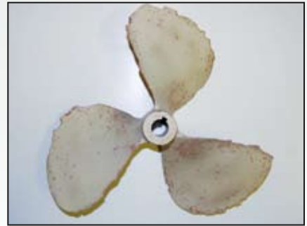
Examples of pitting from corrosion that have damaged these props beyond repair.
