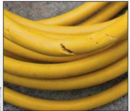
Twelve hours of storm activity caused the chafing on the dock that sliced through the outer jacket of this shorepower cord.
