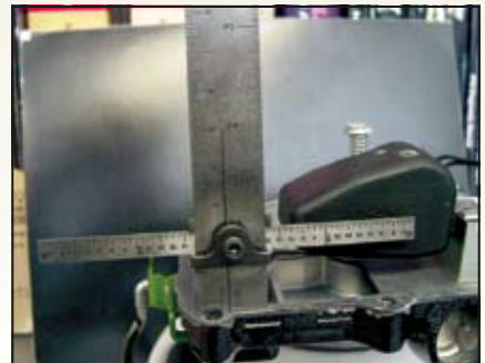
A specialized tool sets carburetor floats to the correct height to prevent flooding.
