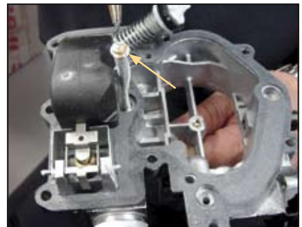
Debris on the power valve plunger can cause the valve to stick open.
