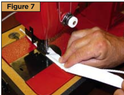
Locking the shock cord in the fold of the sleeve skirt.
