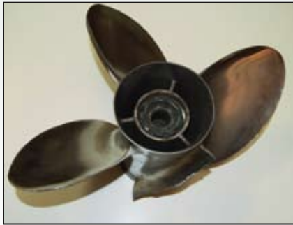
(top) Barely visible hairline crack. (bottom) If not fixed, a cracked blade will break off and the prop becomes scrap.
