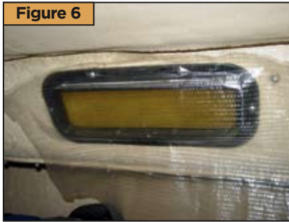
Canvex secured over the portlight with double sided tape ready for markup with a felt tip pen
