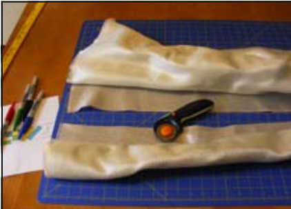
Here is the complete cloth cutting setup: rotary cutter, pad, markers, yardstick and cutting layout. A rotary fabric cutter and pad is the best way to cut fiberglass cloth. Note the crisp, unfrayed edges.
