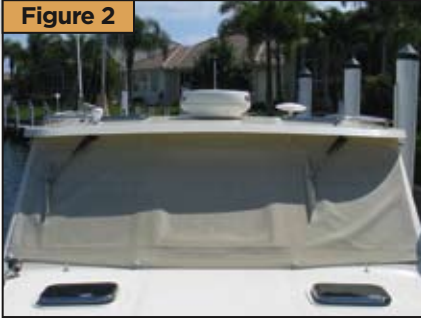
Phifertex Plus as an external cover with Permalock fasteners. Velcro closed sleeves cover the wiper blades.
