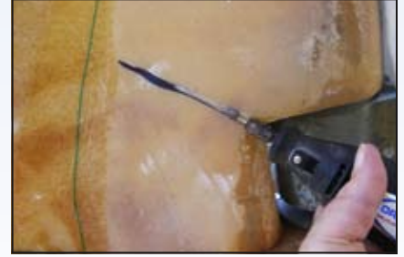
An acorn-shaped cutter in a Dremel tool widened the crack before filling with epoxy.
