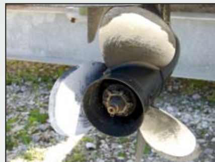
Repaired leading areas are highly visible on this aluminum prop.
