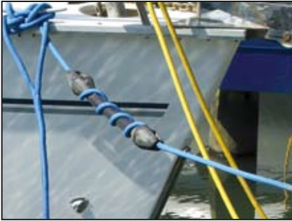
Line snubbers absorb the shock of a quick stop as the boat shifts with wind or current.
