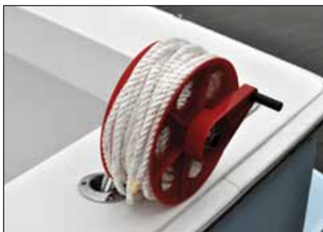
The Anchor Reel relies on a rod holder.
