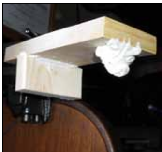
Even hanging upside down, the putty did not sag and held two boards together.
