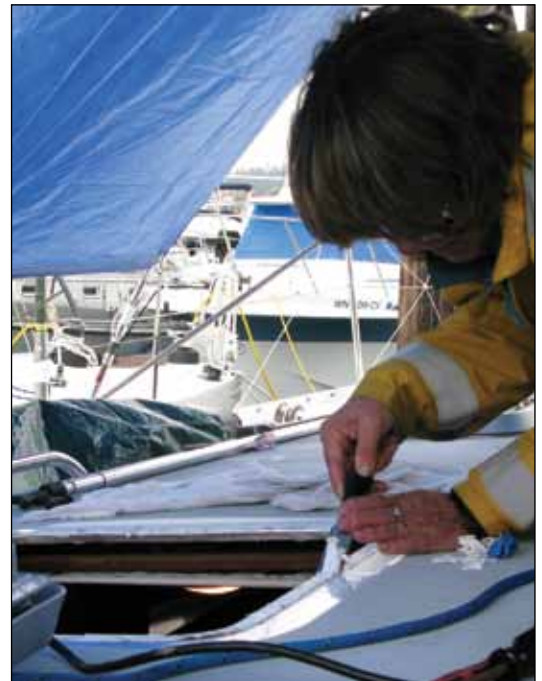
Counter-clockwise from left: Remove the bolts on the interior finish frame. Using painter's tape to protect the deck, carefully heat the old sealant and pry up the frame. You need a clean fit for the new hatches, pictured above.
