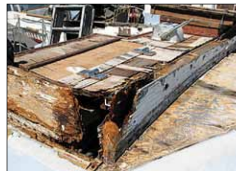
Randy Cunningham refurbished the World War II-era craft after finding one on Craigslist. Each area of the boat needed attention, including the rot on the pilothouse and surrounding area.
