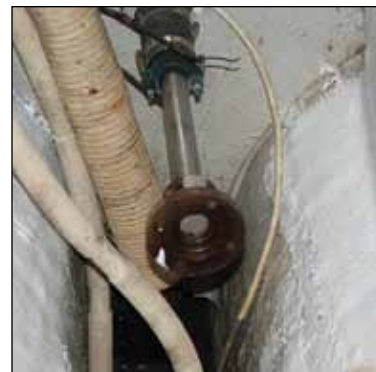
Top: When the engine was stripped, I prepared to hoist it out. Left: I used 4-by-4 verticals and a 4-by-6 oak crossbar to make a strong frame for the chain hoist. The chain had a clear path into the engine room. Above: The empty engine room gave me good access to the shaft coupling, so I could remove that last part of the old engine.
