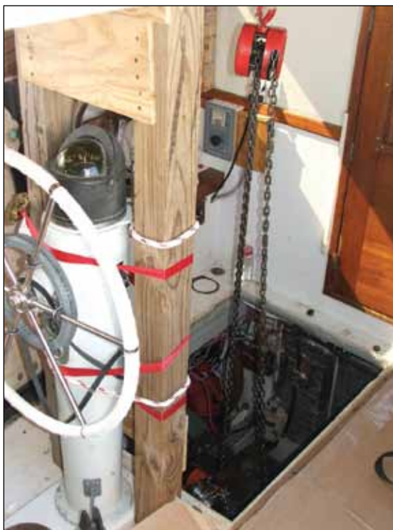
Top: When the engine was stripped, I prepared to hoist it out. Left: I used 4-by-4 verticals and a 4-by-6 oak crossbar to make a strong frame for the chain hoist. The chain had a clear path into the engine room. Above: The empty engine room gave me good access to the shaft coupling, so I could remove that last part of the old engine.
