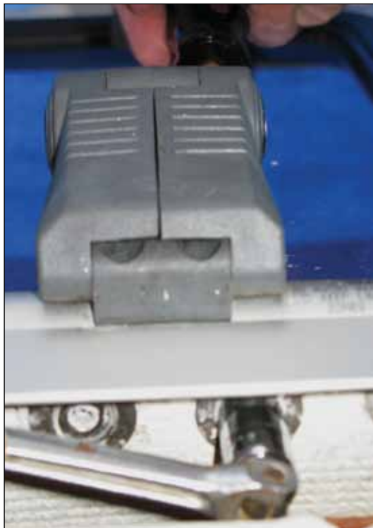
Counter-clockwise from left: Remove the bolts on the interior finish frame. Using painter's tape to protect the deck, carefully heat the old sealant and pry up the frame. You need a clean fit for the new hatches, pictured above.
