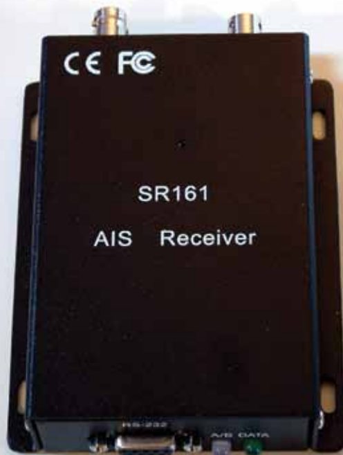
One of the more affordable AIS receive-only units is Milltech Marine's single-channel SR161.
