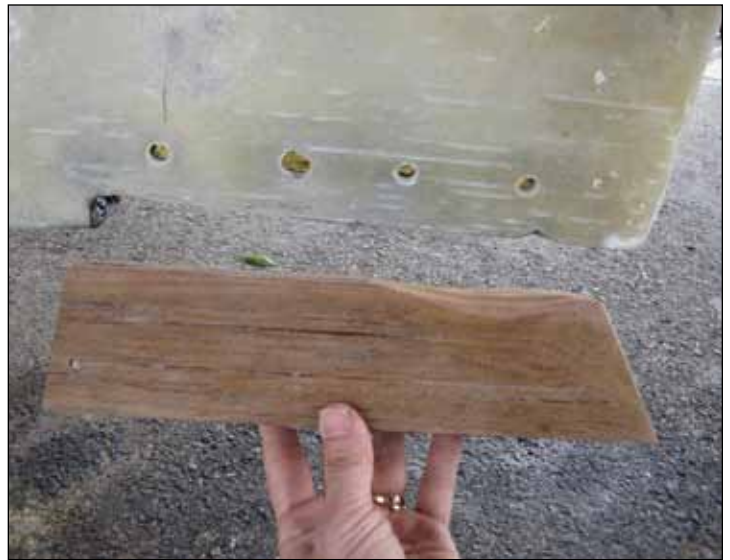
The void was filled with teak encapsulated in epoxy.
