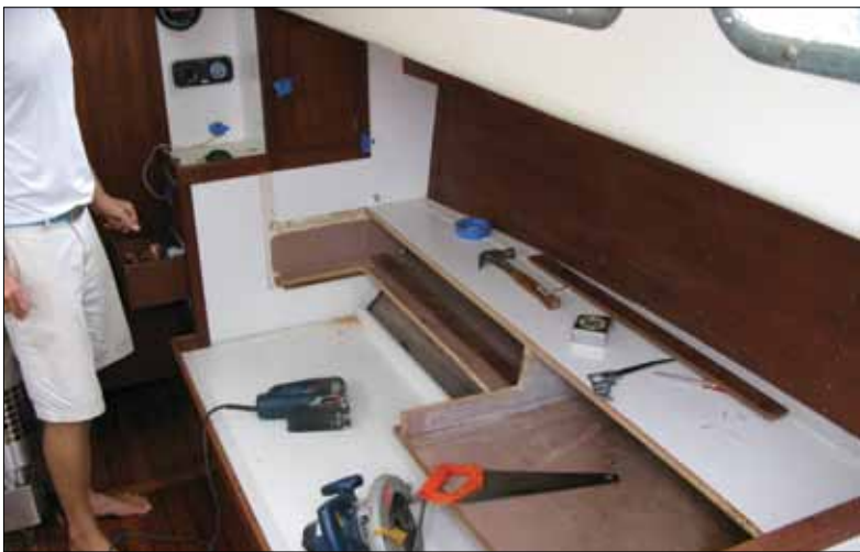
Halfway through demolition of the starboard side, the author cut back the pilot berth and added an angle for the new backrest, leaving intact the lockers that were originally built in.
