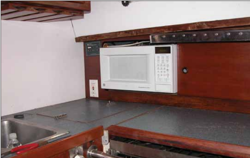
The microwave is mounted in space we borrowed from galley storage, a safe distance from the sink and stove.
