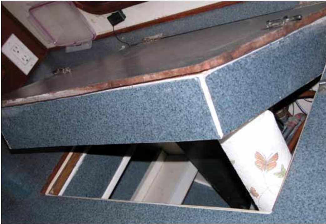
The new 5-inch-thick lid for the refrigerator is virtually all insulation. Wood trim around perimeter provides rigid sealing surface.
