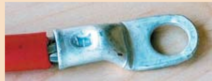
Little or no wire should be visible outside the lug.
