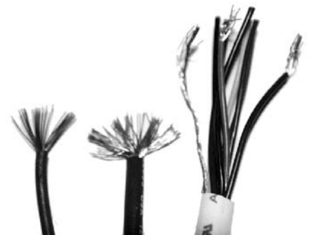
Figure 4: Never use SAE wire (left), an automotive copper wire that has few strands and is 12% smaller than marine grade. Multiple-stranded, tinned copper AWG wire (center) is more flexible and offers three times more corrosion resistance than SAE. To reduce magnetism when routing wires near compass or sensitive electronics, use a twisted pair cable (right) with a braided shield (Ancor Marine).
