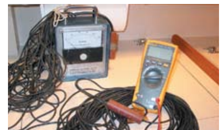
You can check the performance of your boat's bonding system using an analog corrosion test meter (left) or a good quality digital multimeter (right) and a silver/silver chloride (Na/NaCl) reference electrode. The corrosion meter above is the Capac unit sold by US Filter; Guest and Professional Mariner make less expensive models.
