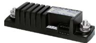
When voltage drops below the pre-set charging voltage, the BlueSea BatteryLink ACR opens to prevent accidental discharge of a battery bank.
