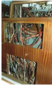
Terminal blocks from right to left: DC house circuits; starboard engine circuits; port engine circuits; tach circuits and remainder to be identified; and house busbar.
