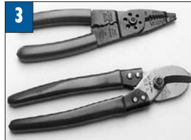
3 Cut/Strip/Crimp Tool (top); Wire and Cable Cutter (bottom).
