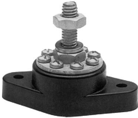
Figure 5: A negative consolidation terminal such as the PowerPost+, provides an attachment point for multiple negative cables, allowing a single cable to connect to the engine ground.
