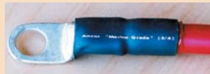
A heat gun produces the best results when shrinking tubing. Note how the adhesive is squeezed out forming a watertight seal.
