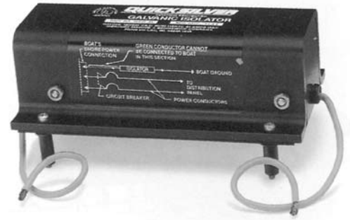
Quicksilver's galvanic isolator protects the hull, zinc anodes and aluminum drives (powerboats) from galvanic corrosion when your boat is plugged into shorepower.
