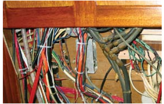
Terminal blocks from right to left: DC house circuits; starboard engine circuits; port engine circuits; tach circuits and remainder to be identified; and house busbar.
