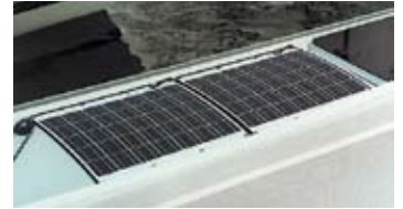
Figure 2 Rigid panel mounted on top of companionway hatch roof on raised aluminum brackets allow airflow underneath.
