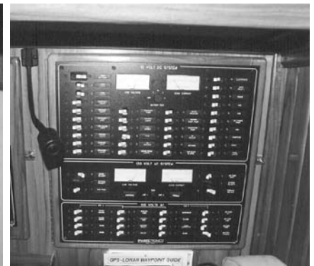
AC panels come in a variety of configurations, depending on your requirements: (right) panel with five-branch circuit capacity for basic installations; (left) Paneltronics' full-function distribution center with controls for shorepower, generator and inverter, current and voltage meters and 10-breaker capacity. Both panels are equipped with reverse polarity lights.
