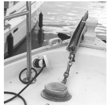
Shorepower inlet mounted in the bow of a Nonsuch 30 requires a watertight unit. Inlets are usually mounted in areas that are not normally subject to submersion, such as the cabin side or cockpit coaming.
