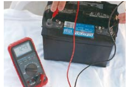
Use a voltmeter to test the start battery and replace if voltage drops below 9.5 volts under starting loads.
