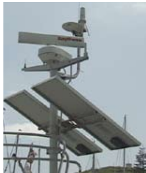
Figure 4 A rigid solar panel fastens to the boat's stern with rail mount clamps.
