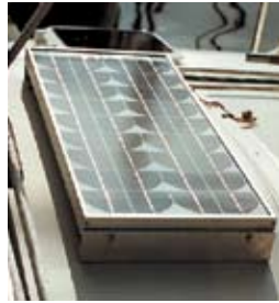
Figure 1 Semi-flexible panels mounted directly to a catamaran deck with corner fasteners.
