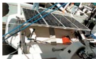
Figure 8 Two metal struts bolted to a stern or radar arch make a convenient place to fasten a solar panel.
