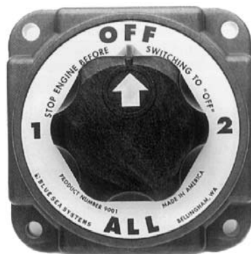
Figure 1: A four-position master switch lets you isolate the batteries, select which battery requires charging or completely cut off all power.
