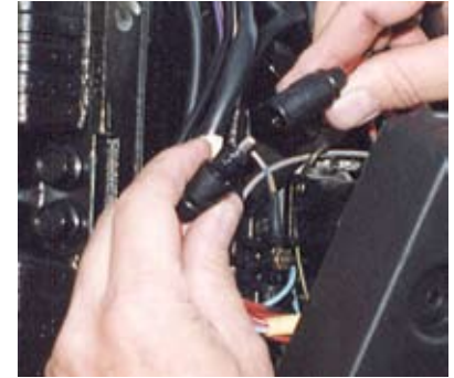
Loose or corroded main engine fuses, multi-pin plugs, socket assemblies and engine control wiring loom harnesses are the most common reason for engine electrical failure.
