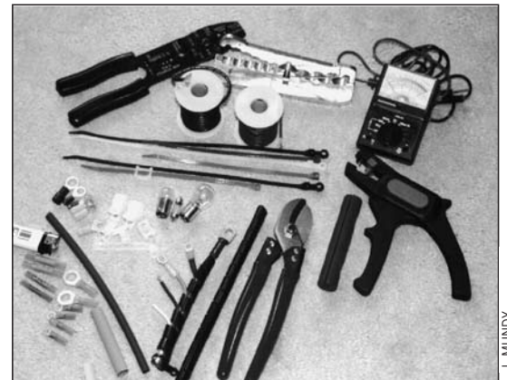
Figure 6: A typical DC electrical tool kit for DIY installations: crimp tool, lug crimper, multimeter, wire stripper, coaxial cable stripper, AWG wire, cable ties and clamps, fuses, assorted crimp and heat-shrink terminals, butane lighter or heat gun, heat-shrink tubing, spiral wrap, wire/cable cutter and wire markers (missing).
