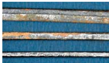
The top plate is from a heavy-duty deep-cycle battery used by railroads. The middle plate is from a popular deep-cycle battery used to power electric golf carts. The bottom plate is from a high-quality
