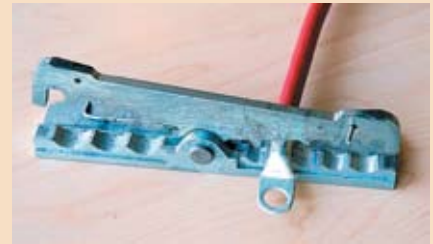
Position the crimp tool in the middle of the lug barrel.
