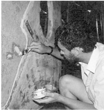
After pressure washing the hull with fresh water, blister cavities were filled with a mixture of microballoons, Cabosil and polyester resin.
