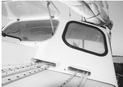
Halyard conduits were fashioned by wrapping fiberglass around an oval plywood form with rounded edges, then coating it with resin. Note the opening front window.
