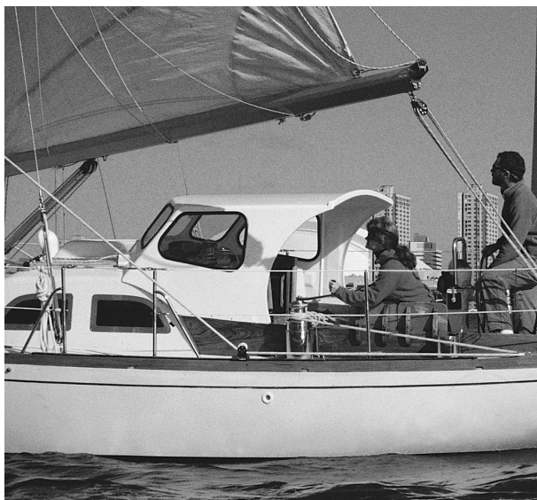
A hard dodger improves visibility, is watertight and the flat roof offers an ideal surface on which to mount solar panels.
