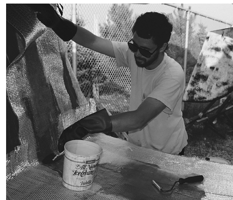
Fiberglass mat was first laid in the mold to create a smooth outer finish when cured.
