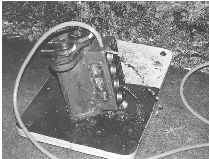
Flushing the block water jackets (this was done after the engine was apart).
