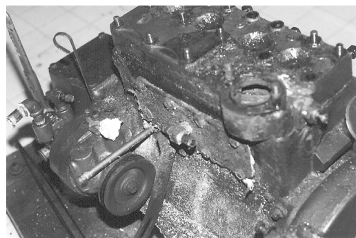
Corrosion and salt buildup on the engine.
