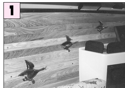
A wood ceiling adds warmth and ambiance to any cabin, but it's more expensive and demands some woodworking skills. To prevent condensation and keep the boat cool in summer and warm in winter, attach foam insulation to the hull between the ribs.
