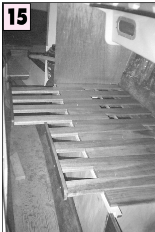
Double berth assembled with two-piece fiddle for easier handling.
