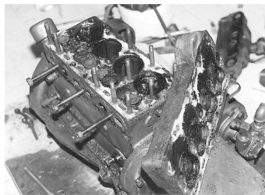
Head off, showing gaskets that need to be removed. Note carbon on pistons and valves.
