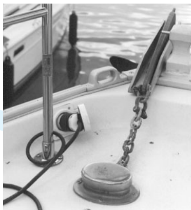
Shorepower inlet mounted in the bow of a Nonsuch 30 requires a watertight unit. Inlets are usually mounted in areas that are not normally subject to submersion, such as the cabin side or cockpit coaming.
