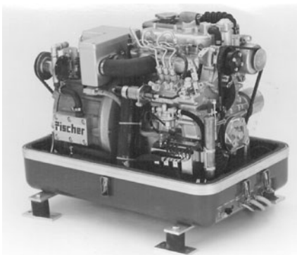
Fischer Panda water-cooled generators with three-piece insulated fiberglass sound shields are extremely quiet: the 7.8kW Panda 8 (shown) has a noise level rating of just 53 dBa.
