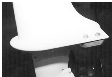
Anode mounted on Johnson 4-hp outboard.
