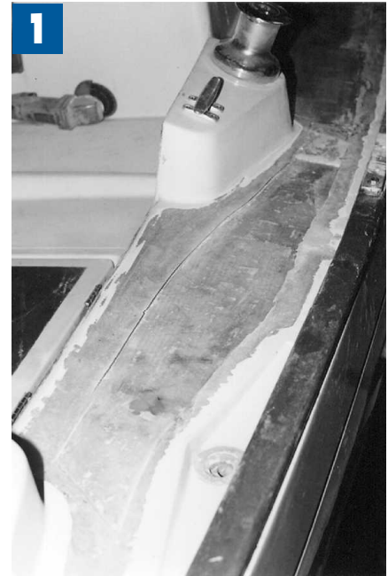
Side deck prepped for balsa core after coating the inner skin with polyester then epoxy resins. Note the beveled edges.
