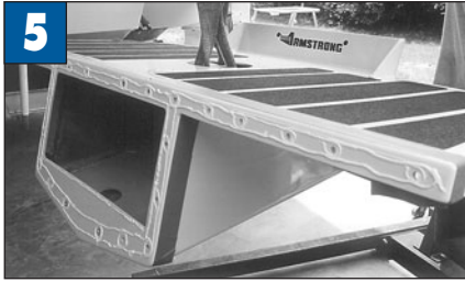
5 3M 5200 is applied liberally to the mounting face of the bracket and around all fastener holes.
