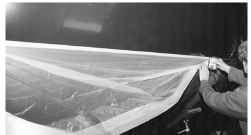
Ready-made drop cloth: 3M Marine's Ready-Mask pre-taped plastic film unfolds to cover surfaces when painting. Specially treated, this film clings to surfaces and is pre-taped with 3M masking tape or Long-Mask.
