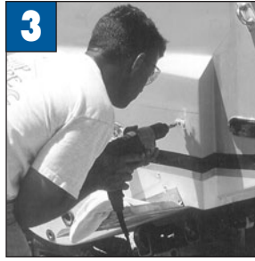
3 Drill pilot holes for bolts, then check for clearance.
