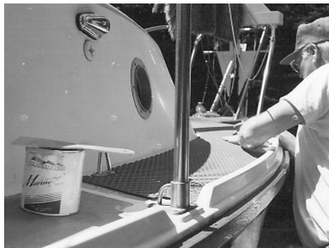
Lay the nonskid in place then apply moderate pressure to squeeze out air bubbles and excess glue.
