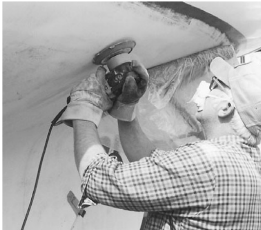
The author sanding with a random orbital sander and 80-grit paper to remove minute traces of bottom paint and smooth over blisters.
