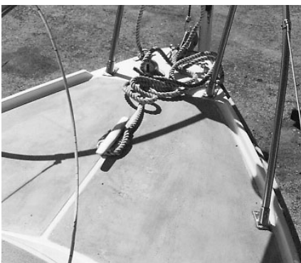
The old nonskid was showing the effects of 25 years of age and weather.
