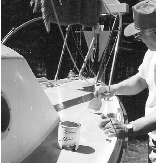
A specially formulated two-part epoxy is applied to the deck and the nonskid material.
