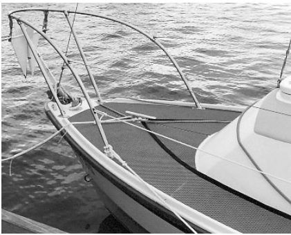
Teak-colored nonskid looks attractive, protects the fiberglass deck and provides better-than-new traction.
