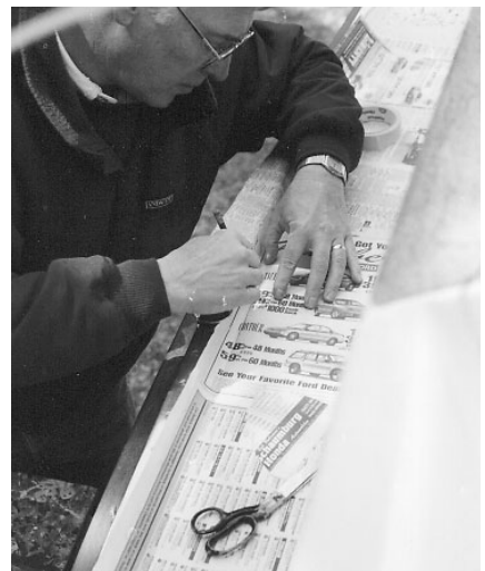
Making accurate patterns is exacting work and any misalignment will multiply once the fabric is glued in place.
