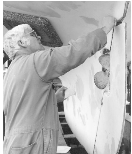
Applying Interlux Watertite fairing compound.
