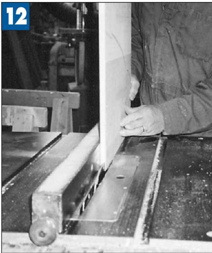
12 Removing the balsa core, which is replaced with a reinforcing spline
