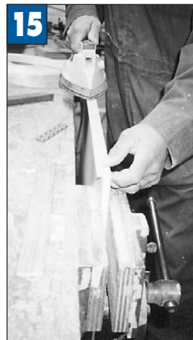
15 Iron-on veneer banding gets applied to all exposed edges.
