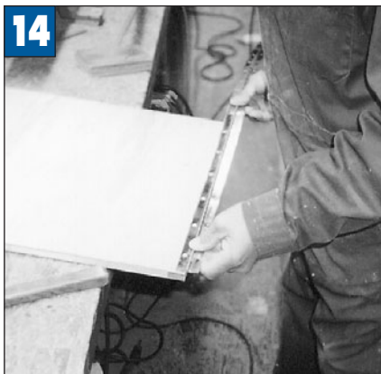
14 Piano hinge is fastened to the reinforced edges.
