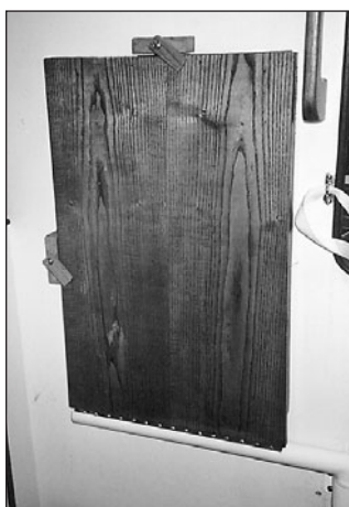
Lightweight table made of 12mm (1/2") DecoLite with fiber-reinforced wood veneer folds against bulkhead.
