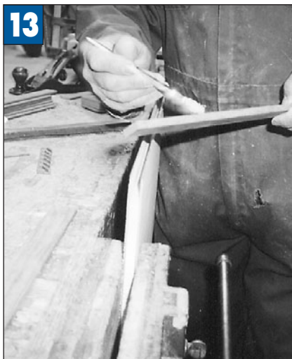
13 Mahogany spline is cut to fit the groove then set flush with slightly thickened epoxy resin.
