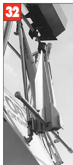
32 Stern anchor mounted within arm's reach when you need it most.
