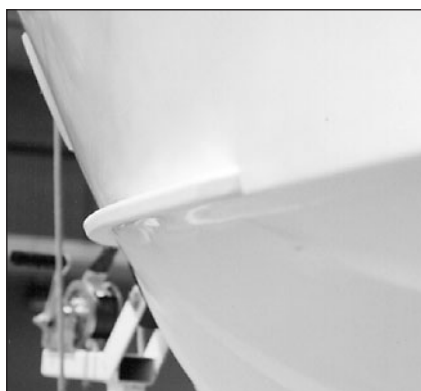
Spray deflector made of King StarBoard mounted at the chine prevents water from spraying upwards onto the deck.
