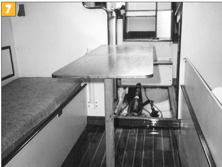
Lightweight table made of 12mm (1/2") DecoLite with fiber-reinforced wood veneer folds against bulkhead.
