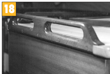
Cut handholds in rails mounted in the galley, chart table or anywhere an extra hand grab is needed. To make a handhold, drill 2.5cm (1") diameter holes, about 15cm (6") apart and up 2.8cm (1-1/8") from the lower edge, then cut out the stock and round the edges. Space cutouts at least 5cm (2") apart.
