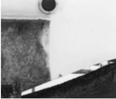
Transom of our test boat coated with bottom wax after two months in freshwater. The right side has been cleaned with Castrol Super Clean.
