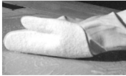
Use an abrasive pad-backed rubber glove to clean side decks, cockpit floor drains, behind stanchions or any area where brushes don't reach as well.
