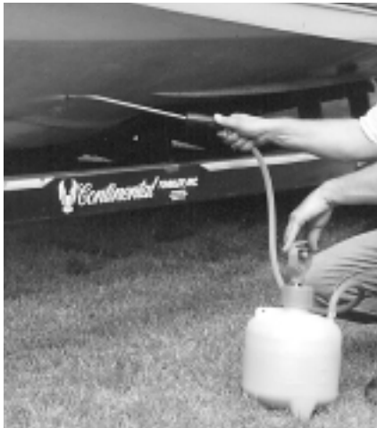
Pressure wash: a plastic garden sprayer with a spray wand does a great job of hull cleaning.
