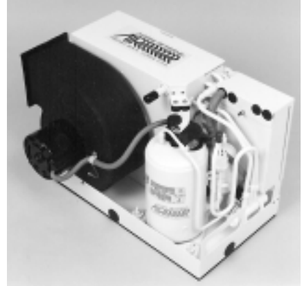
Measuring 30cm (11-3/4") high, 46cm (18") wide, 24cm (9-1/2") deep and weighing just 22kg (48lb), the 7,000 BTU Vector Compact by Marine Air is the most compact of the self-contained units.
