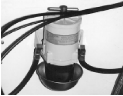
Racor primary diesel fuel-water separator with metal base to protect see-through glass bowl from breakage. For safety reasons, glass or plastic bowls are prohibited on gasoline-powered boats.
