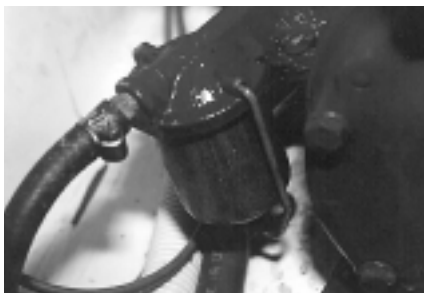
Fuel-water separator for gasoline inboard or stern drive engines has metal bowl that must be drained to determine if any water is present.
