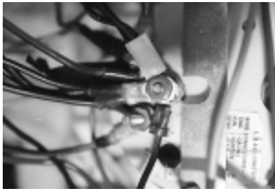
Original dealer installation shows eight negative wires crowding the "GND" post on the tachometer, leaving barely enough space to thread the nut.
