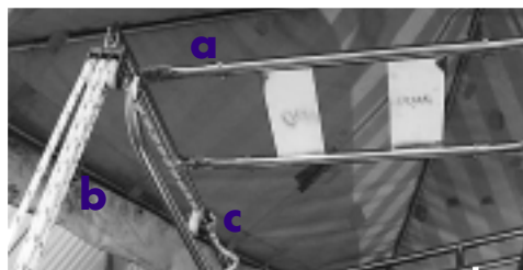
Typical options include (a) horizontal connecting struts, (b) block and tackle, (c) quick-release clam cleat to secure lifting line, (d) ratchet tie-down and (e) quick-removal mounting shoe.
