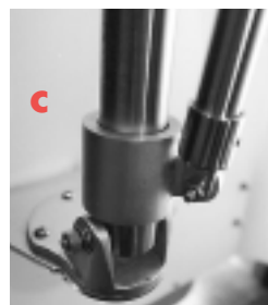
Examples of adjustable rail mounting brackets: (a) Ocean Marine UHMW plastic rail bushing; (b) Atkins & Hoyle cast rail mount with compression strut transfers loads downward onto base (c).
