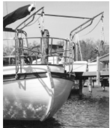
Ocean Marine's rail-mount davits with horizontal strut tie the two davit arms together to eliminate sway.
