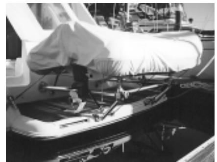
Atkins & Hoyle swim platform system utilizes a removable rotating davit to lift and rotate dinghy onto a cradle.
