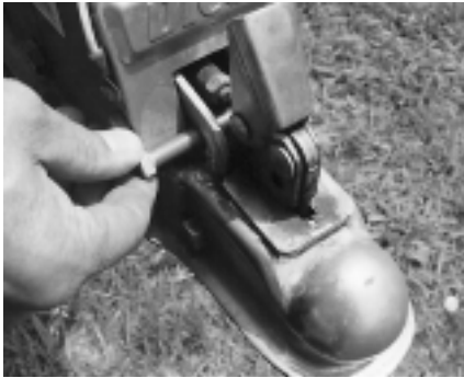
(top) Did you know you need to release this surge brake unit by inserting a 12mm (1/2") pin (left) when backing up?
