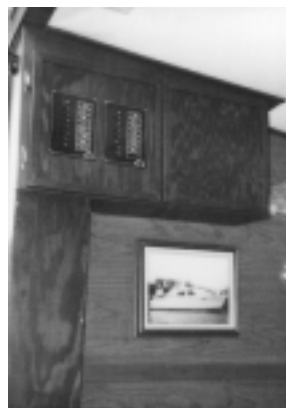
(right) Electrical cabinet and 12-volt breaker panels for house loads. (top) Wiring and dual battery switches inside cabinet.
