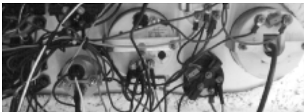
Inside view of outboard dash gauges and a cluttered wiring job. Non-factory supplied hourmeter, trim and water-pressure gauges completed the add-on package.
