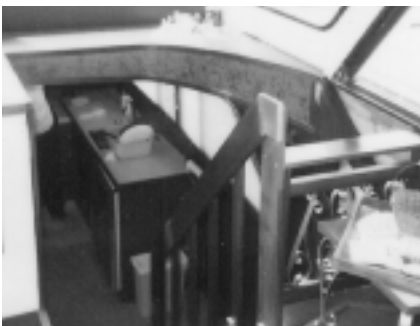
Dash and entranceway finished with Naugahyde and arborite, handrail and custom filler piece added.
