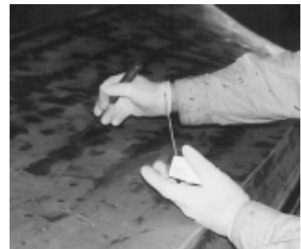
Filling all vent holes and staple dimples.
