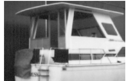
Vinyl-covered plywood closes in the space between the vertical support posts and the side.
