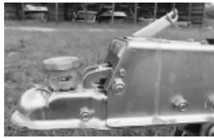
(top) Did you know you need to release this surge brake unit by inserting a 12mm (1/2") pin (left) when backing up?
