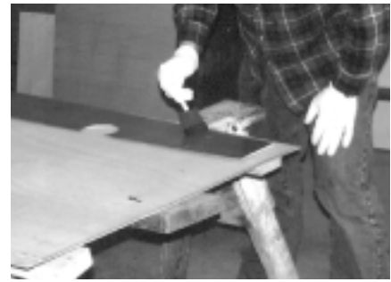
Plywood mating surfaces are coated with resin to prevent drawing resin from the thickened mixture and forming a resin-starved joint.
