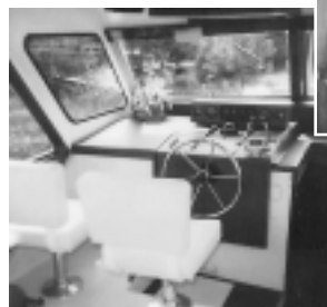
Renovated helm with compass, new controls, gauge box and breaker panels installed.
