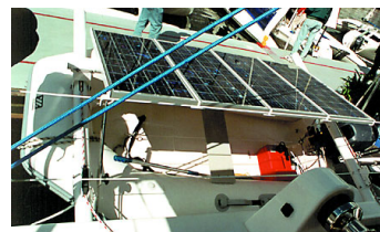
Figure 6 A pivoting stanchion-to-stanchion mount secures the solar panel on a rigid piece of metal tubing secured between stanchions with rail mount clamps.
