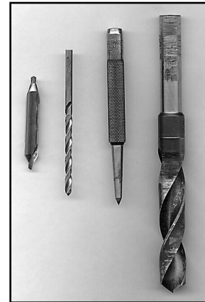
Tools for drilling stainless steel: center drill, a small pilot drill, center punch (actually a prick punch), reduced shank drill (9/16" to 1/2").
