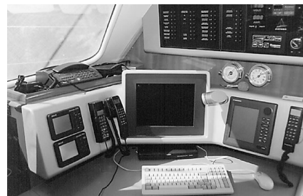
(above) Yeoman's "operations" board integrates GPS data with electronic plotting. (below) Command center onboard the Catana 472 multihull.
