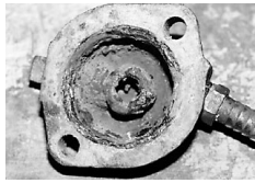
Before: Hard scale and rust deposits on the (left) block water jacket inspection plate, (above) cylinders and (bottom) thermostat housing.
