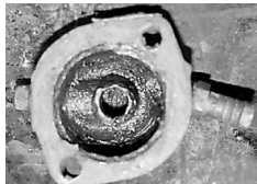
After: (left) Water jacket plate, (above) cylinders and (bottom) thermostat housing were cleaned of rust and scale after circulating a 1:1 MarSolve-water solution for 3 hours.
