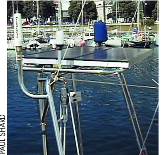
Panels securely mounted to tube supports that fasten to bracket on stern tower.
